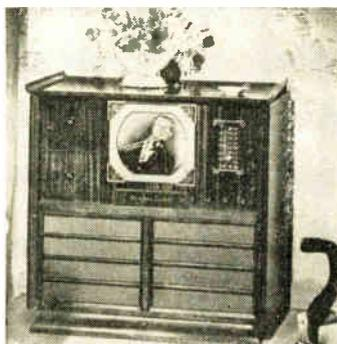
This model, the Chinese Classic, is in mahogany veneer with an Oriental motif, and combines AM-FM-television-phonograph. Has 92-square-inch picture screen. Standard broadcast and FM are built into television chassis. Has facilities for playing any type phonograph record, with two changers, one for standard or LP intermixed or for 7-inch LP in sequence. the other for 45-rpm records.
