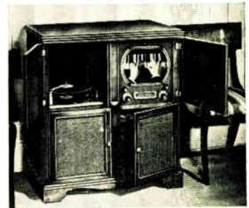
Screen on this television console combination is 63 square inches. Set uses a 10-inch picture tube, and features all-channel reception, built-in antenna and new discriminator circuit. AM-FM radio has 10-inch speaker. Record player handles all speeds and all sizes of records automatically.
