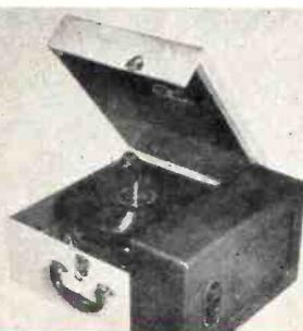
Waters Conley three-speed automatic record changer has three tubes, including amplifier, volume and tone controls, and high-fidelity amplifier.
