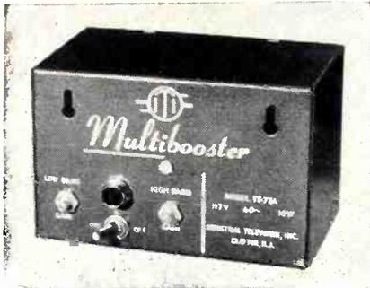
The Multibooster is a broad-band, television antenna amplifier for use with multiple installations. Features the same uniform response circuits of the Auto booster. Separate high- and low-band gain controls are provided. Use in conjunction with the Auto-booster is designed to combat receiver radiation problems.
