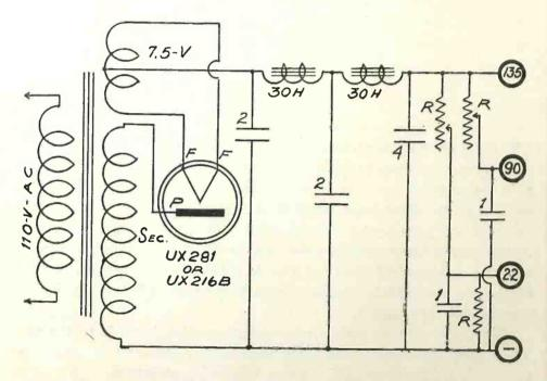
choke coils, two 2-mfd., one 4-mfd. and two 1-mfd. filter condensers are necessary. Also provide two variable high resistance units for voltage controls, a standard socket, binding posts and a 10,000-ohm fixed resistance.
