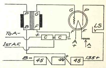
POWER tubes may be employed with any type of set. Their use results in greater volume and ideal tone quality. Slight charges are necessary in the receiving set. These are shown in the accompanying circuit. It is essential to employ higher B battery voltage and an additional C battery.
