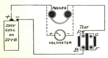
In TESTING a transformer primary, it is best to have it out of the set. Wire a battery in series with a pair of earphones as shown. To one side of the transformer make a permanent connection to the battery as shown. The test clip from the earphones should be brushed against the other transformer primary terminal. If a click is heard it indicates that the transformer winding is not open.
