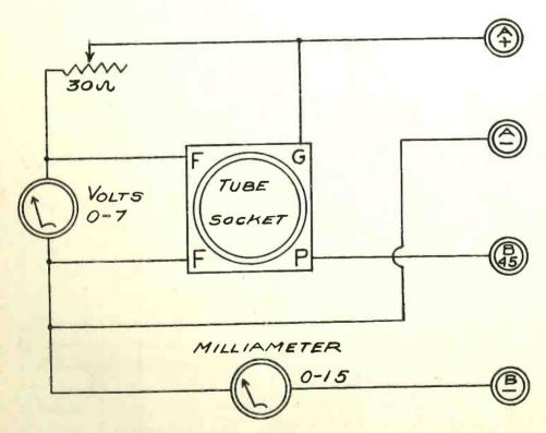
from 0 to 10 volts and a milliammeter reading from 0 to 15. Only the best of meters should be employed. Besides the meters the hook-up calls for a 30-ohm rheostat, a universal tube-socket, four binding posts, a sheet of bakelite about 7 by 9 inches. Bus-bar wire may be employed
