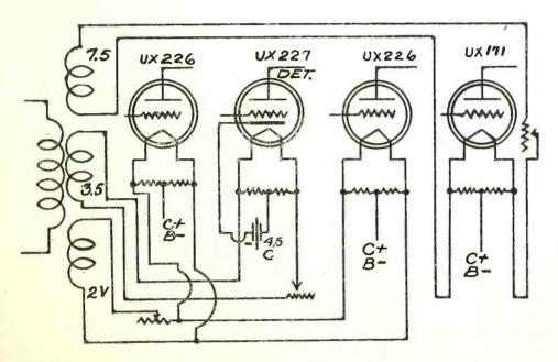
FOR SEVERAL years there has been a tendency on the part of manufacturers to build receiving sets to operate direct from the house lighting service. A number of such sets have already been put on the market and have been successful. Owners of receivers which require the use of a storage battery can now convert the filament wiring so as to accommodate the new UX-226 or CX-326 and UY-227 or C-327 alternating current Radiotrons.
