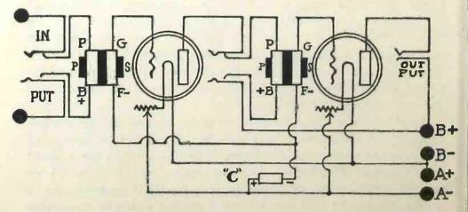
desirable in the first and second stage, and most manufacturers now mark transformers "first" and "second" stages to meet this requirement.
