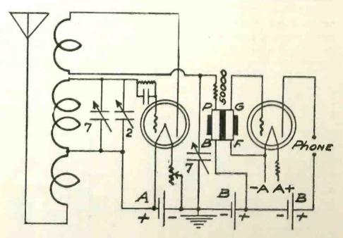
sary to connect two condensers in parallel as shown, the second condenser, consisting of but two plates, will enable the operator to follow up and control any signal better than if the condenser was not employed.
