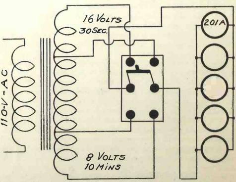
VACUUM tubes of the UX-201-A, CX-301-A, UX-199 and C-299 types which have lost their usefulness but still light and are not defective may be put through a process known as reactivating and
