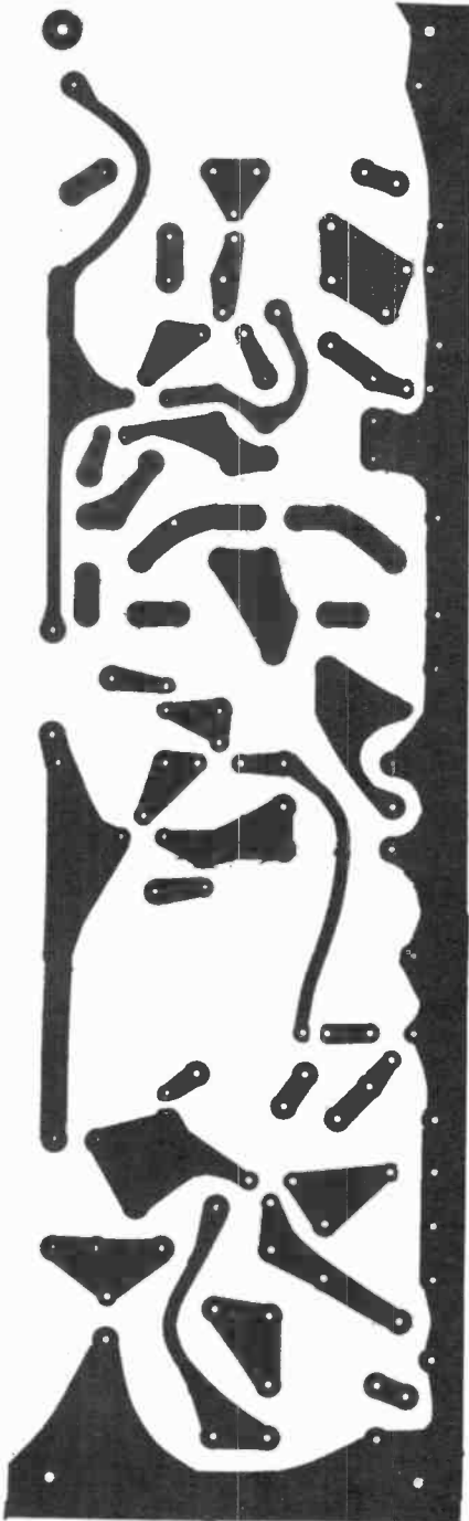
Fig. 6. Actual-size printed board for assembly of instrument preamplifier. The preamp can also be used independently with any instrument audio system.
