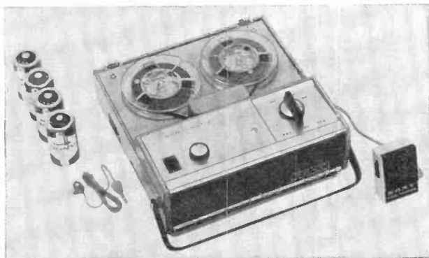
Sony "Sony-Matic 907" 3\frac{1}{4} -inch reel; 1 track; 2 speeds ( 3\frac{3}{4} and 1\frac{7}{8} in/s); operates on 4 "D" cells for 20 hours; has automatic record level circuit (a.v.c.), and can be remotely controlled; 8\frac{3}{4} " x 8\frac{3}{4} " x 5\frac{1}{2} "; 5\frac{1}{2} lb.
