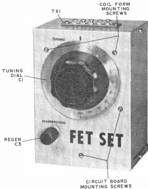
Fig. 2. Start construction by drilling holes in the aluminum box to accommodate the tuning dial shaft and regeneration control. Then drill mounting holes for the circuit board and coil form as shown here.
