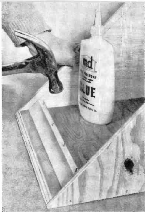
Fig. 3. Side cleats are miter cut at 45° angles; then glued and nailed to sides, 1/2" in from front.
