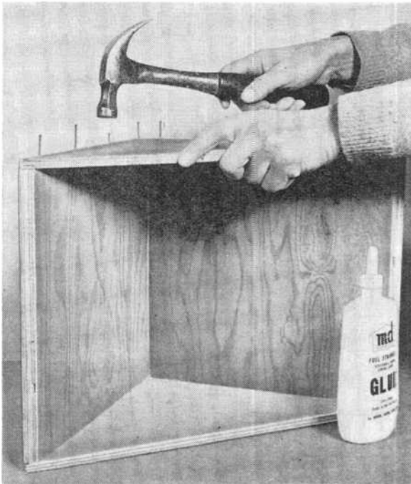
Fig. 2. Liberal bead of white glue between joined members helps to rigidize enclosure and provides air seal. Finishing nails anchor members together.
