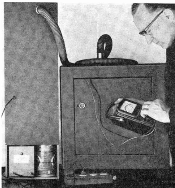
Fig. 9. The front door does not come down to the bottom of the cabinet to allow for air intake and observation of the indicator lamp. To prevent operation when the door is open, a TV "cheater" system is door operated.
