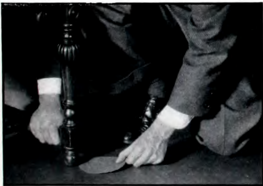
Felt pads under a set will often aid in minimizing unpleasant noises
