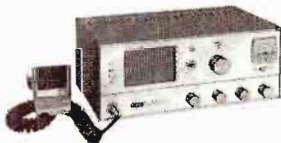
New Model 712 Sentinel 12 Dual Conversion 5-watt CB Transceiver. Permits 12-channel crystal-controlled transmit and receive, plus 23-channel tunable receive. Incorporates adjustable squelch & noise limiter, & switches for 3.5 watt P.A. use, spotting, & Part 15 operation. Transistorized 12VDC & 117VAC dual power supply. $99.95 wired only.
