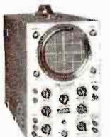
Model 460 Wideband Direct Coupled 5" Oscilloscope. DC-4.5mc for color and B&W TV service and lab use. Push-pull DC vertical amp. bal. or unbal. input. Automatic sync limiter and amp. $89.95 kit, $129.50 wired.
