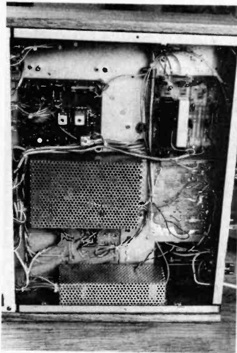
With the cover removed, the upper chassis is visible. Note the slot for the accessory filters, and the heavy RF shielding.
