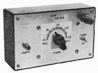
Whether you order the Super Booster kit from the Electronic Workshop or build the preselector from your spare parts collection, you'll still have to buy a suitable cabinet to house it in. The prototype's cabinet is Allied/Radio Shack's part number 270 B 627. A bakelite cabinet with aluminum faceplate is the easiest to work with.
