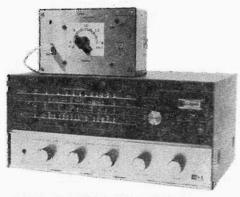
Super Booster helps this Realistic DX-120 to run after flea power BCB DX, by acting either as an "electronic antenna" or as a preamplifier.
