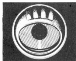
Fig. 3. Above is shown a tuning eye indicator or "Magic Eye" which facilitates in the proper tuning of not only domestic broadcasting stations but short-wave stations as well.
