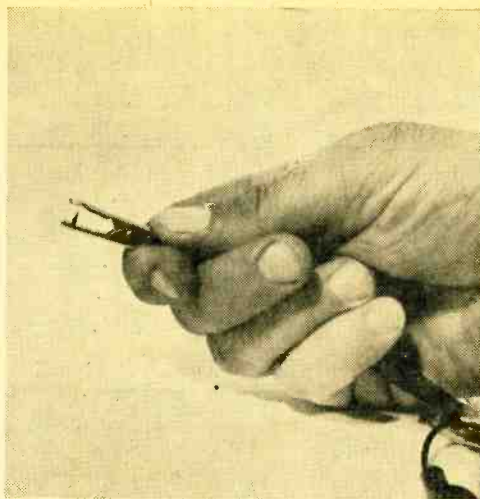
Attached gun killer cables have insulation-piercing alligator clips that stab through insulation, making contact but not injuring wires to CRT color grids.
