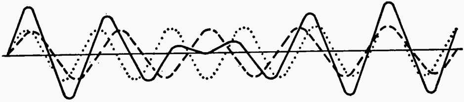
Fig. 10. Artist's representation of how beat is formed. Phase of two tones is basic here, since notes will tend to either reinforce or cancel one another.
