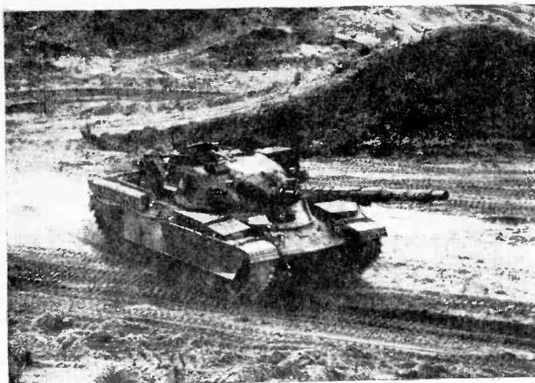
Fitted with laser simulator on top of gun barrel, British-made Chieftain tank rumbles into battle on training exercise. Tank's engine, radio, and gun go dead when hit with electronic shells; smoke automatically pours from tank when hit would have left it totally disabled.
