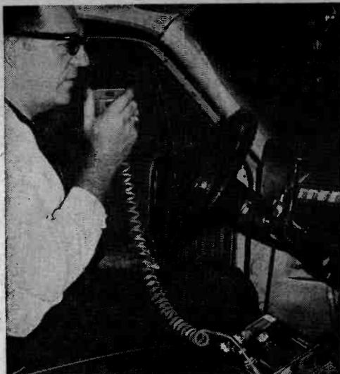
Mobile unit (above) calls Operation Spook Patrol's console operator (below) Tom Overall, KOM4664. Console is equipped with two FM (152-174 MHz) receivers to monitor police.
