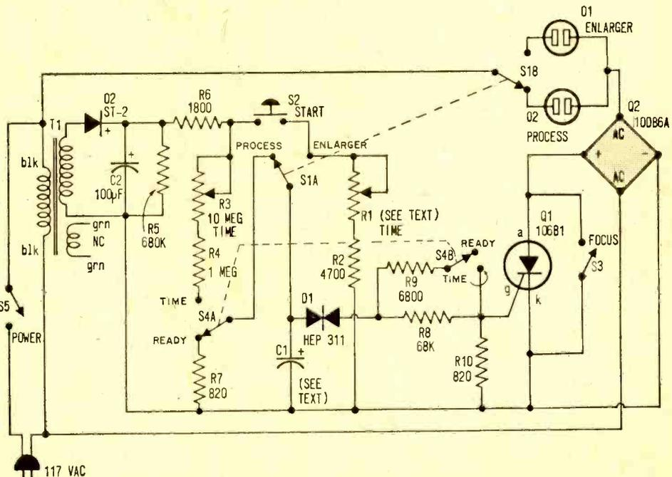
on (and the bridge conducts) whenever a current of more than 200 microamps (1/5 of a milliamp) is fed into the *gate* terminal.
