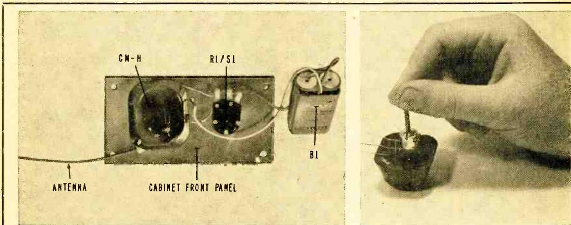
Practically any mounting arrangement will work for Police Converter, but it's best to keep leads from R1 to module as short as possible. Module (at right) is roughly size of ice cube.
