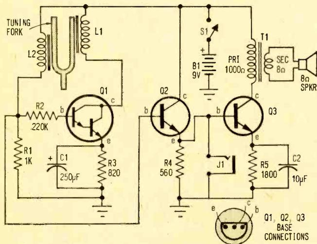
Schematic reveals Freq Standard's simple but highly accurate circuit. Mechanical tuning fork controls Q1's frequency of oscillation; audio tone appearing at Q1's base is then amplified and fed to either J1 (for further amplification) or direct to Freq Standard's speaker.
