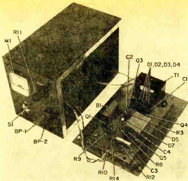
Here's what's inside our regulated supply. Note accessibility of components on circuit board. Because power transformer is relatively heavy, it needs extra support to prevent board from cracking.
