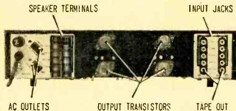
Output transistors are recessed in heat sinks, which are themselves recessed to provide flat, non-protruding rear apron. Both main and remote speaker terminals (at left) have their own common (ground) connections.
