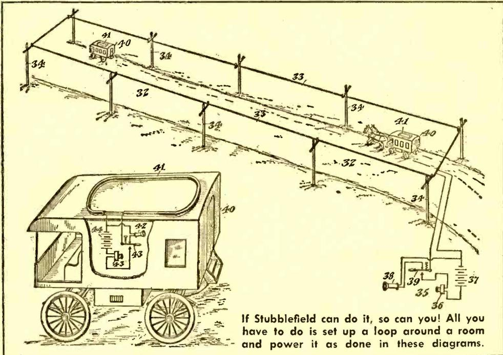
If Stubblefield can do it, so can you! All you have to do is set up a loop around a room and power it as done in these diagrams.
