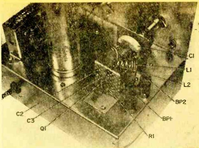
dial calibration. Another cause for variation in the original calibrations could be a change in transistor Q1.
