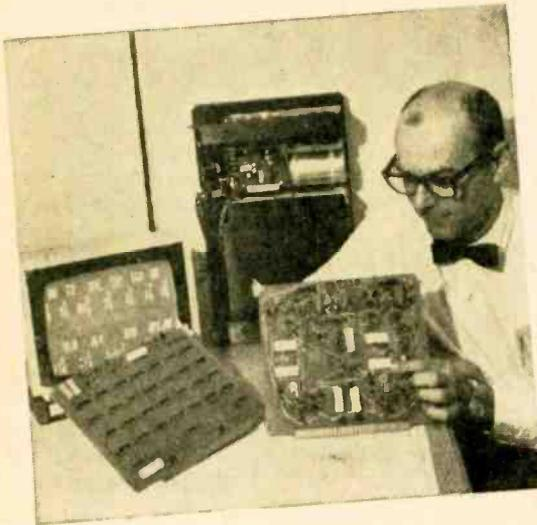
... new ICs help put market transactions on brokers' desks? Developed by Trans-Lux Corporation, the new Vidi-Quote records current stock-exchange information in binary code, then converts it to alpha-numeric characters which are displayed on a compact TV monitor. Its ICs are by Texas Instruments.
