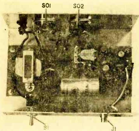
Completed PC assembly fits easily in base of 3 x 5 x 7-in. aluminum cabinet. Use at least #18 wire to connect up SO1 and SO2.
