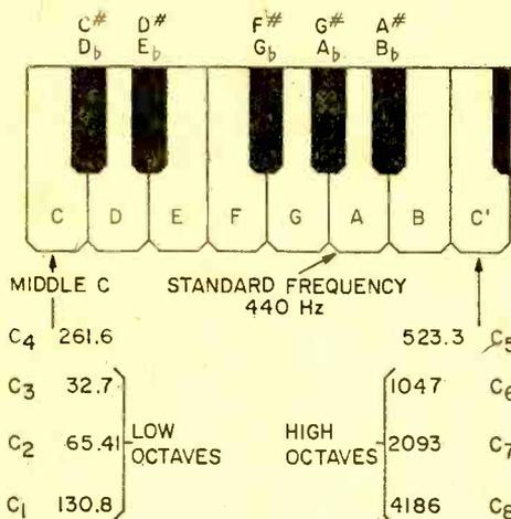
Fig. 4. Equal temperament scale now in common use allows no difference between sharps and flats (D<sup>#</sup> and E<sup>b</sup> are thus identical).
