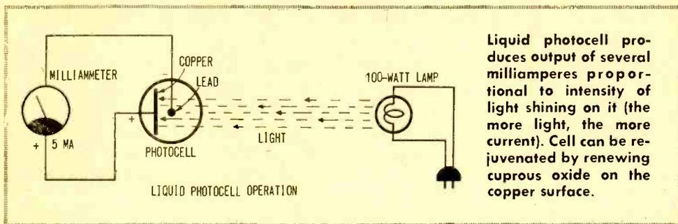
the form of visible light, strikes a suitably prepared metallic substance, electrons are emitted. In the absence of light, the copper and lead electrodes of this photocell have a small potential difference, as does an electrochemical battery with no load applied.
