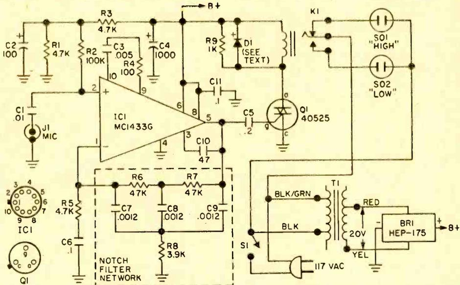
SO2 are chassis-type AC receptacles; one provides for the high-intensity lamp, one for the low. In the model shown a microphone connects to J1 so that the mike can be positioned some distance from the control unit. However, the mike can be placed directly in the cabinet by eliminating J1 and cementing a mike element to the front panel.
