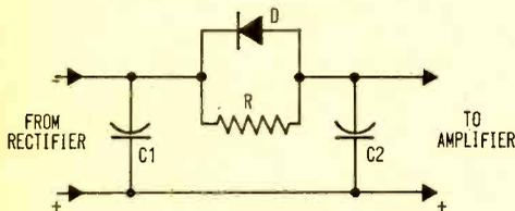
You might try adding additional power supply filtering by adding capacitor C2, diode D and resistor R, as shown in the diagram. Capacitor C1 is the existing output filter capacitor. When there is no audio signal going through the amplifier, power supply current is low, the diode does not conduct, and filter section R/C2 reduces power supply ripple. When power supply current rises, the diode conducts, shorting R, and allowing heavy current to flow
