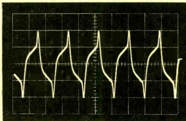
Fig. 4. Output of guitar amplifier with maximum fuzz, R1 set to 0 resistance. Note high degree of distortion.
