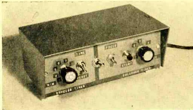
Finished product is very professional looking timing device that is of inestimable value in any darkroom, be it for professional or amateur photographers. It combines facilities to time development of film and/or paper as well as exposure timing for the enlarger. Incorporating silicon controlled rectifier and sophisticated timing approach, unit provides two different timing ranges economically by sharing common components.
