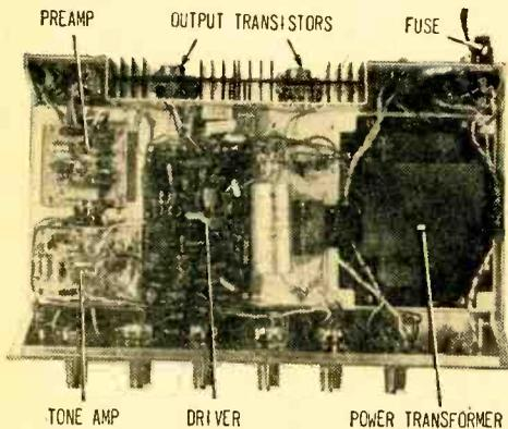
Each side of chassis contains printed circuit modules for single amplifier channel (this is upper side of completed amplifier). Top-side also contains power-supply filter, shown to left of husky power transformer. Even chassis is assembled in modular form: front (with controls), back, and amplifier base.
