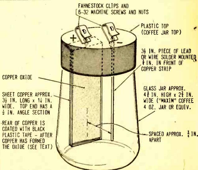
is not critical, but the jar must be made of clear glass and should have a plastic lid, or you will have to make a wooden or plastic lid to fit. The copper sheet may be difficult to obtain. We cut and flattened a length of 1/2-in. copper tubing for our model.
