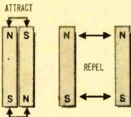
Fig. 3. Vanes can attract one another only when polarities differ. Here, polarities are always same, so vanes repel.
