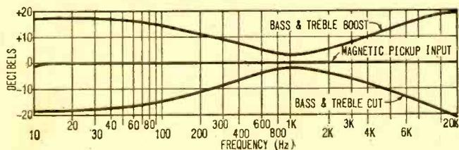
RIAA equalization on 3150 was ruder flat from 20 to 20,000 Hz. Bass and treble controls had fulcrum around 1-kHz point, with maximum boost and cut of some 20 dB.
