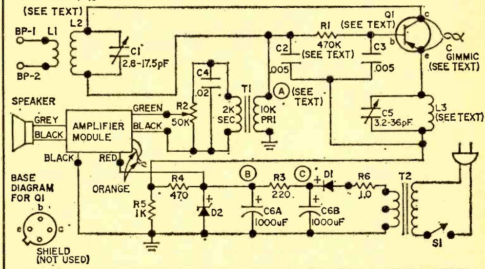
L3 is then self-supporting when mounted directly to C5. Use a rubber grommet to protect the leads from L3-C5 as they pass through the chassis from bottom to top.
