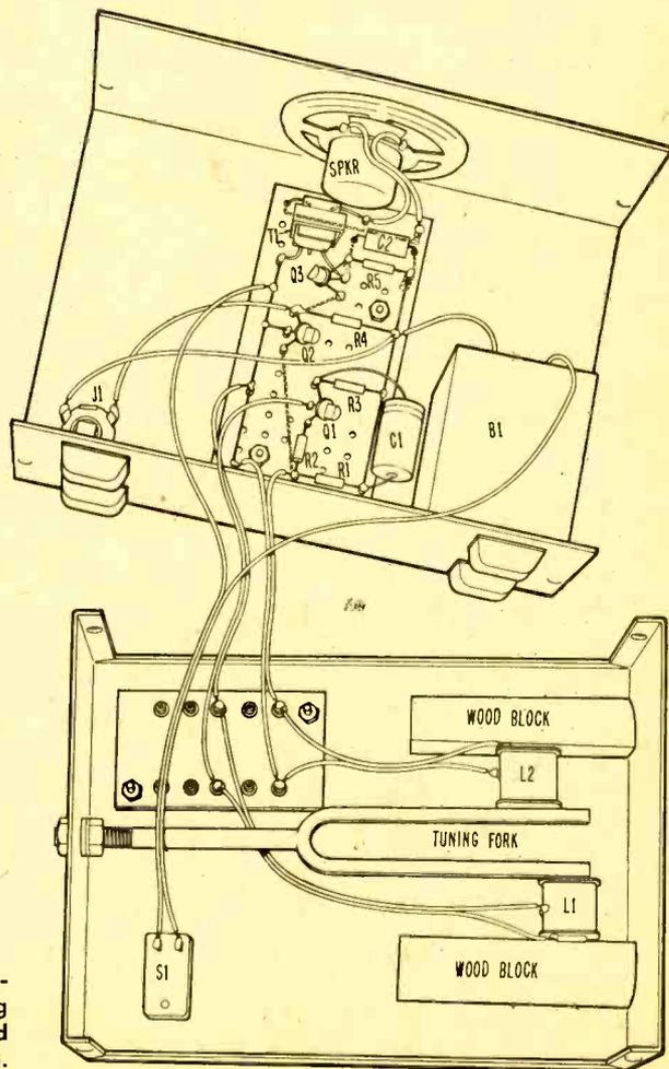
Freq Standard's mechanical construction is simplified by placing tuning fork in bottom of minibox, perfboard and most related components in top.
