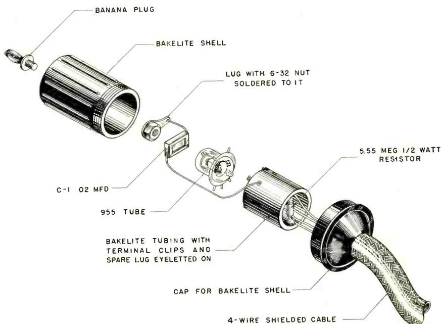
Fig. 4. Exploded view of probe showing construction for use with 955 tube.
