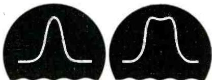
Fig. 7. Response traces for different degrees of selectivity; sharp (left), and broad (right).
