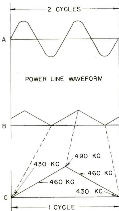
Fig. 1. Pyramid wave, B, developed from power-line sine wave, A; and output frequency variation, C, over one cycle of line voltage.
