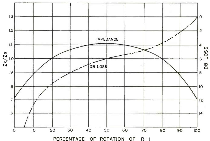
Fig. 2 The impedance ratio,  $Z_x/Z_s$ , is shown by the solid line and the loss in db is indicated by the dotted line, for various settings of the potentiometer.
