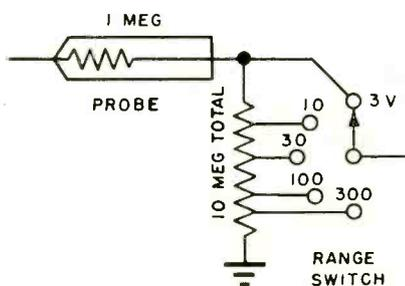
Fig. 1. Simplified input circuit of RCA Volt-Ohmyst.
