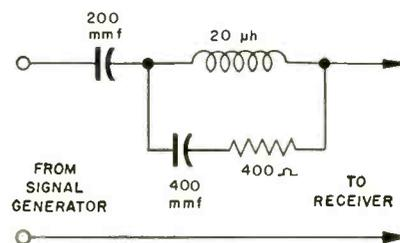
Fig. 8. Circuit of standard dummy antenna.
