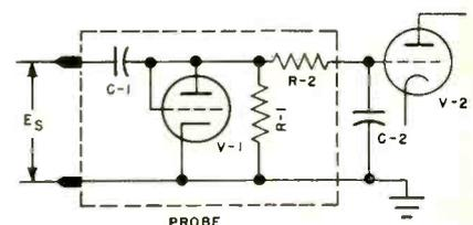
Fig. 2. Simplified input circuit of General Radio 726A vacuum tube voltmeter.
