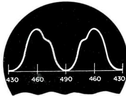
Fig. 2. Appearance of output of improperly adjusted I-F amplifier with oscillograph sweep synchronized at the power-line frequency.
