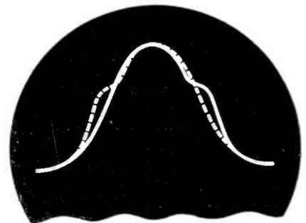
Fig. 3. Same I-F response as in Fig. 2, but with oscillograph sweep synchronized to twice the power-line frequency. The solid line indicates the response for the upswept half-cycle; the dotted line for the down-swept half-cycle.
