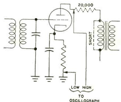
Fig. 6. Connections of oscillograph to biased detector, showing addition of resistor in plate circuit, and short across coupling transformer.
