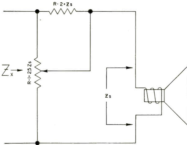
Fig. 1 Method of connecting simple wire-wound potentiometer and additional resistor to make a pad which approaches constant-impedance characteristic.
