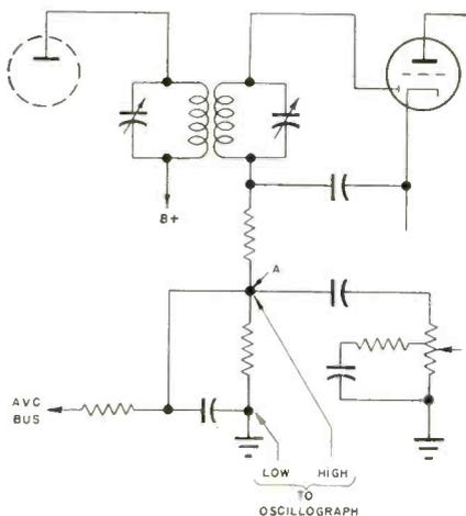
Fig. 5. Method of connecting oscillograph leads to receiver using diode as second detector.
