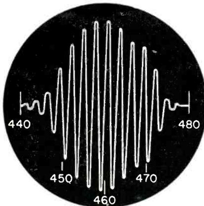
Fig. 4. Waveform appearing across secondary of I-F transformer with frequency-swept signal.
