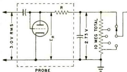
Fig. 3. Simplified input circuit for modified RCA Volt-Ohmyst.
