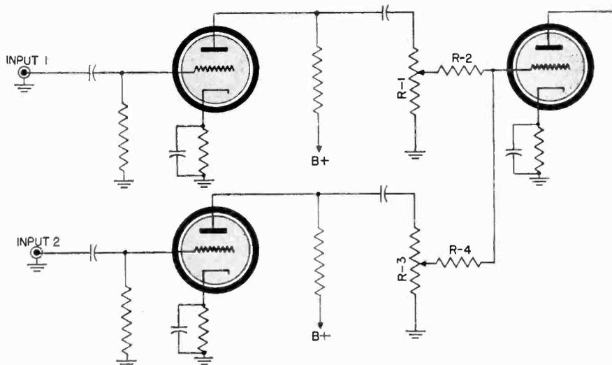
Fig. 11 One method of mixing inputs from two microphones. This method is in common use, and is quite satisfactory.
