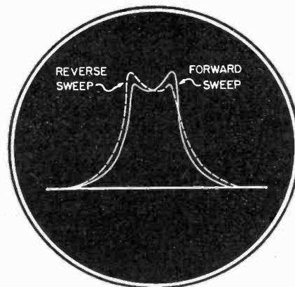
Fig. 8. Pattern obtained from a properly aligned discriminator using the method described in the text.
