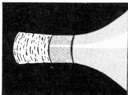
Fig. 2 Cork is placed in voice coil as shown.
