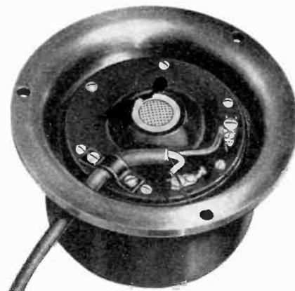
Fig. 10 A diaphragm type reproducing unit—the Jensen Hypex is equipped with a unit of this type.
