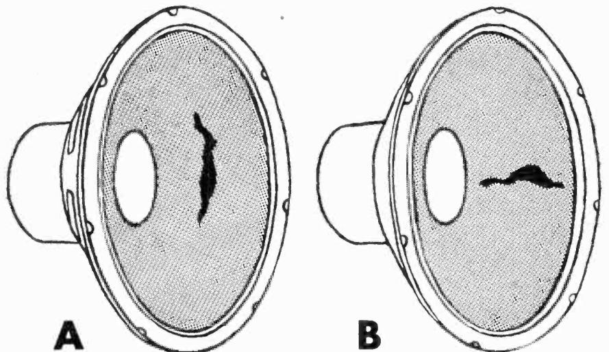
The tear A can be repaired while the one on speaker B cannot.
