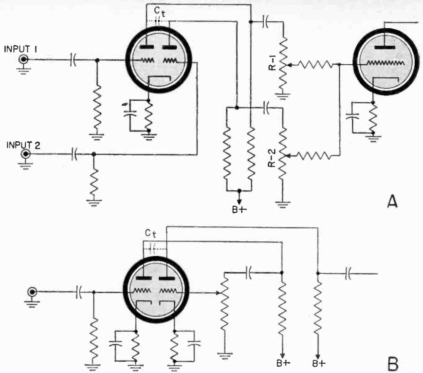
Fig. 14 Capacity  $C_t$  between tube elements results in crosstalk between channels. These circuits are not satisfactory.
