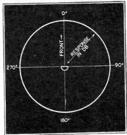
Fig. 1 Directivity pattern of pressure-actuated microphone. Curve shows unit to be equally sensitive in all directions.
