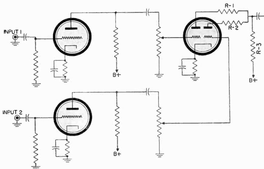
Fig. 13 Third type of mixing circuit, also satisfactory.
