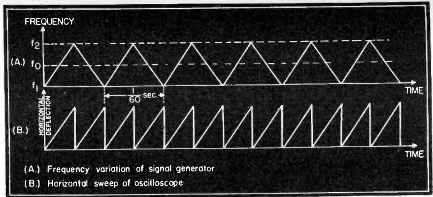
Fig. 7 The frequency variation of the signal generator and its relation to the horizontal sweep of the oscilloscope.
