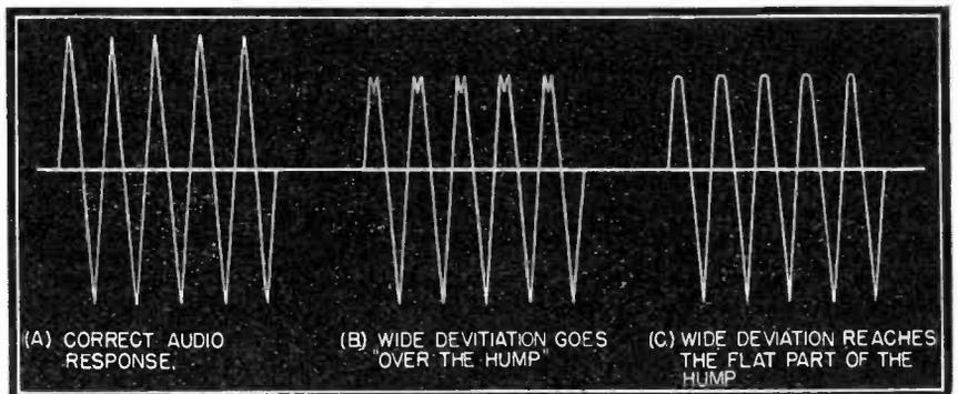
Fig. 3 The effect on the output of a discriminator of a too widely deviated signal.
