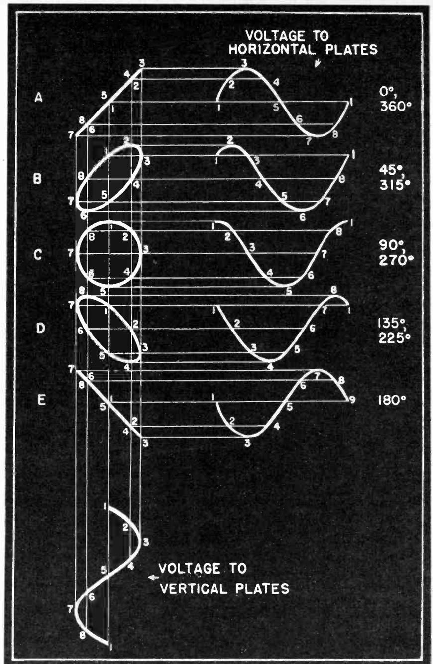
Fig. 6 Various types of patterns obtained with different phase relationships between the vertical and horizontal voltages applied to the cathode-ray tube.
