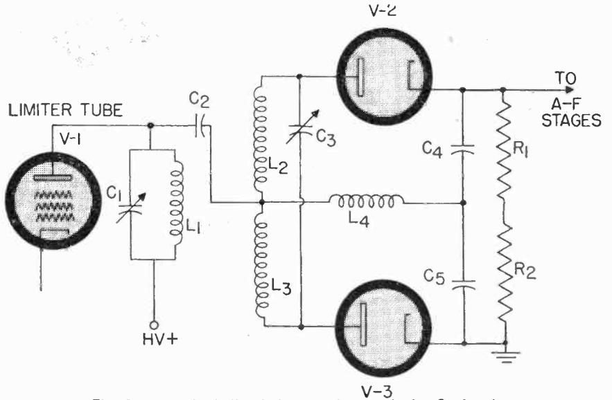
Fig. 1 A typical discriminator circuit, Foster-Seeley type.
