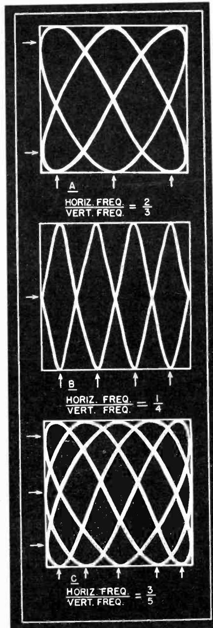
Fig. 8 A is the pattern for a 2:30 frequency ratio between the horizontal and vertical voltages; B with a 1:4 ratio; and C with a 3:5 ratio.
