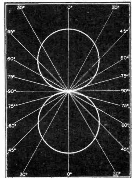
Fig. 2 Curve for "velocity" microphones shows them to be bi-directional.
