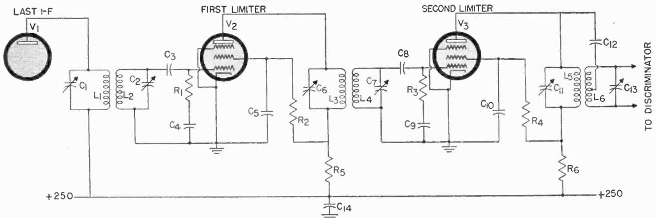
Fig. 6 A two-tube or double limiter circuit.
