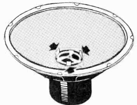
Fig. 1 Placement of shims used when realigning the voice coil of a speaker.
