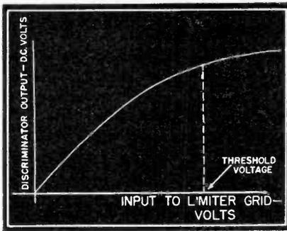
Fig. 4 Output response curve of a limiter stage — threshold voltage is usually on the order of 50 microvolts or less.
