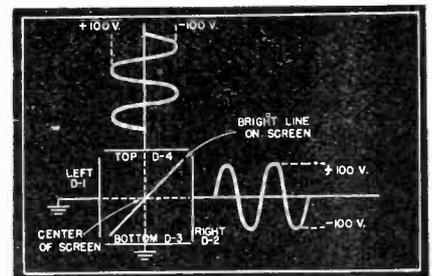
Fig. 5 When two sine wave voltages which are in phase are applied to the vertical and horizontal plates of a cathode-ray tube, the beam forms a straight line on the screen as shown.
