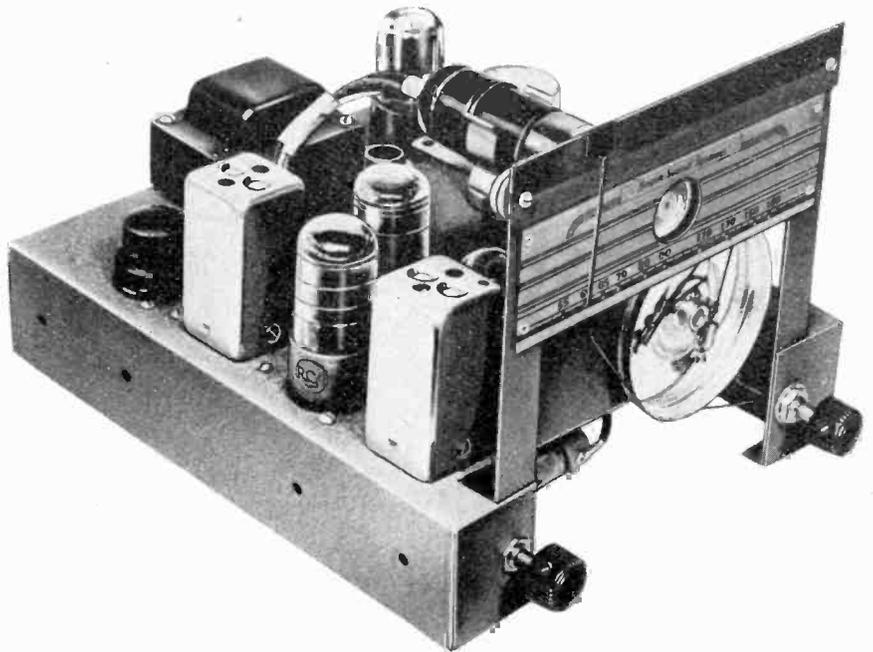
Fig. 16 A radio tuner especially designed for use with PA systems—made by the Bogen Company.
