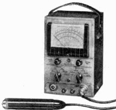
voltages up to 1000 volts and resistances of from zero to 1,000 megohms.
