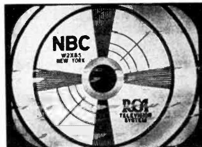
Fig. 18. A test pattern showing the effects of excessive auto ignition interference.
