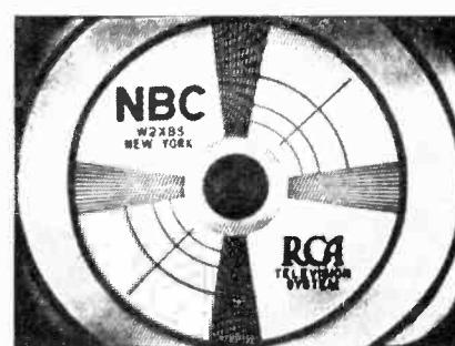
Fig. 20 Beat frequency interference produced by drifting stray carrier.
