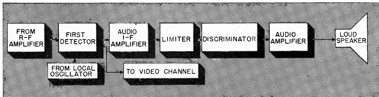
Fig. 2 A partial block diagram of a television receiver showing the audio and video channels. At the output of the first detector, the video and audio signals separate and feed into their respective intermediate frequency amplifiers.
