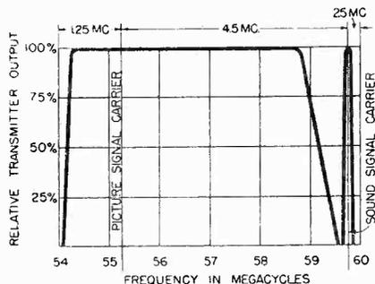
Fig. 1 The combined video and audio channels of a typical television station.
