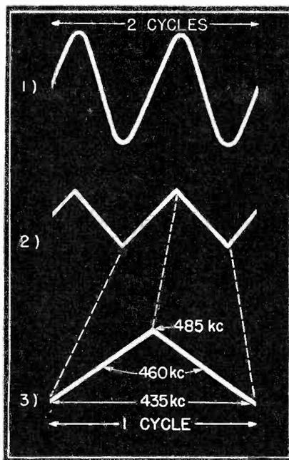
**Fig. 4** A pyramid saw-tooth wave. (1) is the 60-cycle line voltage wave from which it is developed.
