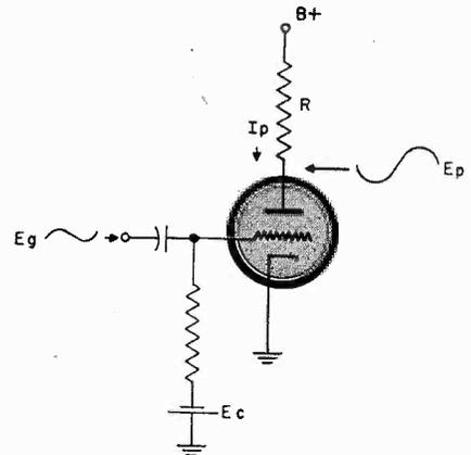
Fig. 2 The plate voltage variation is an amplified version of the signal fed to the grid.
