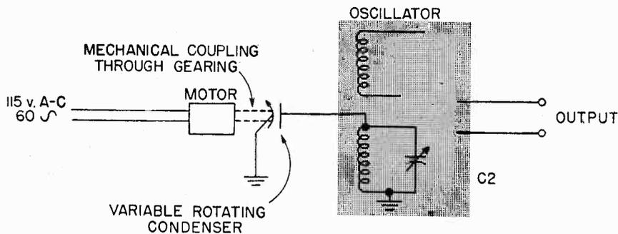
Fig. 2 A sweep frequency modulated signal generator using a motor-driven rotating condenser.
