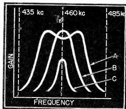
Fig. 1 Intermediate frequency curves with various degrees and types of transformer coupling. A is for double tuned transformer coupling when overcoupled. B is double tuned transformer coupling at critical coupling. Single tuned coil or single tuned transformer coupling gives a similar curve. C is the curve for double tuned transformer coupling when undercoupled.
