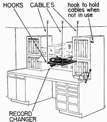
at the ends of the chains to hold the changer being worked on, as shown in the diagram. A hook or wire placed on the upper corner of the bench serves to keep the chains out of the way when they are not in use.
