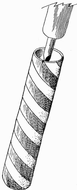
ameter. One end of the tubing is plugged with a piece of wood cut to fit. A piece of sheet iron or aluminum is tacked to the inside end of the plug to protect the wood from the hot iron. The tube is then
