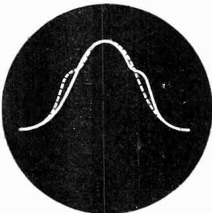
Fig. 9 The same intermediate frequency response as that shown in Fig. 8 with the oscillograph sweep synchronized at twice the former rate. The solid line indicates the response for the half cycle at increasing frequency, and the dotted line represents the response at the decreasing frequency half cycle.
