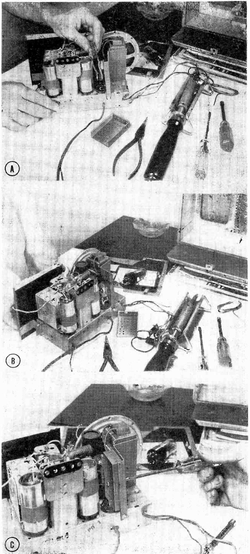
**Fig. 10** Steps followed in installing a selenium rectifier. The unit is mounted above the rectifier tube socket, and a shield is placed over it as illustrated.
