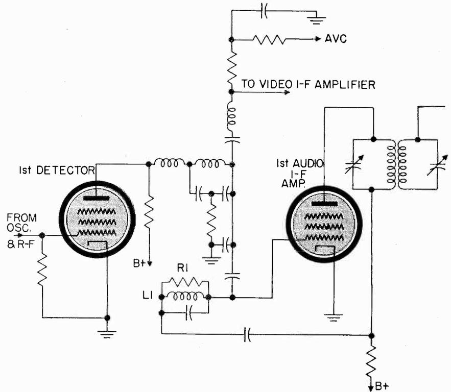
Fig. 6 Simplified diagram of first detector and first audio IF amplifier stages showing the parallel resonant circuit which is used to select the audio carrier and reject the video signal.
