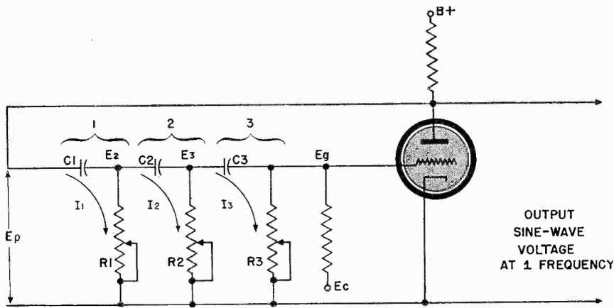
Fig. 4 A simplified schematic of the phase shifting network used in a phase-shift oscillator.
