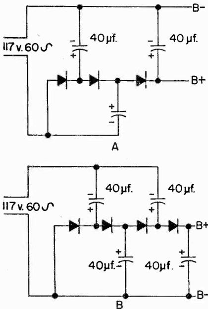
Fig. 7 A is a voltage tripler circuit using three 200 ma selenium rectifier units. B is a voltage quadrupler circuit using four 200 ma selenium rectifier units.
