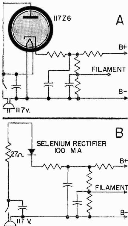
**Fig. 9** A is a typical power supply circuit using a 117Z6. B is the same power supply circuit after conversion to a selenium rectifier unit.
