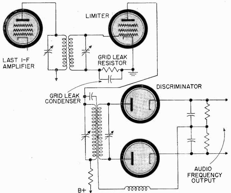
Fig. 7 Simplified diagram of the limiter and discriminator circuits. The limiter shown above uses grid leak bias.
