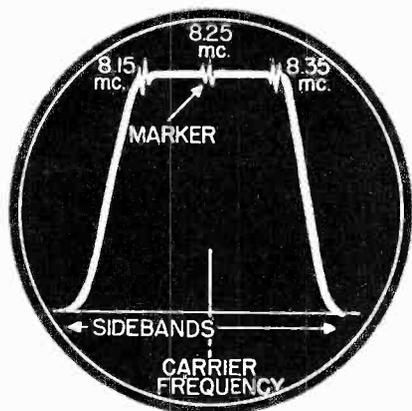
**Fig. 3** Typical response curve of a tuned IF amplifier as used in the audio system of a television receiver.
