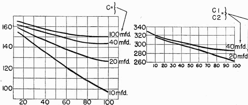
Fig. 6 A shows the voltage regulation curves of a half wave rectifier using a 100 ma miniature selenium unit. B shows the voltage regulation curves of a voltage doubler circuit using two 100 ma units.
