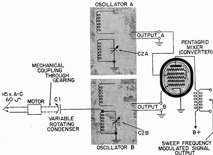
Fig. 3 Sweep frequency modulated signal generator using the double oscillator method. The sweep frequency remains constant for all center frequencies.
