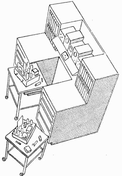
and can be moved in and out of the test position at will. In this way a disassembled set can be moved about the shop without difficulty.
