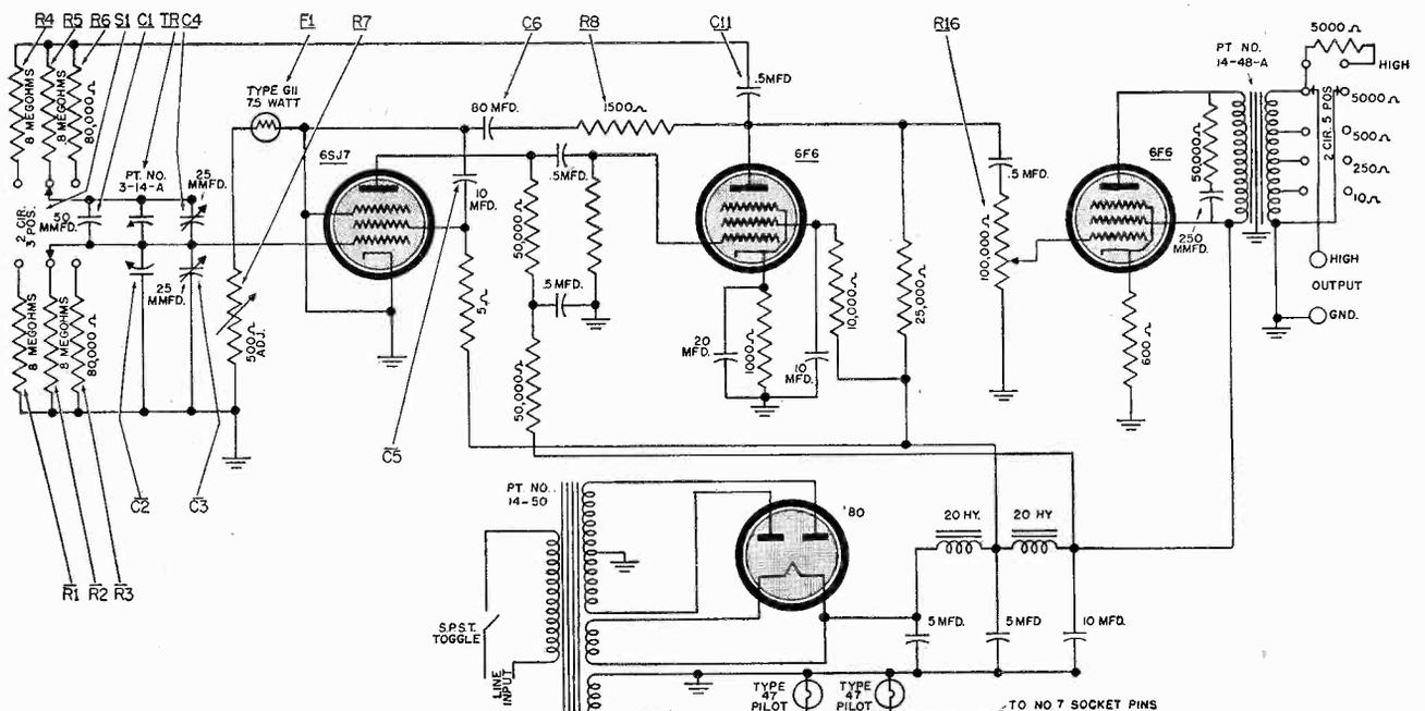
Fig. 6 A complete Wien bridge type audio oscillator.
