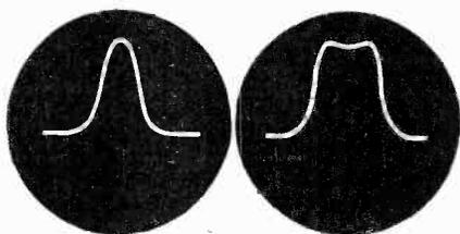
Fig. 10 The response traces for two different degrees of selectivity: On the left for sharp, and on the right for broad.
