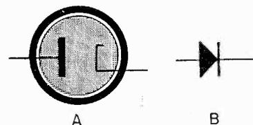
Fig. 4 A is the symbol for a vacuum tube diode, and B is the symbol for a dry metal rectifier.
