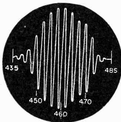
**Fig. 5** Wave form appearing across the secondary of an IF transformer when using a frequency swept signal. The actual wave as it appears on the 'scope will fill in.
