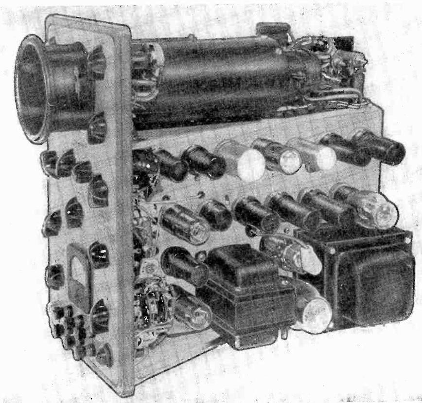
**The internal construction of the new oscilloscope shown in the lower right hand corner of the page. This 'scope is characterized by a wide frequency range and high gain.**
