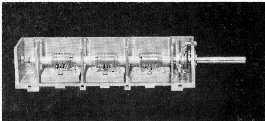
**The Inductuner, a unit developed by Du Mont Labs. It provides an extremely wide tuning range from approximately 49 to 210 megacycles. Provision is made for RF stage, mixer stage and oscillator stage tuning.**
