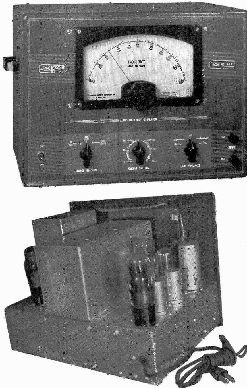
Fig. 1 The Jackson Audio Oscillator Model 652. This is an example of a well designed Wien bridge audio oscillator. Note the conveniently arranged controls and good internal construction.
