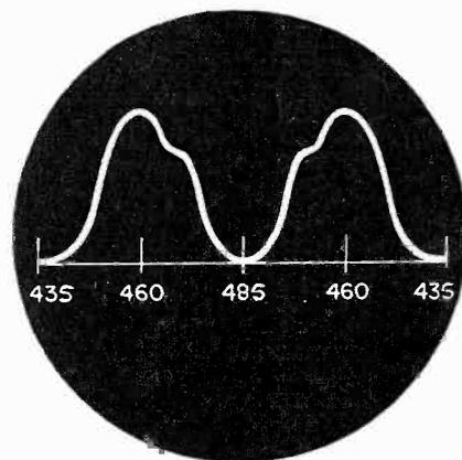
Fig. 8 The appearance of an improperly adjusted IF amplifier with the oscillograph synchronized at a rate of one sweep per rotation of the motor-driven condenser. If a reactance tube modulator is being used, the synchronization is at power line frequency.
