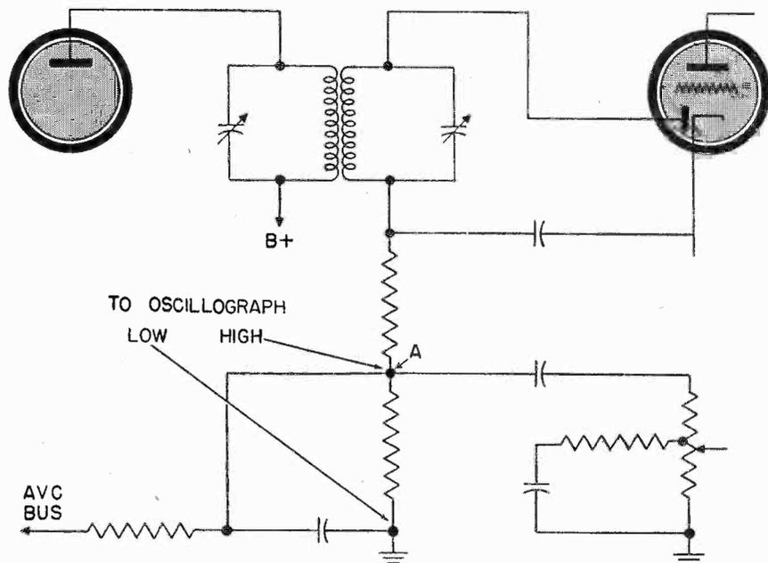
Fig. 6 Points at which the oscillograph leads are connected to a receiver using a diode second detector.
