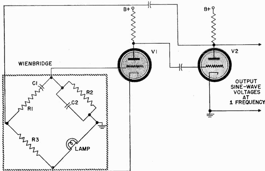
Fig. 5 A simplified schematic of a Wien bridge audio oscillator.
