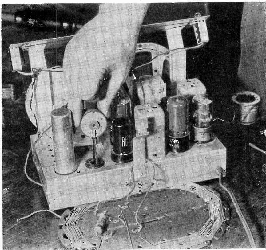
Fig. 1 A selenium rectifier being placed in mounting position above the rectifier socket of a small table model receiver.
