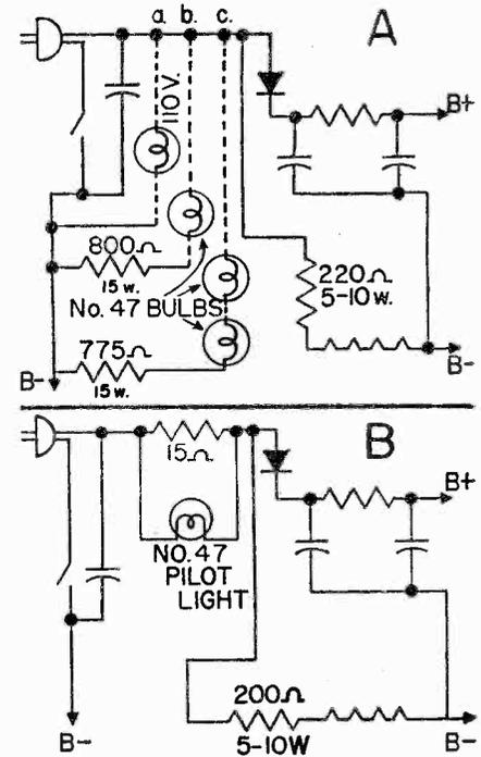
Fig. 12 Four ways in which the pilot light may be connected when converting a power supply using a 35Z5 rectifier to a selenium rectifier unit.
