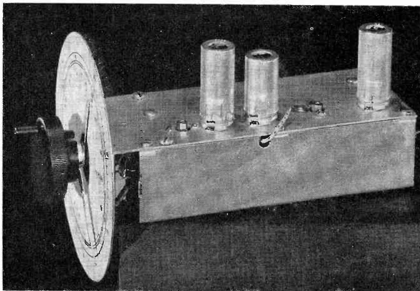
**The Inputuner, in which the Inductuner is used. The three shields cover the RF, mixer and oscillator tubes.**
