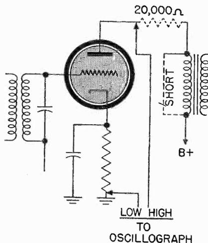
Fig. 7 Points used when connecting the oscillograph to a receiver using biased detector. A 20,000 ohm resistor is inserted in the plate circuit and the primary of the transformer is shorted out.
