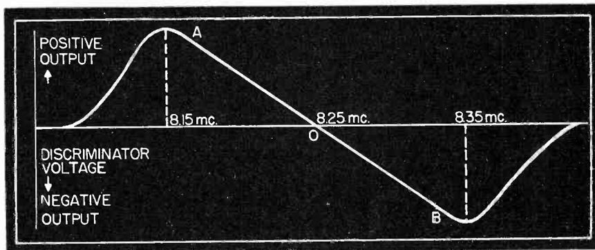
**Fig. 5** Characteristic response curve of a typical discriminator as used in a television receiver.
