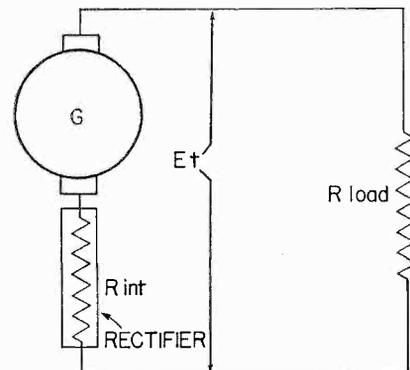
Fig. 5 Simplified diagram illustrating the effect of the rectifier internal resistance on the output voltage.
