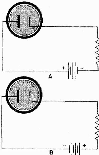
Fig. 8 In circuit A, current will flow through the diode. In circuit B, current will not flow through the diode. C is the effective circuit of an ohmmeter connected across a selenium rectifier. The meter reads 10,000 ohms. When the leads are reversed, as in D, the meter reads 100,000 ohms. The greatest current flow is, therefore, with the connections of C.
