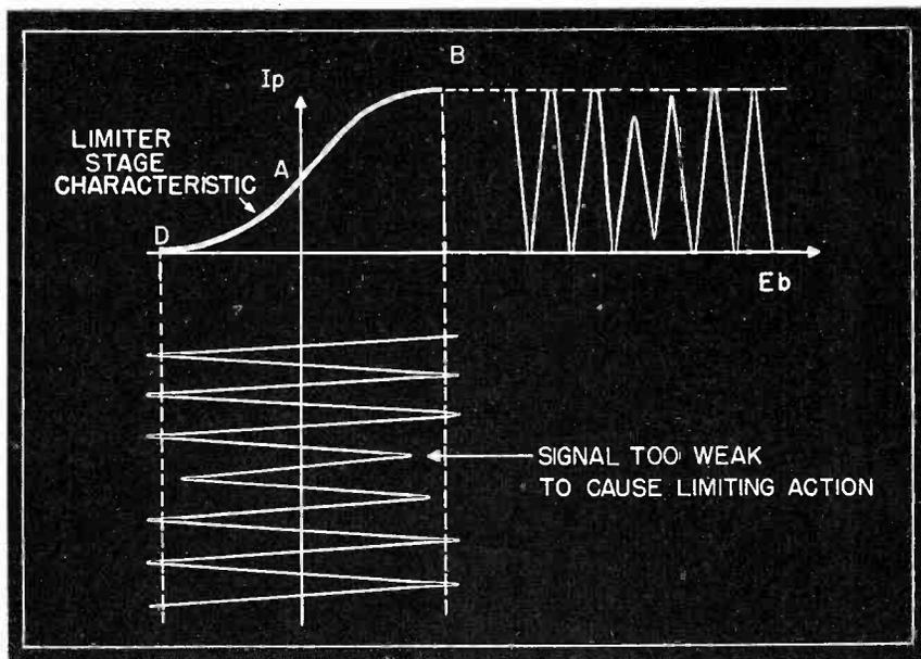
**Fig. 4** Limiter stage response curve showing the limiter action on the signal. When the signal is not strong enough to reach points B and D and saturate the limiter, no limiting action occurs.
