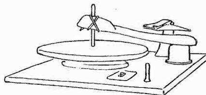
gram. The arm is placed near the top of the spindle and an elastic band is wound back and forth around them.
