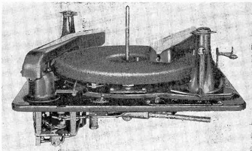
Fig. 2 The slicer type record changer. This changer is equipped with a recording as well as a playing head.
