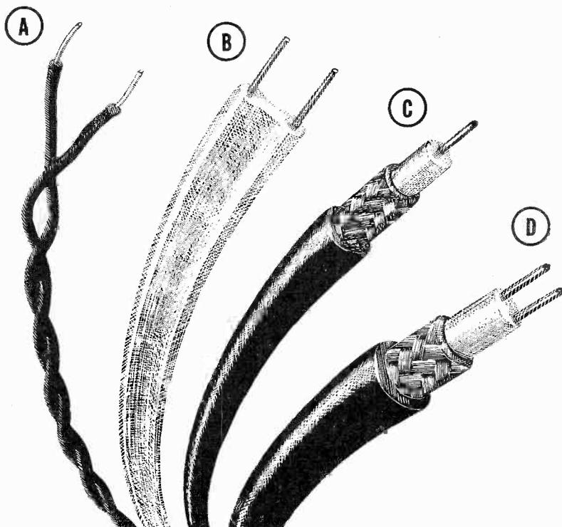
Fig. 1 Four types of transmission line now being used with FM and television antennas: (A) Twisted pair; (B) Two wire parallel conductor; (C) Coaxial cable; (D) Shielded parallel pair.
