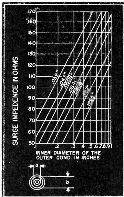
Fig. 5 A chart showing the impedance of concentric transmission line (air dielectric) for different combinations of inside and outside conductor sizes.
