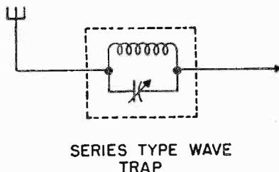
Fig. 6 A series type wave trap which can be constructed from an RF choke and a trimmer condenser.
