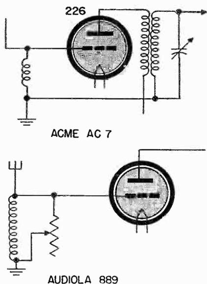
Fig. 1 In the older TRF's, the antenna is usually connected directly to the grid of the first RF amplifier as shown in the simplified schematics above.
