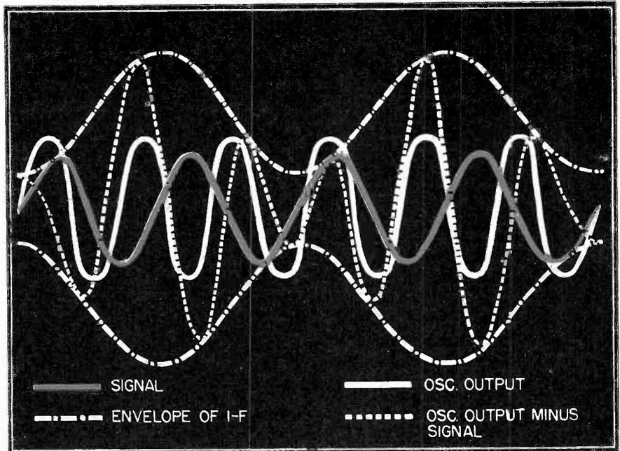
Fig. 2 Pattern showing the incoming signal, the oscillator output and the signal at the input to the IF.
