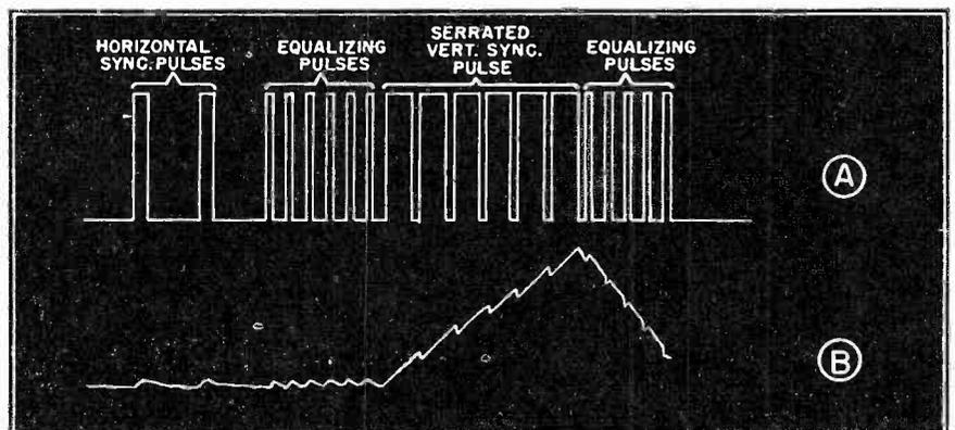
Fig. 6 A, a composite sync signal showing the horizontal sync pulses, the equalizing pulses and the vertical serrated sync pulses. B, the separated vertical sync pulse after it passes through the integrating circuit.
