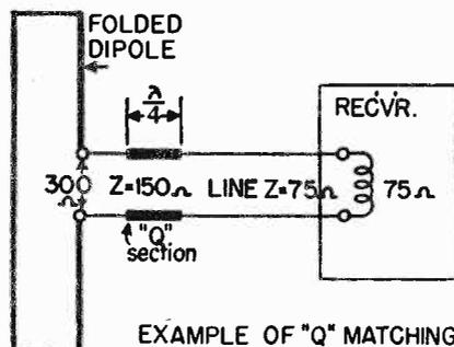
Fig. 7 A matched system using a Q section. The Q section acts as a transformer. To obtain desirable efficiency, the conductors used in the Q section should be of fairly large diameter.
