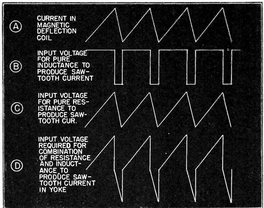
Fig. 8 The waveforms necessary to obtain magnetic deflection: A, the waveform of the current in the magnetic deflection coil; B, the input voltage necessary to produce a saw-tooth current in a pure inductance; C, the input voltage necessary to produce a saw-tooth current in a pure resistance; D, the input voltage required to produce a saw-tooth current in a combination resistance and inductance such as found in the yoke.
