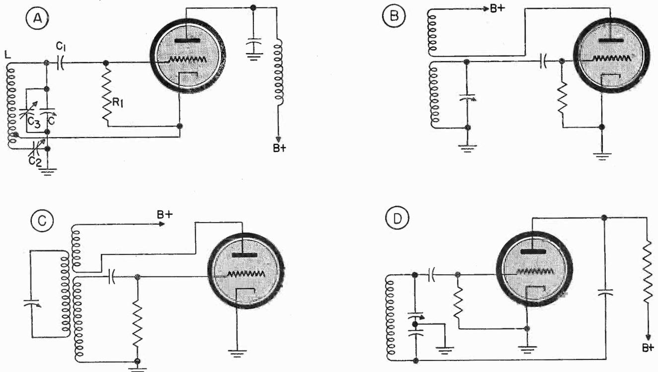
Fig. 3 Four types of oscillator circuits: A, a modified Hartley; B, a tickler feedback type; C, a Meissner; D, a Colpitts.
