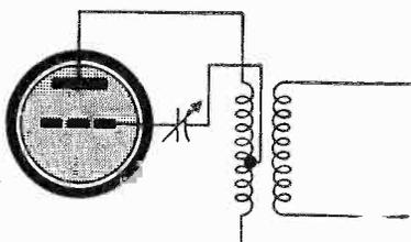
Fig. 4 Method used to neutralize a stage to prevent oscillation and instability.
