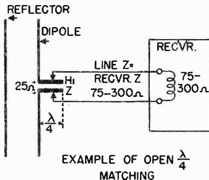
Fig. 8 An open end quarter wave stub used to match a 75 or 300 ohm line to a 25 ohm antenna.
