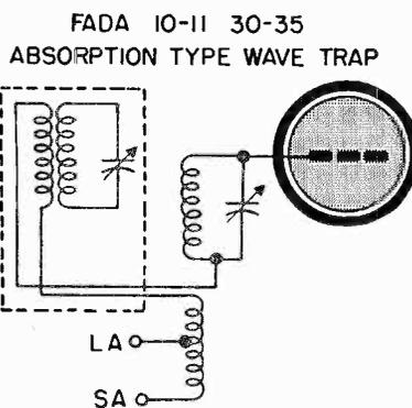
Fig. 5 An absorption type wave trap.
