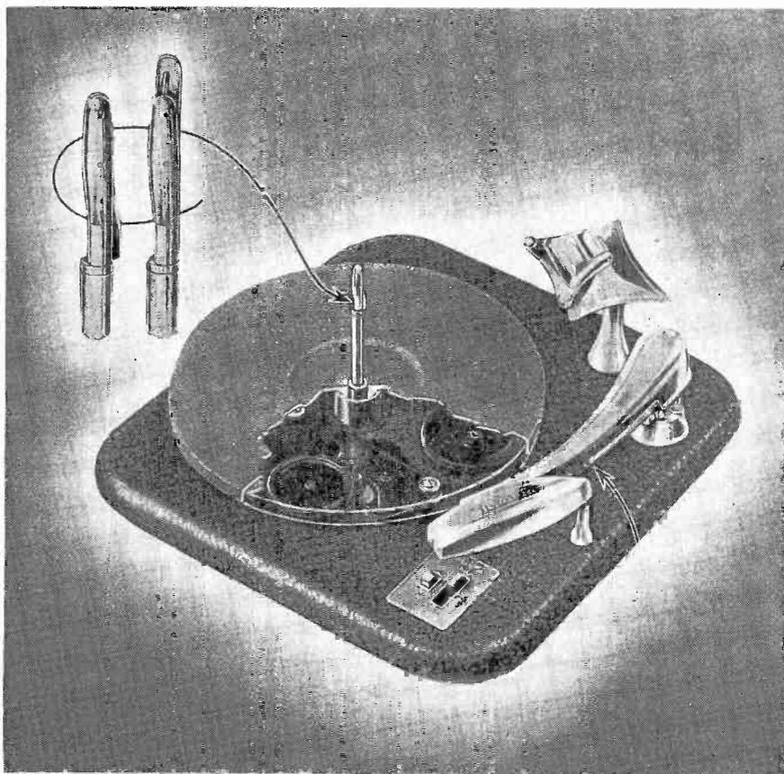
Fig. 3 A toggle post changer with an enlarged view of the spindle. The spindle on the left is in normal position; the spindle on the right is in position to drop a record onto the turntable.
