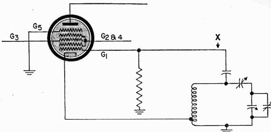
Fig. 7 6SA7 pentagrid converter.
