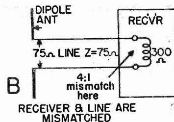
Fig. 6 Correctly and incorrectly matched antenna systems. In (A) the 75-ohm line matches at both the antenna and receiver ends; and, therefore, the match is correct. In (B) the 75-ohm line matches the antenna but does not match the input of the receiver.
