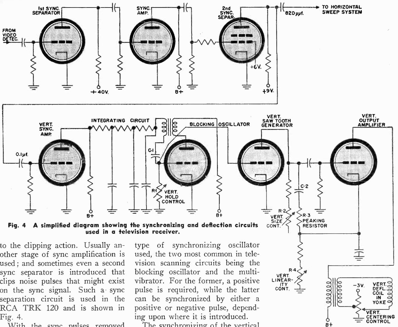
Fig. 4 A simplified diagram showing the synchronizing and deflection circuits used in a television receiver.
