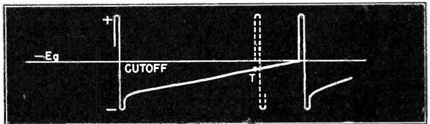
Fig. 7 The waveform of the signal on the grid of the blocking oscillator tube.
