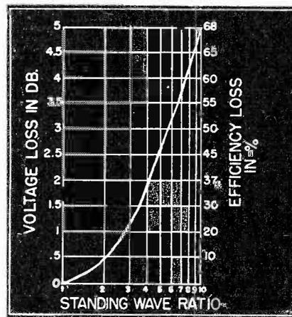
Fig. 2 A curve showing the voltage loss in db and the efficiency loss in per cent for various standing wave ratios.
