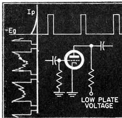
**Fig. 3** Simplified circuit of a triode clipper and its input and output waveforms.
