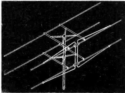
**Fig. 8** The S/C Laboratories stacked array, consisting of two dipoles, one above the other, with a reflector behind each dipole. This type of antenna gives both horizontal and vertical directivity.
