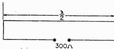
**Fig. 4** A folded dipole. The center impedance of this antenna is 300 ohms which can be matched by standard twin parallel conductor transmission line.
