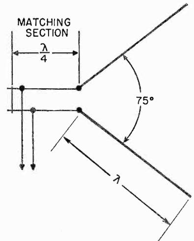
**Fig. 12** The rhombic antenna. This antenna gives a low angle of reception and comparatively wide band coverage.
