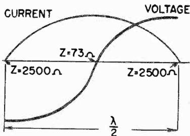
Fig. 1 The voltage and current distribution as they appear on a half wave dipole.
