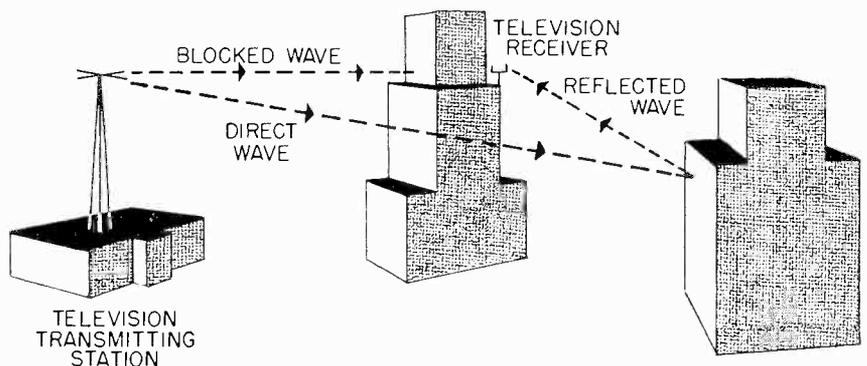
Fig. 16 The above figure shows the way in which a reflected wave can be used to obtain satisfactory reception.
