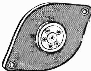
hole. The wafer socket is mounted in the usual manner and the miniature socket is placed in the hole and held by its retaining ring.
