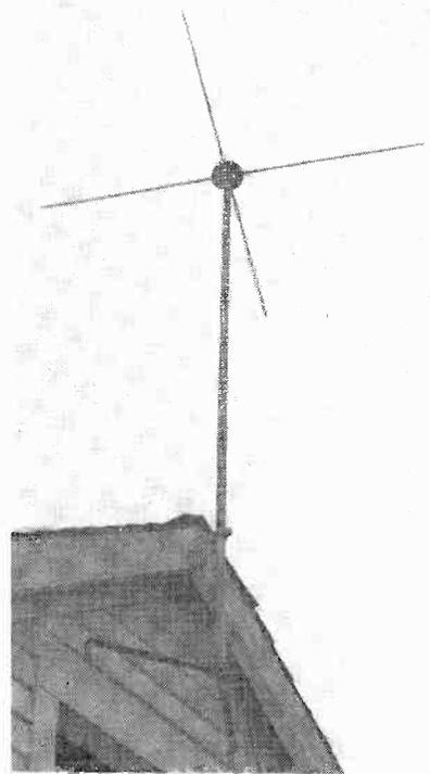
**Fig. 13** The Workshop Associates non-directional antenna. In locations where signals must be received from widely different directions and no trouble is experienced with reflections, this antenna will give excellent results. In areas where the signal strength is low or there are serious reflected signals, this antenna can be converted to a three-element parasitic beam, using a kit supplied by the manufacturer. The heading of the article shows the converted antenna.
