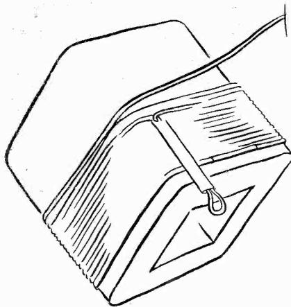
**Fig. 3** The taps are made by twisting a pigtail of wire and bringing it to the edge of the winding between layers of insulating paper. The taps may be tagged or identified by their length.
