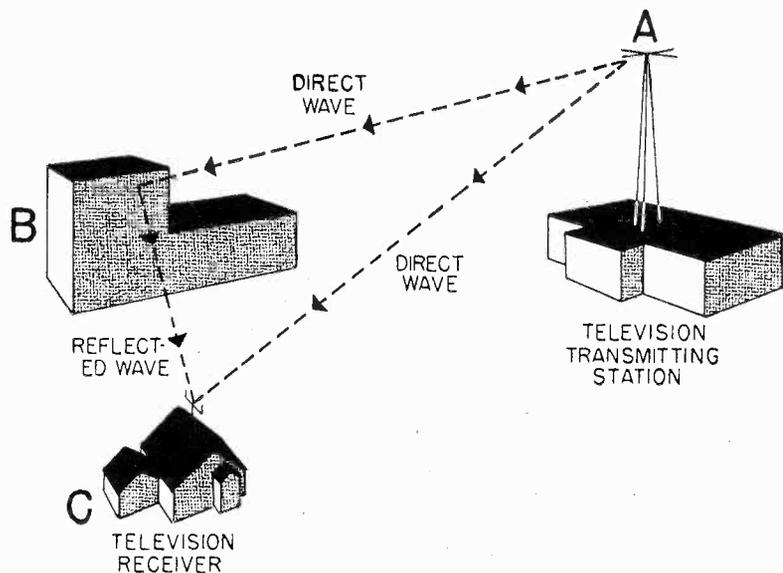
**Fig. 6** As shown above, a reflected wave reaching the antenna of a television receiver follows a longer path than the direct wave. When this phenomenon takes place, the result is a distortion of the picture which is commonly known as a "ghost."
