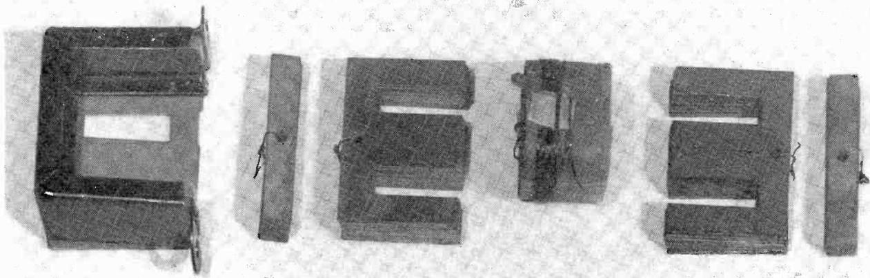
Fig. 1 The completely disassembled transformer ready to rewind.
