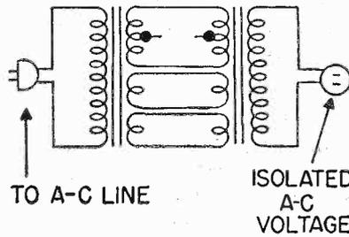
ratings can be used by connecting the filament windings so that they increase or decrease the output voltage. If hum is noticed in the set under test, the chassis can be grounded and will still be independent of the AC line.
