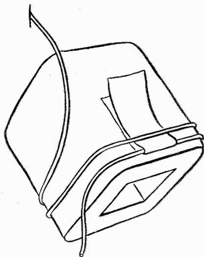
**Fig. 2** As shown above, when starting the winding, a piece of paper is used to hold the first turn in place.
