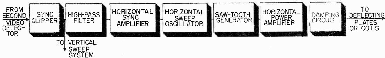
Fig. 1 A block diagram of the horizontal sweep channel of a television receiver.
