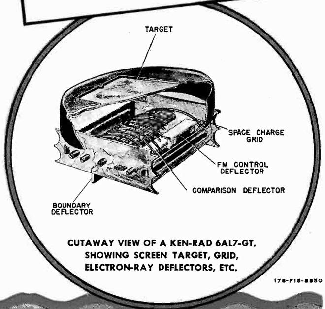
CUTAWAY VIEW OF A KEN-RAD 6AL7-GT, SHOWING SCREEN TARGET, GRID, ELECTRON-RAY DEFLECTORS, ETC.
