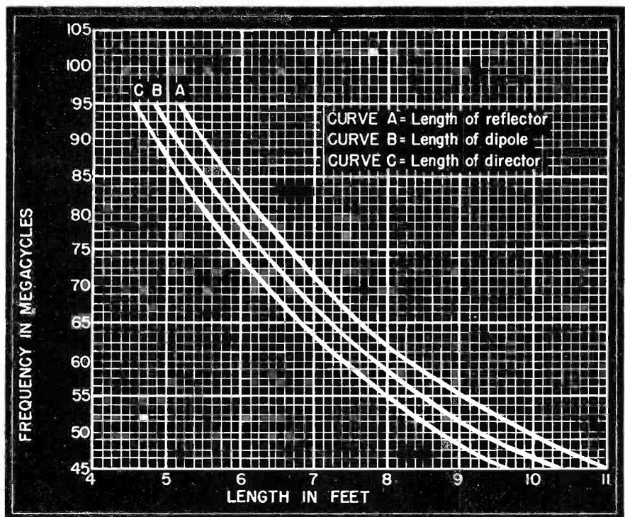
Fig. 2 A curve showing the length in feet of a dipole, a reflector or a director for frequencies from 45 to 95 mc.
