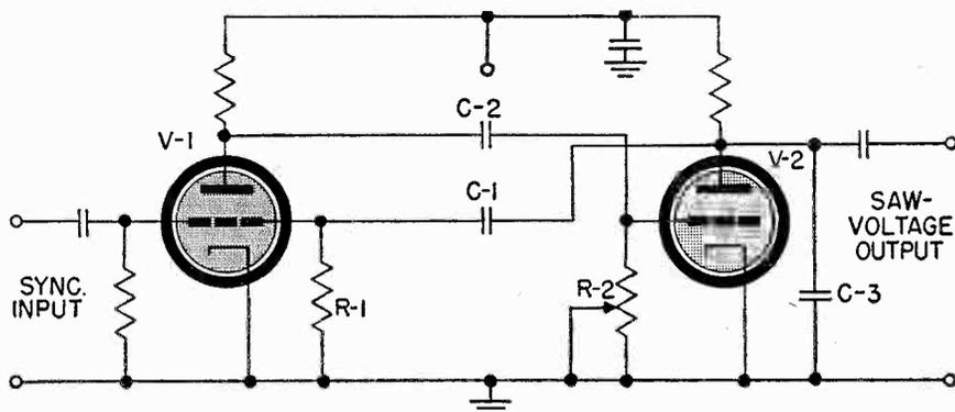
Fig. 5 Circuit diagram of a multivibrator with provisions for synchronization.
