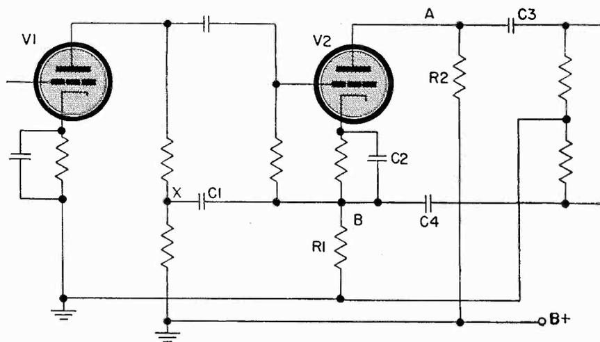
Fig. 4 A phase inverter utilizing the cathode follower principle. While this circuit requires only one triode, circuit values are much more critical than those of the two-tube phase inverters.
