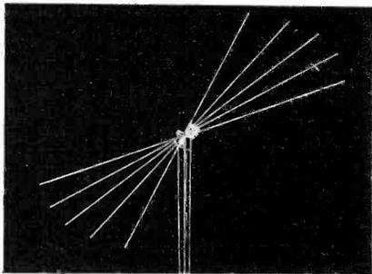
**Fig. 10** The Andrew Di-Fan antenna. This antenna covers an extremely wide band of frequencies without serious attenuation.
