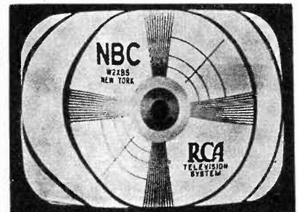
Fig. 9 A test pattern showing horizontal non-linearity.
