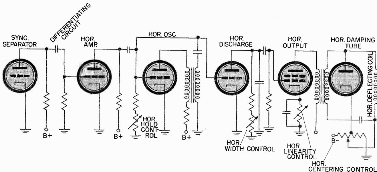
Fig. 2 A partial schematic diagram of the horizontal sweep system of the television receiver.
