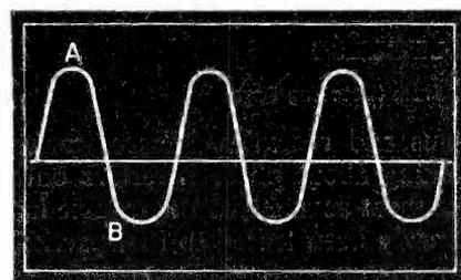
**Fig. 6 Distortion of the wave form which results from an improperly balanced phase inverter circuit. The positive peak is of higher amplitude than the negative peak. This condition results in harmonic distortion.**
