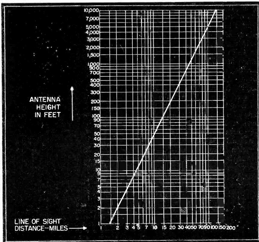
**Fig. 9** The above graph shows the relation between antenna height and line of sight transmission distance.
