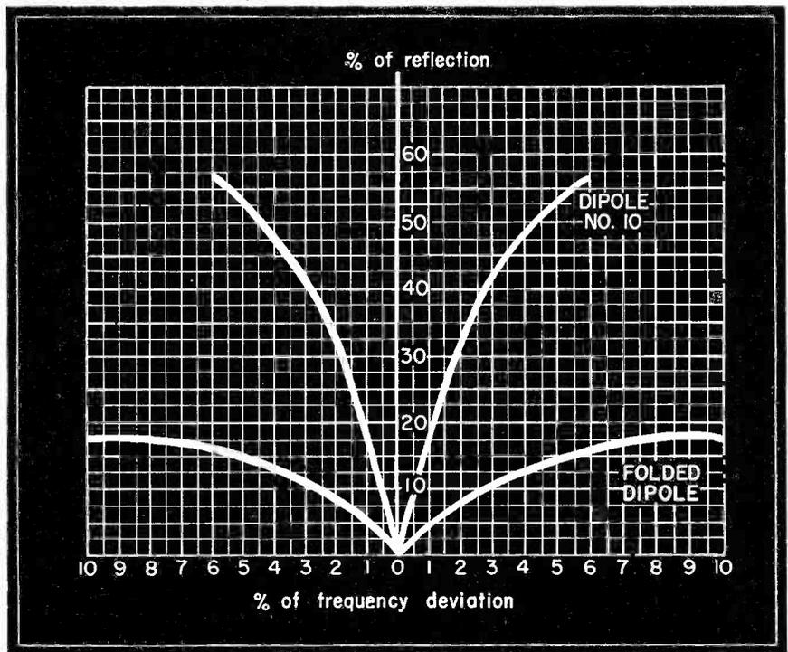
**Fig. 5** Curves showing the comparative band widths of a folded dipole constructed of 1" tubing and a simple dipole constructed of #10 wire.
