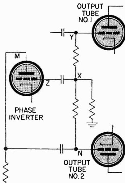
Fig. 3 A partial circuit diagram of the self-balancing type of phase inverter. In this circuit negative feedback is used to balance the signals on the grids of the two tubes used in the phase inverter.
