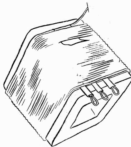
**Fig. 4** As the winding is completed, a piece of insulating paper is used to hold the last turn in place as shown above.
