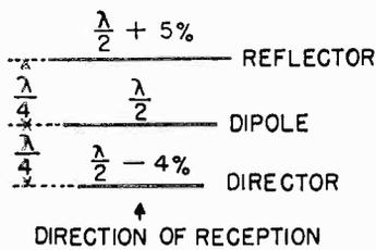
**Fig. 7** A parasitic beam which consists of a dipole, a reflector and a director. Quarter wave spacing between the elements is used. The reflector should be approximately 5% longer than the dipole, and the director should be approximately 4% shorter than the dipole.
