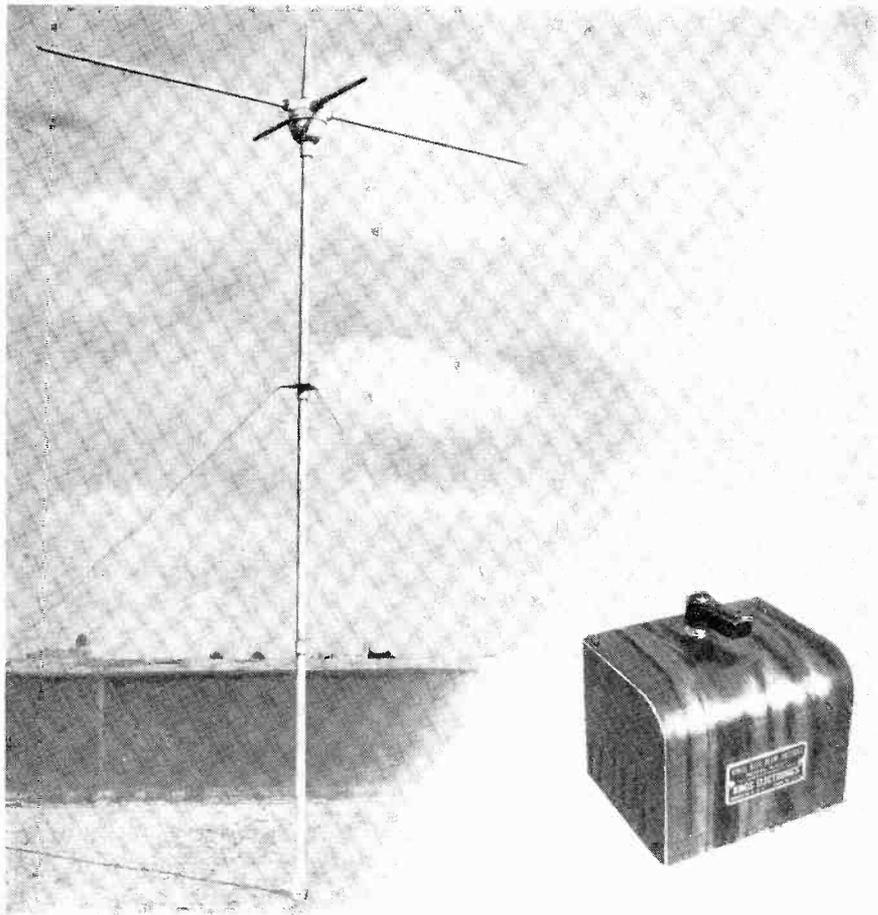
Fig. 15 Kings Electronics antenna which consists of two dipoles set at right angles to one another and cut for two different frequencies. The antenna can be rotated from a remote control box located at the receiver.
