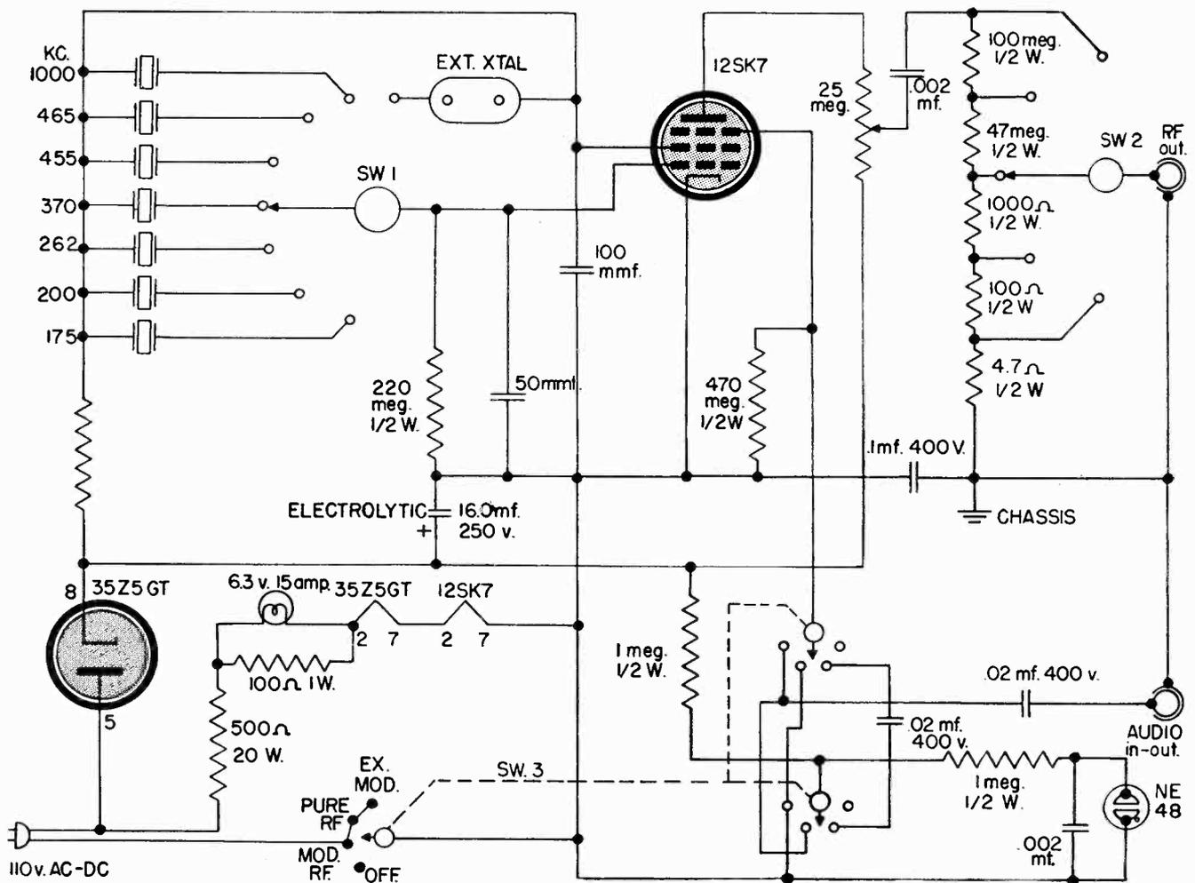
Fig. 2 Complete circuit diagram of the Bliley CCO.
