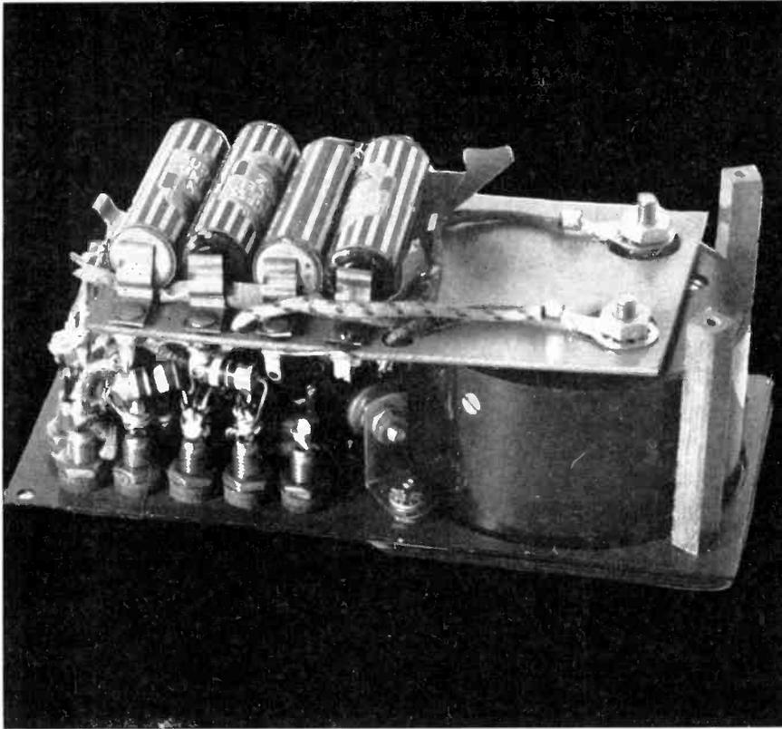
**Fig. 2** Miniature type of multimeter especially useful for portable work. Switches are eliminated by the use of a large number of tip jacks.
