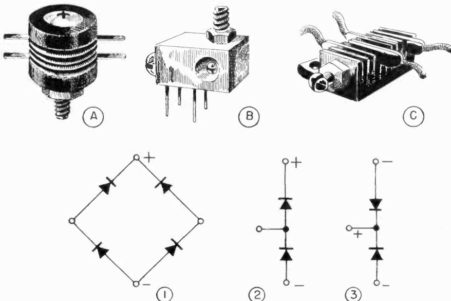
Fig. 3 Types of copper oxide rectifiers which the serviceman is likely to encounter in servicing his own test equipment. (See text.)
