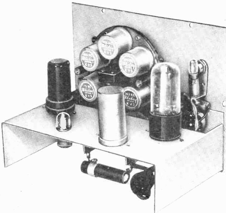
Fig. 1 The Bliley CCO with the case removed. The seven crystals are mounted around the rotary switch and held in place by the large round plate.
