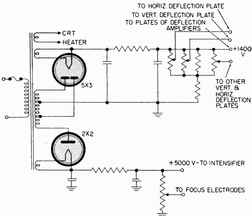
**Fig. 3** A circuit diagram of a high voltage and low voltage power supply for a television receiver using an electrostatically focused and deflected tube.
