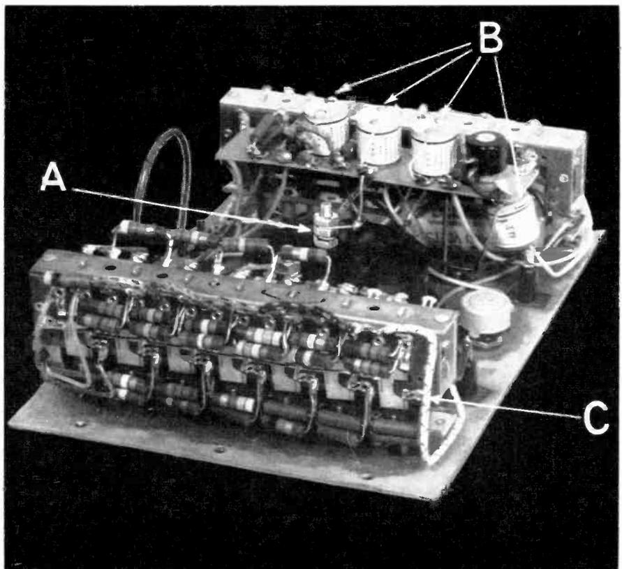
Fig. 1 Internal view of a typical volt-ohm-milliammeter, showing copper oxide rectifier (A,) precision resistors (B,) and push-button switch assembly (C.) Proper care of these and other parts is explained in the text.
