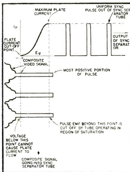
Fig. 2 Graph illustrating the variations of plate current with grid voltage changes
