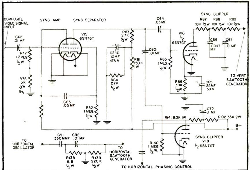
Fig. 5 Four triodes serve as sync amplifier, separator, and clipper (DuMont). This design assures sufficiently high amplitude, freedom from noise and hum
