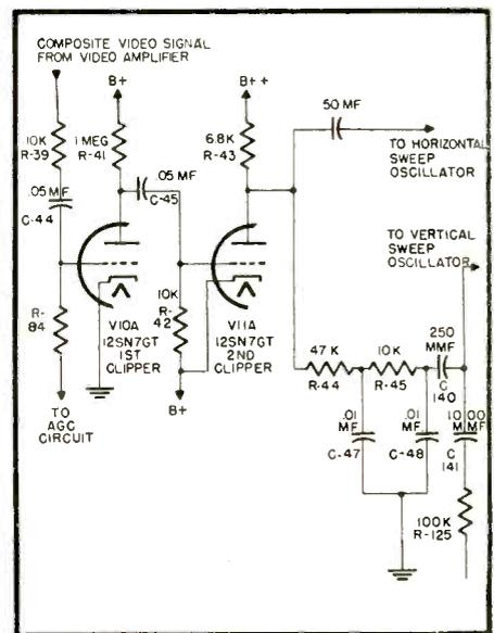
Fig. 3 Some Motorola receivers contain this dual triode which acts as a double clipper
