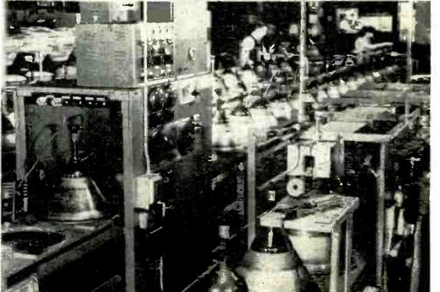
Railroad exhaust. A nearly perfect vacuum is obtained as each tube passes through the various evacuation processes automatically. The tubes pass high-temperature ovens to drive all the gases out of the tube material.
