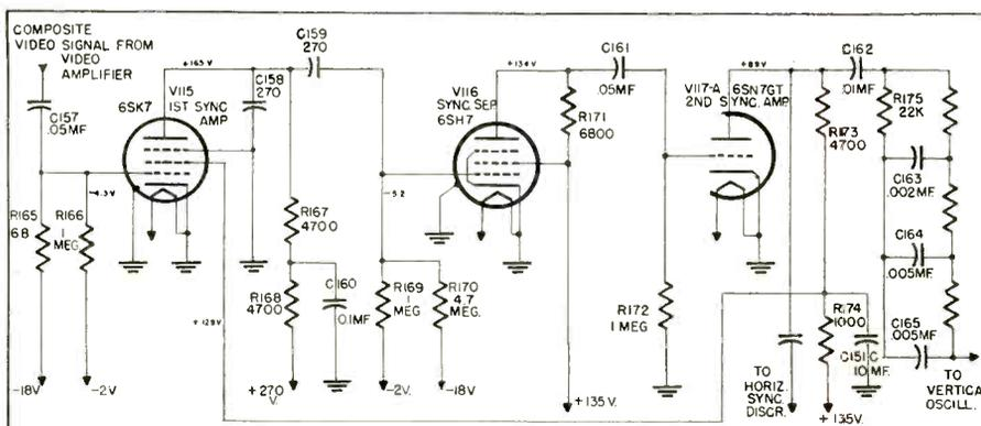
Fig. 6 RCA and Ansley receivers use the network shown above, using two pentodes and a triode for sync separation, clipping action removes amplitude variations
