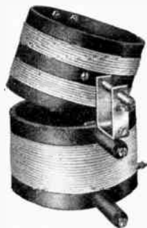
R-93 Specially Designed Coupler for Using Antenna
