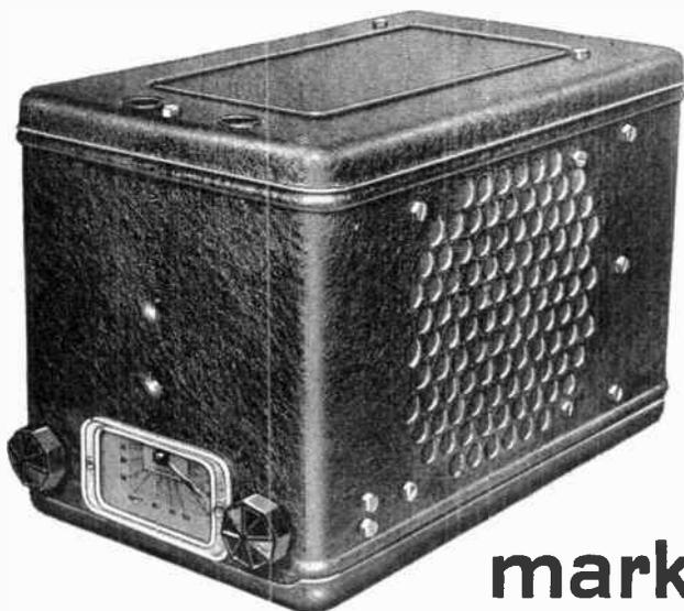
Self-contained as it is, the Crosley Roamio "4A1" can be easily installed in any car with the controls convenient to the driver, either to the right or left of steering wheel. The airplane type dial appears just below instrument panel.
