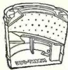
In addition to Power-Air fuel savings, the exclusive Duo-Therm Burner gets *more heat out of every drop of oil*. That's because it mixes air and oil in 6 stages (only the Duo-Therm Burner does this!) for clean, efficient operation from low pilot to highest flame.
