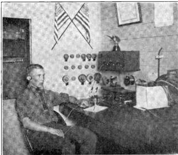
Mr. Lester has indeed a first-class station and we extend to him our compliments for the neatness and appearance of his apparatus. The transmitter is a 1-K.W. spark type and the receiver a home-made regenerative set.
