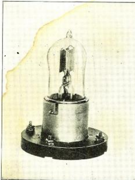
Fig. 24. A So-Called V.T.-21 and its Socket, a Tube Which Has Been Much Used by the U. S. Signal Corps.
