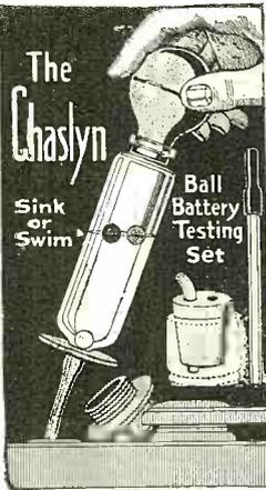
Just insert nozzle in cell and draw up some acid; then, without removing from cell, "read" the condition of acid by the way the three balls of differing colors and densities sink or swim.
