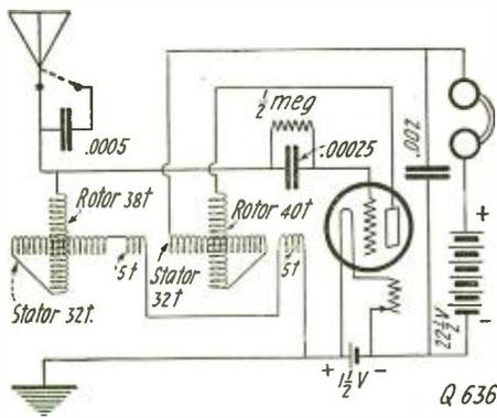
Diagram of the Aeriola, Sr. Receiver. Two Variometers Are Used, One as the Tuning Unit and the Other in the Plate Circuit.
