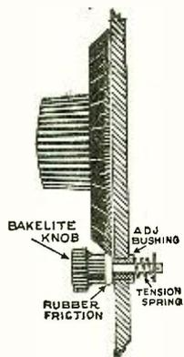
This is one of the best aids to fine tuning yet produced. To attach, just drill 1/4 inch hole in the panel, insert the bushing and shaft and replace the cotter pin. The tapered adjusting bushing takes up wear as well as inaccurate drilling and the spring
