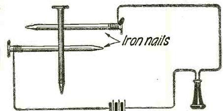
Fig. 20. The Hughes' Nail Microphone Its Function Resting on Imperfect Contact.
