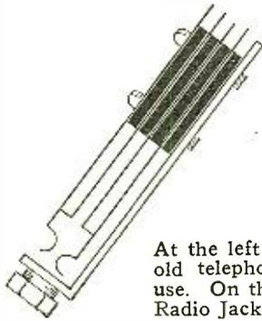
At the left is an adaptation of the old telephone jack sold for radio use. On the right is the Improved Radio Jack. Notice no soldering is necessary, the small compact size, the short leads which reduce capacity effects. Any standard plug fits the Improved Jack. Price \$1.00.
