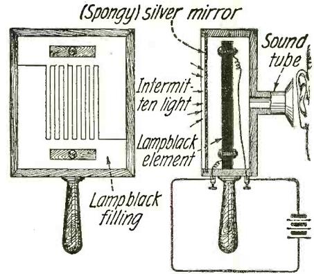
Figs. 17-18. Bell's Photophone. It Can Speak, Sing, See, Hear and Feel Electricity and Magnetism Aside from a Few Other Choice Accomplishments.
