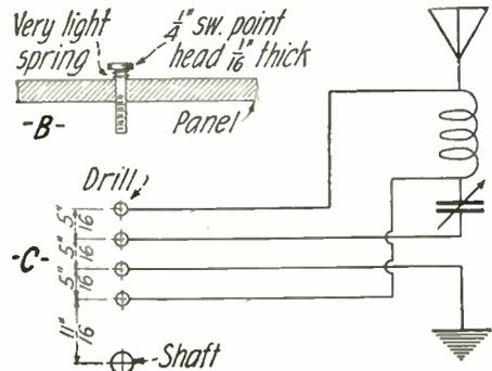
The Layout and Connections for the Series-Parallel Switch. Small Springs Underneath the Switch Points Provide the Necessary Friction Contact Against the Brass Strips.
