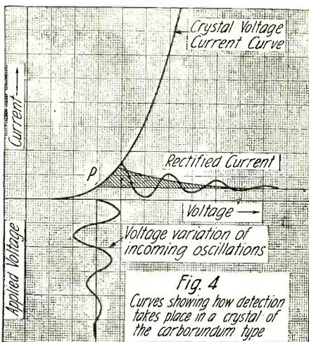
Fig. 4 Curves showing how detection takes place in a crystal of the carborundum type
