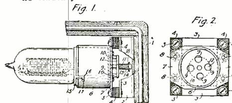
silient portions 4, on which the socket and tube are mounted, prevents any vibrations or jars contributed to the casing to which the bracket 2 is attached, from seriously affecting the lamp.
