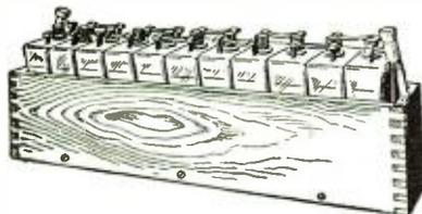
was found to be 7.07 ampere hours. The over-all dimensions of the battery are 17" long, 4" wide and 5" high. The end cells of the group of 11 are provided with binding posts for connections to the set. The active plate area of this type is about  $6\frac{1}{4}$  square inches. The vent plugs on this type are made of hard rubber and screw into suitable threads on the top of the composition filling the tops of the cells. Lead strips are used for connecting individual cells.
