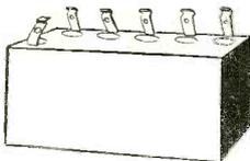
which would produce noises in a vacuum tube receiver and the operation was found to be entirely satisfactory. Fifteen flashlight cells of the larger size are moulded into a block of encasing sealing compound. Taps are taken off after 16½ volts in 1½-volt steps until the total of 22½ volts has been reached. Binding posts are provided for these taps.
