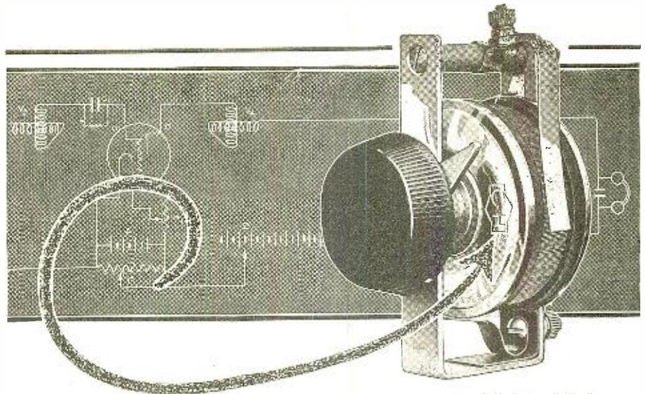
The C-H Radio "A" Battery Potentiometer.
