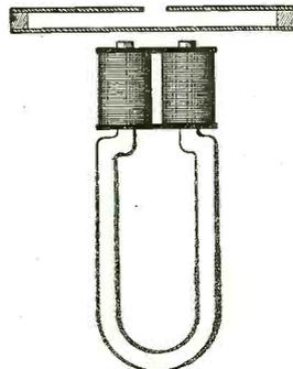
Fig. 13. A Receiver of the Magnetic Type Employing a Resonating Chamber in Conjunction with the Diaphragm.
