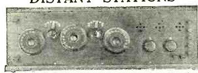
F. R. S. Complete Two-Stage Long Range Receiver Set includes two "Audio" transformers, condenser, two moulded variometers, moulded variocoupler, three V. T. sockets, filament rheostats, dials, Read 'Em binding posts, switch points in attractive cabinet and drilled panel complete, ready to hook up. A \$125 Radio for..... **\$40**
