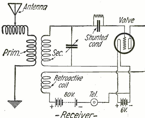
The Circuit of the Receiver. For Reception Over High Power Transmission Lines the Receiving Aerial Is Placed Parallel to Them.
