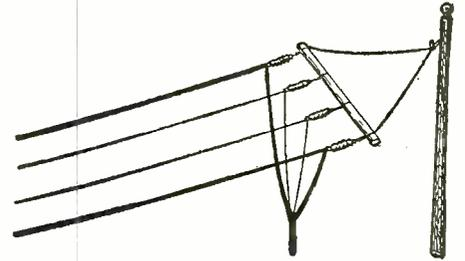
Showing the Distribution of R. F. Current in a Four Wire Flat Top Inverted "L" Antenna.
