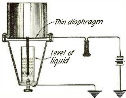
Fig. 6. A Receiver Produced by Gray. Vibration of the Diaphragm Caused Variations in the Distance Between Two Points Immersed in a High Resistance Liquid Thereby Varying the Battery Current in a Local Circuit.
