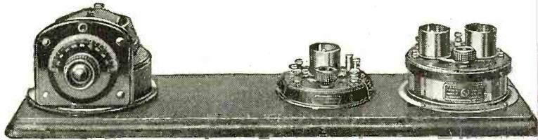
Complete Receiving Set—Coupled Circuit Tuner, Detector Unit and 2-stage Amplifier
