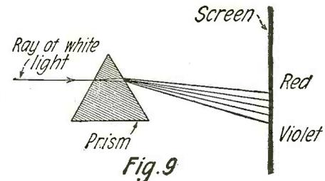
Showing How a Prism Refracts White Light and Resolves it Into Different Colors, Each Color Being Refracted a Different Amount on Account of Difference in Wave-lengths.
