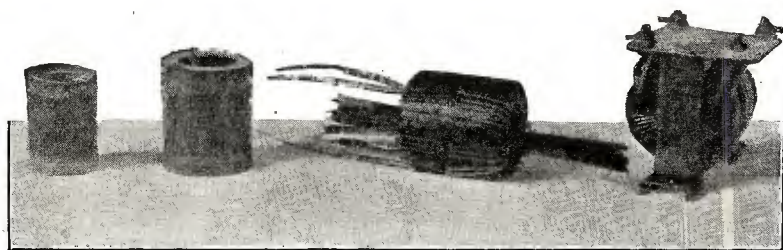
An Audio Frequency Amplifying Transformer, Constructed From Parts of a Ford Spark Coil.
