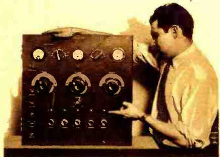
PILOT LIGHTS TELL WHAT IS HAPPENING BEHIND THE PANEL. Harold Herbert, the builder of the set, is pointing to the row of lights that indicate whether everything is functioning correctly within the receiver. © Kadel & Herbert.
