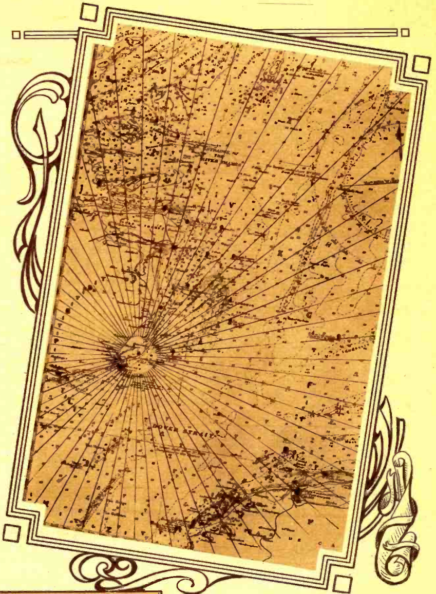
CHART OF THE RADIO LIGHTHOUSE. By means of a chart similar to the one above, mariners can determine their position at sea in relation to the transmitter at South Foreland. It will be noticed that every few degrees on the chart has its own letter, which is transmitted within those degrees only.
