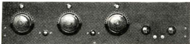
Fig. 2. Panel view of the receiver, showing the two switches for controlling the panel lights and the filaments of the tube.
