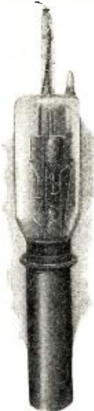
One of the high-power water-cooled vacuum tubes is shown at the left. The plate of the tube is the metal cylinder at the bottom, from which the heat is dissipated by the cooling water.
