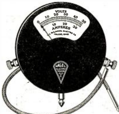
If you own a "Super-Het" or are operating your set with dry cells, you need this Nagel Voltmeter, a combination instrument for testing both A and B batteries.
