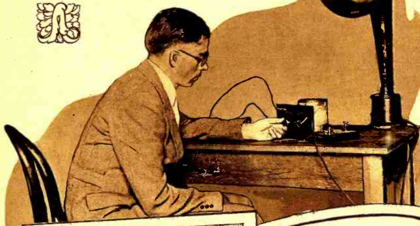
CRYSTAL SET OPERATES LOUD SPEAKER. In the Radio Laboratory of the Bureau of Standards in Washington, Morris S. Strock has succeeded in obtaining signals from a loud speaker using a crystal detector alone. He states that a big antenna and a good crystal are necessary. © Harris & Ewing.
