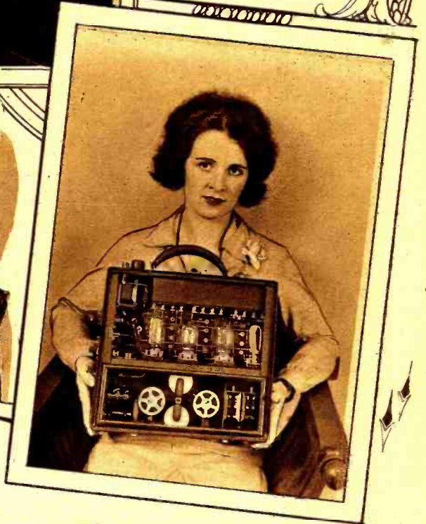
RECORDS BROADCAST MUSIC ON MAGNETIZED WIRE. In this four-tube reflex receiver is a magnetized wire on which is recorded broadcast music, which can be reproduced at any time. The recording mechanism can be seen in the bottom of the cabinet. © Kadel & Herbert.
