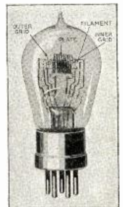
A double-grid vacuum tube that is manufactured in England. It has the same internal construction as that on the opposite page. A special socket is required for these tubes, as they have five connection prongs.
