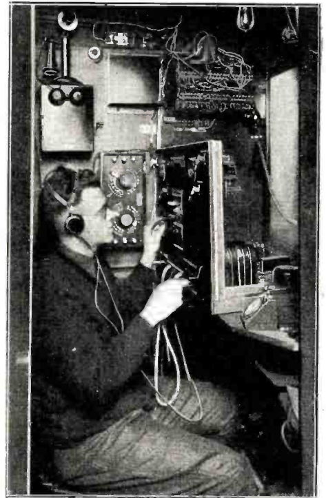
A monitor is in charge of the signals as they go from the land line to the radio link in the transatlantic chain.
