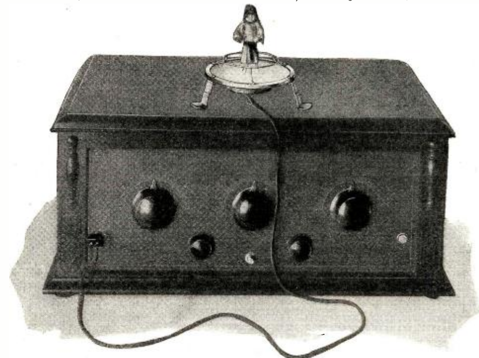
Complete view of the radio dancer and a standard radio outfit. It should be noted that this instrument works well only in connection with a set of at least three tubes. The dancer does not work on one-tube sets or crystal sets, as good loud speaker volume is needed for the operation of the device.
