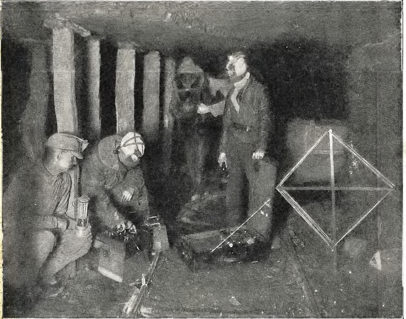
A portable experimental loop transmitting and receiving station used in studying the absorption of signals in passing through beds of coal, effects of metallic conductors and mine water.
