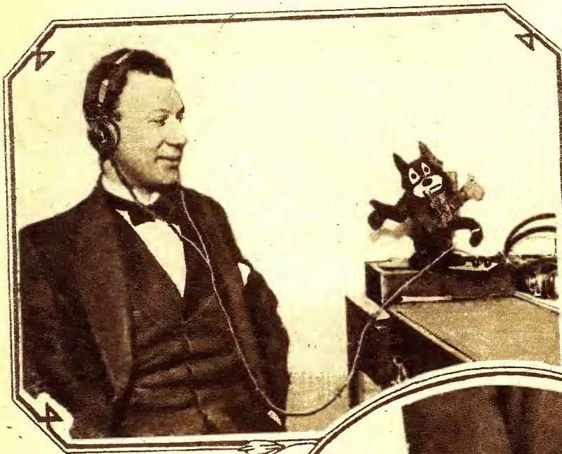
Above: A new feature in radio sets is this one of Felix, the Movie Cat. The tail forms the tuner and the solitary whisker on the face acts as the "cat whisker" for the crystal. © Keystone View Co. Right: A complete radio receiving set that fits the vest pocket. The crystal detector is mounted on the small panel containing the switch. Below: A miniature honeycomb coil tuner that operates just as well as a large one.
