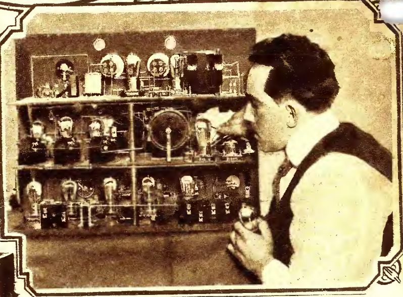
Above: This unique Super-Heterodyne was built by Henry Brinkman of Pelham, N. Y. The top shelf contains a two stage tuned radio frequency amplifier, the second shelf the detector, oscillator and intermediate radio frequency amplifiers, and the third shelf the second detector and three stages of audio frequency amplification, the third being push-pull. © Kadel & Herbert. Left: John Shepherd, 3rd a prominent merchant of Boston owns this six tube portable radio set. It is composed of three stages of radio frequency amplification, a detector and two stages of audio frequency amplification. © International Newsreel.
