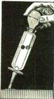
Small, fits easily under tables, or into Battery compartment of set. No figures to see—you do not have to withdraw Hydrometer from the battery to read. Saves all chances of spilling acid. The patented balls tell the story. Swim all THREE, charged fully. Sinks the WHITE, charge still right. Sinks the GREEN, charge is lean. Sinks the RED, charge is dead. Chaslyn Balls standard equipment with leading battery manufacturers on glass cased batteries.
