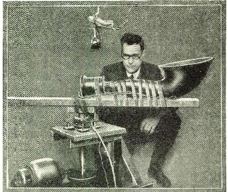
The source of the sound is a loud speaking horn, which is secured on a revolving arm. This is operated by a one-half horsepower electric motor; by rotating the source
