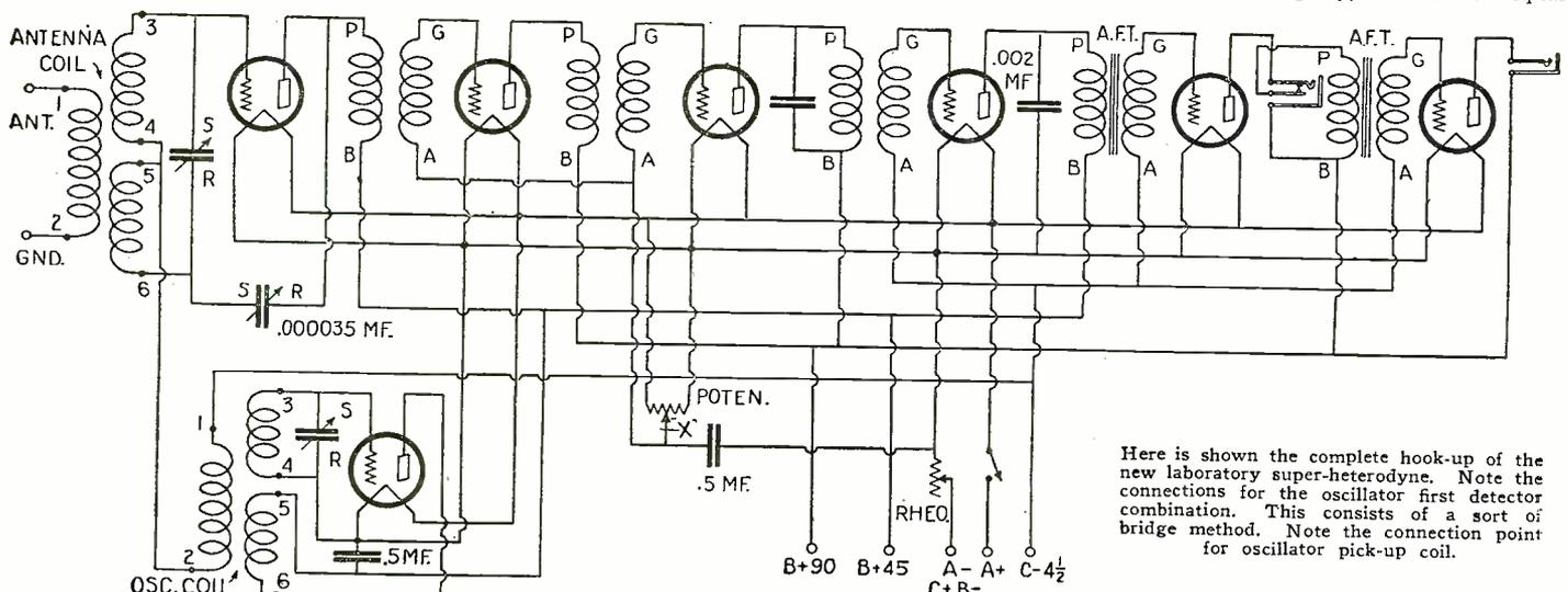
Here is shown the complete hook-up of the new laboratory super-heterodyne. Note the connections for the oscillator first detector combination. This consists of a sort of bridge method. Note the connection point for oscillator pick-up coil.
