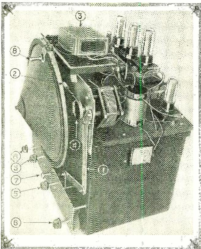
The apparatus removed from the cabinet. At 1 is shown the system of levers for compensating the capacity of the coils; 2 is the connecting cable of piano wire; 3, "C" battery; 4, pulley; 5, compensator controls; 6, rheostats; 7, filament lock switch; 8, tuning control lever.
