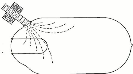
The invention consists in the process of exhausting the bulb of a thermionic valve or the like, the employment of a magnetic field to prevent damage to the glass of the bulb.
