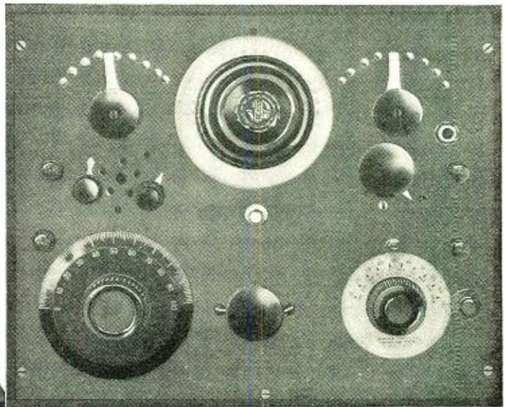
Above is shown a front and back panel view of the home-made set which has heard almost every broadcaster in the United States. Note that no sacrifice of efficiency is made for the sake of simplification of control. All tuning devices have vernier arrangements.
