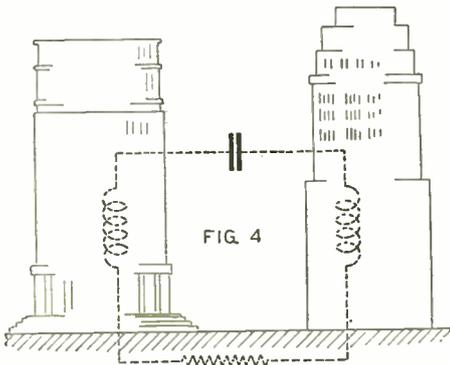
The steel framework, metal pipes, etc., in and between tall buildings may form an oscillating system as shown in this illustration.
