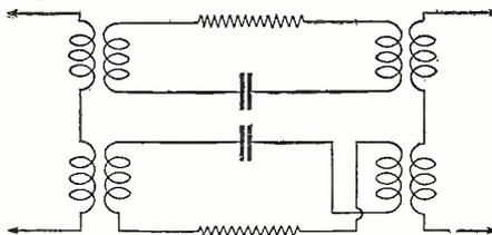
The invention consists in the combination with primary and final oscillatory circuits of two intermediate oscillatory circuits through each of which
