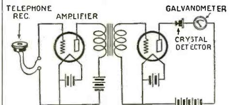
The circuit diagram of the apparatus used in testing building materials.
