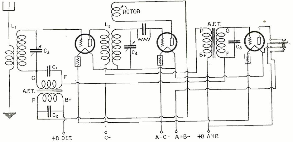
Schematic diagram of the receiver. Automatic current filament control and a filament control jack are two features that aid in simplicity of tuning.
