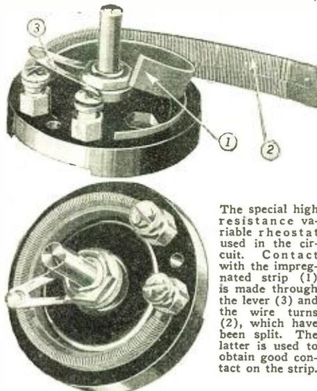
The special high resistance variable rheostat used in the circuit. Contact with the impregnated strip (1) is made through the lever (3) and the wire turns (2), which have been split. The latter is used to obtain good contact on the strip.
