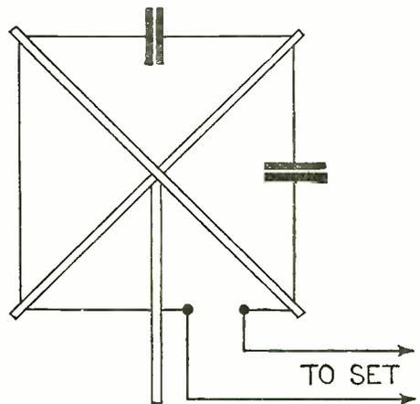
First loop antenna to be used in radio was designed by DeForest. Above is a diagram of it. Note the condensers.
