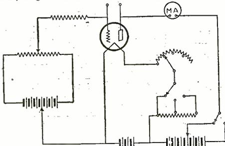
cuit, a testing instrument in one of said circuits and a resistance unit in one of the circuits for protecting the testing instrument should the grid and plate of the electron tube be short-circuited.
