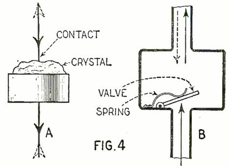
A crystal detector is really a valve and an analogy is given above.
