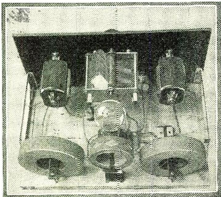
Back view of the laboratory model. Notice that the fields of both stators and rotors of the variometers are always at zero coupling with the fields of the two large coils.
