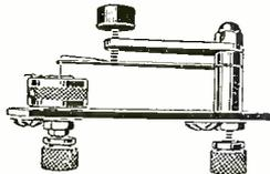
Street, Medford, Mass. It is designed for panel mounting. A very fine, accurate adjustment of a crystal contact can be obtained with this detector.
