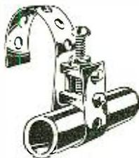
method of obtaining a good permanent ground on water pipes, etc.
