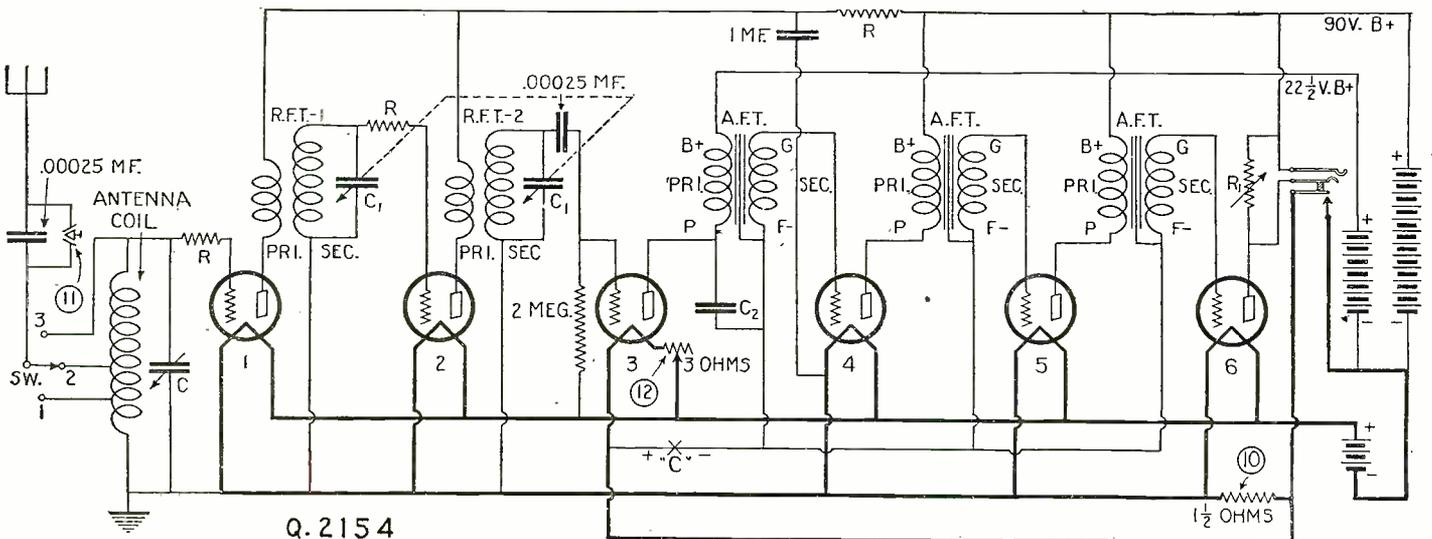
Schematic diagram of connection system employed in Universal Plio-6, a receiver designed to cover a wave-length range of 35 to 3,500 meters, by use of the well-known plug-in coil principle. Plugging the loud speaker plug into its jack puts the set into operation automatically, as a "filament control" jack is used.
