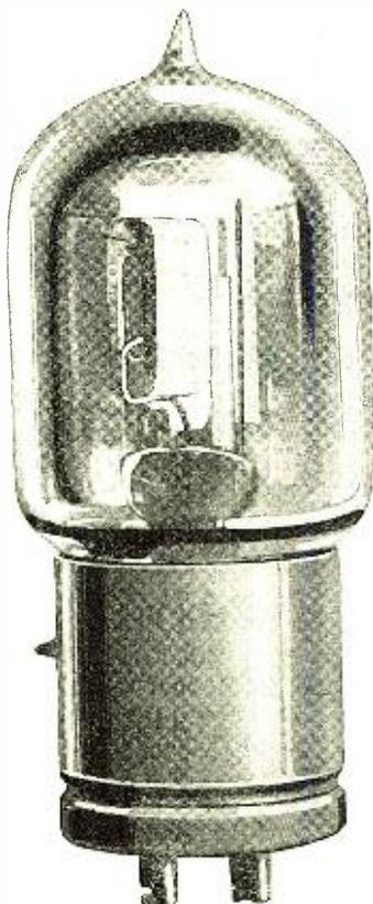
Note that in this new tube the position of the elements is horizontal, at an angle of 90° from the usual method of mounting.
