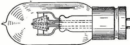
The invention consists of a mount for an electron device comprising a looped filament, a grid having a plurality of rounded portions concentrically disposed about the filament and a plate having a plurality of rounded portions disposed about said grid.
