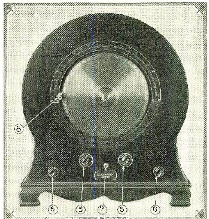
The cone loud speaker is part of the front of this receiver. The numbers correspond to those shown on the left. Stations can be logged by recording the numbers on the scale indicated by tuning control, 8. Photos courtesy of the R. E. Thompson Mfg. Co.
