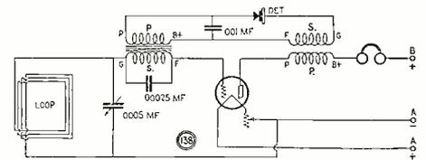
Many experimenters claim that the reflex here shown gives a greater output of undistorted signal than any other single-control one-tube set.
