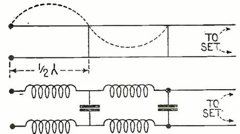
Back in the early days, about 1906, Dr. DeForest in experimenting with short waves, ran into the design of filters. Above is the Lecher wires and below the later filter design deduced from it.
