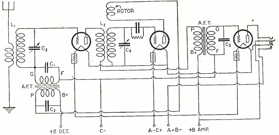
Schematic diagram of the receiver. Automatic current filament control and a filament control jack are two features that aid in simplicity of tuning.
