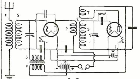
The Harkness Reflex circuit, shown above, uses the Rice method of neutralization to prevent oscillations in the R.F. amplifier.
