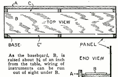
unnecessary long leads. The transformers, sockets and other instruments may be fastened to the baseboard by small nuts and bolts.
