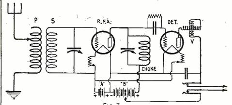
This circuit is better than that shown in Fig. 2 as the plate impedance of the amplifier tube can be tuned.
