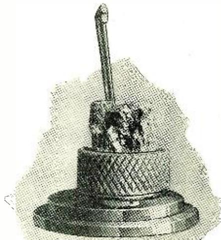
An ordinary piece of crystal, such as that used in a crystal detector for radio work, is shown in the above photograph.
