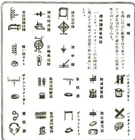
Here are the Chinese words for the apparatus shown at the side. The manner of reading is to start at upper right side and read vertically. Courtesy of La Sinda Radio.
