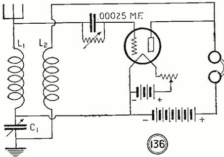
In the circuit shown above, no control of the coupling between coils L1 and L2 is needed. The condenser C1 simultaneously controls both tuning and regeneration.
