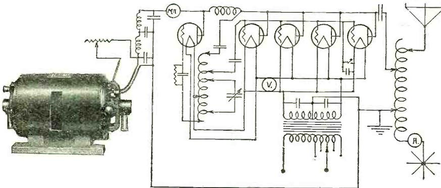
Item No. 8 Type M. G. 113 500 volts 150 watts when used with one five watter as a master oscillator and four as amplifiers, will make a set of which the owner may be justly proud. A real DX getter.
