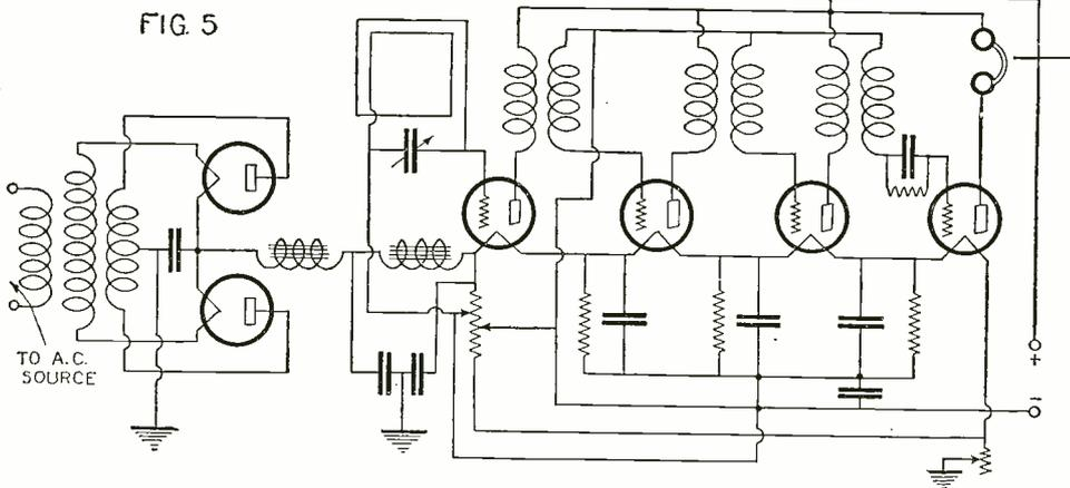
This circuit illustrates a receiver and "A" eliminator combined. Condenser values are 2 mfd. each.
