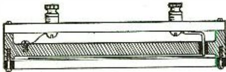
period of vibration so low as to be below audibility and supported in such a way as to receive vibrations from an acoustic source, a fluid-tight chamber beneath the diaphragm and electrostatic means for converting the acoustic energy into electrical energy.
