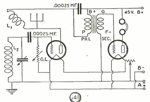
A popular British hook-up in which increased selectivity is obtained by coupling the antenna circuit through the tickler coil.
