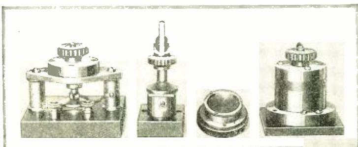
One of the most important parts of the crystal-controlled oscillator is the crystal holder. At left are shown four types developed by the General Electric Co. The two at the left are for experimental work while the others are commercial types.
