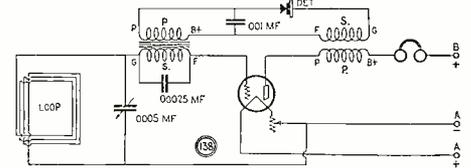
Many experimenters claim that the reflex here shown gives a greater output of undistorted signal than any other single-control one-tube set.
