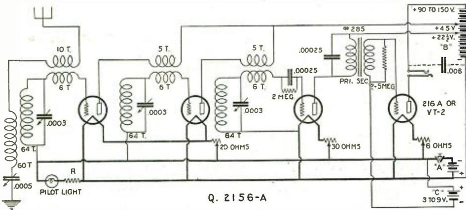
The Garrison circuit. An unusual arrangement of coils with the object in view of preventing circuit oscillation, and at the same time retaining selectivity and a negative grid bias of the radio frequency tube grids.
