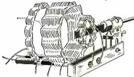
An excellent method of mounting a three-circuit tuner is shown above, there being a minimum of insulation in the apparatus.
