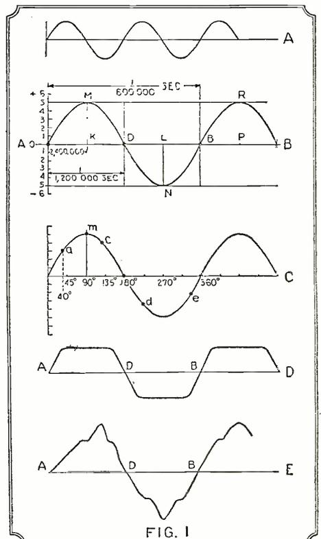
Various kinds of curves used in radio, showing voltage or current against time.
