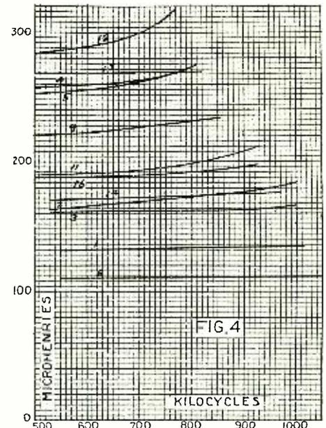
The curvature of the graphs indicate the presence of distributed capacity in the coils.
