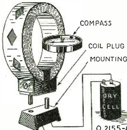
A simple and efficient method for determining whether honeycomb coils are correctly "poled."
