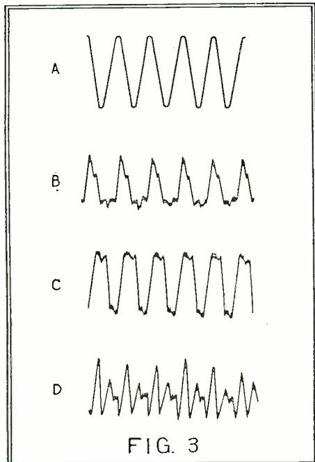
Oscillograms of the original pure sine wave as transmitted, and various forms of distortion that occurred before reception.
