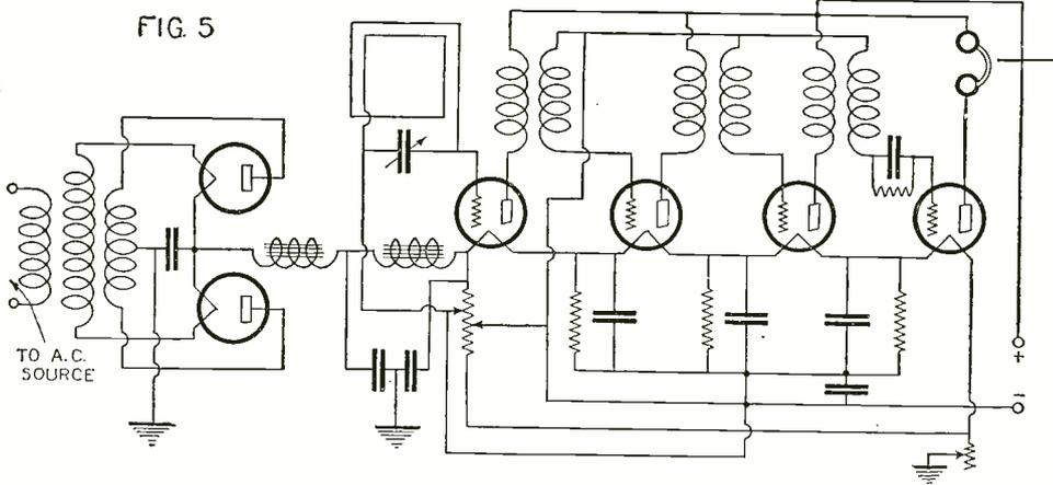
This circuit illustrates a receiver and "A" eliminator combined. Condenser values are 2 mfd. each.
