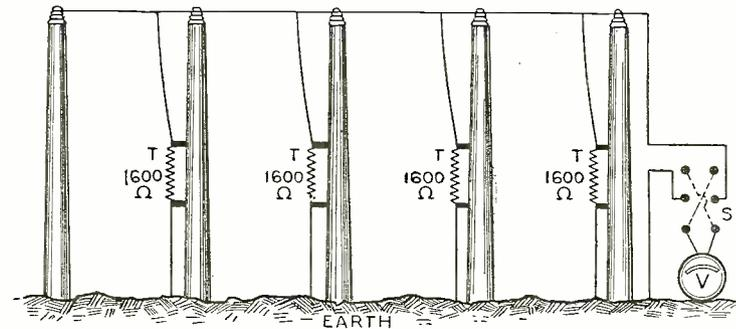
Fig. 2. The circuit that was used in the tests. It was found that the voltage indicated by the voltmeter, V, rose and fell to 28 volts following the behavior of alternating current. The reversing switch, S, was used only to get a reading on the meter.
