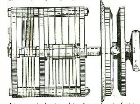
plates, a set of rotor plates for each set of stator plates, means for independently rotating the rotor plates and means for simultaneously rotating the rotor plates.
