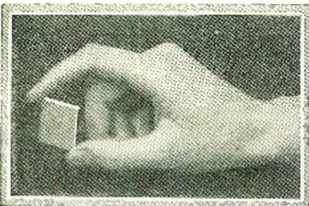
Some idea of the size of the crystals used in broadcast work may be obtained from the photo above. Note the small crack in the crystal being held. Refer to opposite page.
