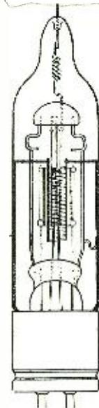
Fig. 5: Sketch of Dr. Hull's new tube, showing method of shielding the control grid from the plate.
