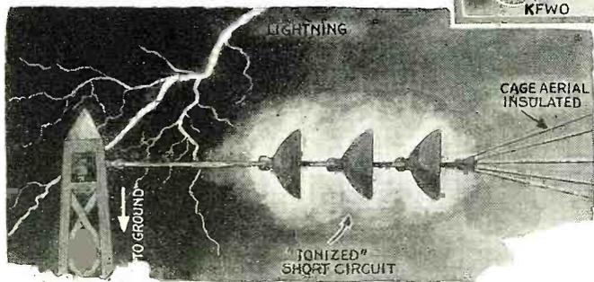
Lightning can interfere with a radio program, not only as static, but also as a short circuit, as shown by a recent experience at the great Bound Brook, N. J., station, WJZ. The aerial is insulated from its supporting towers; but the lightning playing around the latter "ionizes" the air, making it conductive; and the result is a momentary short-circuit to ground, like the closing of a switch, shutting off the transmission until the effect ceases.
