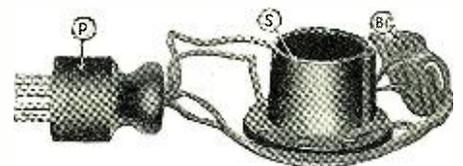
P, plug which fits in the final A.F. socket in the set; S, socket for power tube; BC, wires for additional batteries.
