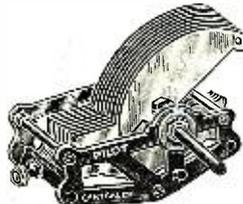
Company, Inc., 323 Berry Street, Brooklyn, New York, is of the low-loss, one-hole-mounting type. This seventeen-plate condenser has a minimum capacity of 12 mmf. The plates are so shaped that a very even distribution of the broadcast stations along the dial periphery is obtained. This instrument is neatly and efficiently built.
