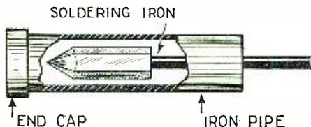
If you place your soldering tool in an iron pipe like the above, scale will not form on the iron as when heated in an open fire.
