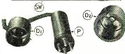
Back view of the meter panel: M, meter; SW, changeover switch; R, protective resistor. Below: P, plug; D1, D2, adapters.
