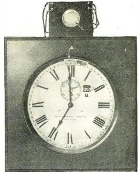
Above, the face of the Time Chime just before the signal; the minute hand has closed a switch, A, as shown in the diagram below. Twelve seconds before the signal, the second hand closes another and the pilot lamp, L, lights. The announcement is then made to the radio audience, and the Western Union signal strikes the chime, which goes out through WRNY's transmitter.
