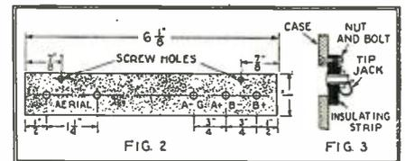
Fig. 2 shows the bakelite strip in which the tip jacks, shown in detail in Fig. 3, are installed.
