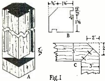
Details are shown above for the construction of the legs of the cabinet, if a lathe is not available.
