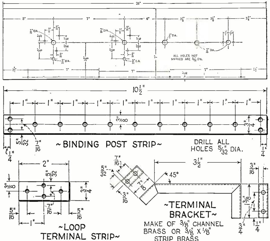
Top—Drilling layout for the front panel. Mark out all the holes with a hard, sharp pencil, and then make dents in the panel with a center punch wherever a hole is to be made. Do not attempt to drill without first doing this. Center—Layout of the long binding-post strip. Bottom—Details of the loop terminal strip and the supporting brackets; three of the latter are required.
