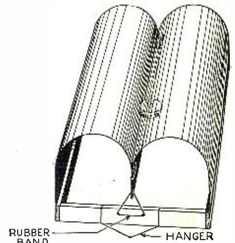
Fig. 2-B. The completed loud speaker, arranged for use on the wall, as viewed from the top. The position of the unit is indicated.
