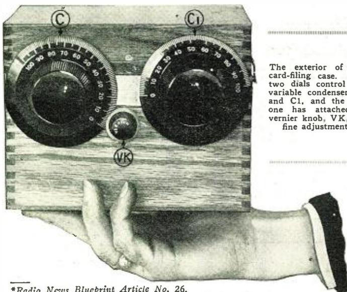
The exterior of the card-filing case. The two dials control the variable condensers, C and C1, and the left one has attached a vernier knob, VK, for fine adjustment.
