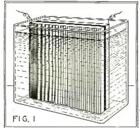
Two metallic plates, separated by an insulator, and immersed in a metallic-salt solution, will assume light-sensitive properties in about a week.
