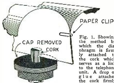
Fig. 1. Showing the method by which the diaphragm is firmly attached to the cork which serves as a link to the telephone unit. A drop of glue attaches the cork firmly to the diaphragm, while its weight has little damping effect.
