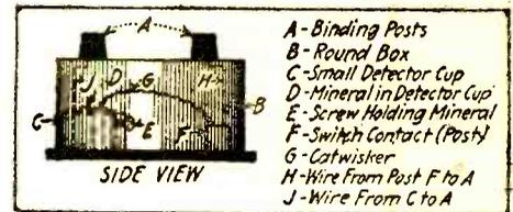
A detector of this type requires no adjustment, as the contact point and crystal are enclosed in sealing wax.
