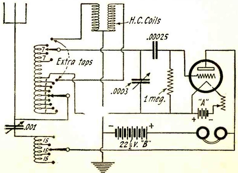
The addition of two honeycomb coils in the Reinartz circuit, as shown, permits the covering of high wavelengths.
