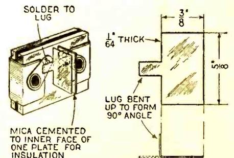
An auxiliary condenser useful for equalizing capacities.
