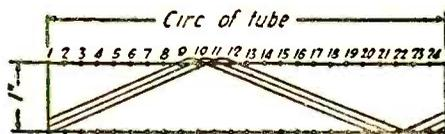
By this system of winding unit honeycomb coils the appearance of the commercial product may be duplicated.
