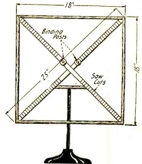
Good results will be obtained at short distances with this loop, using one or more tubes.
