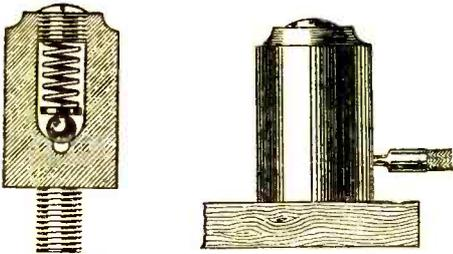
A quick-change binding post may be easily made, as shown above.
