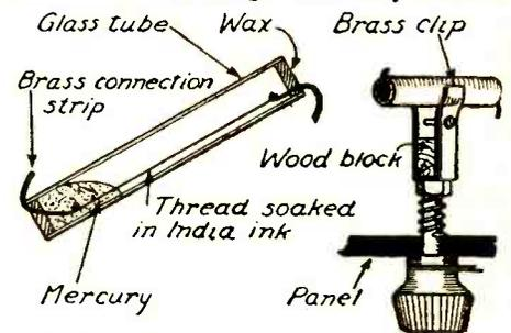
Details of a mercury variable grid leak.
