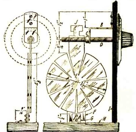
Details of the spider-web coil mounting. The coil forms can be made of any good insulating material.
