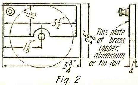
Dimensions and details of the stationary plate and its mounting.
