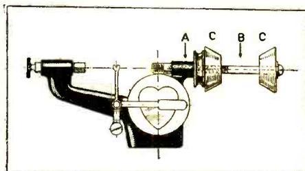
Sewing machine bobbin coil winder.
