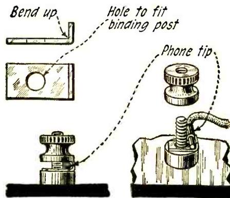
For loose binding post connections.
