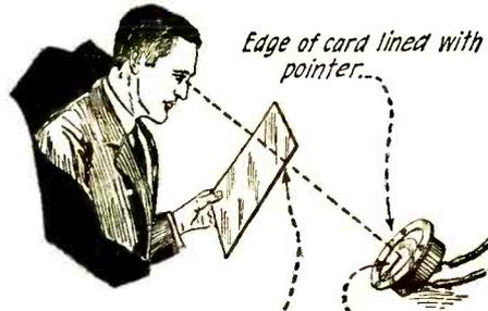
Reading sighted and lined with card edge. A good way of reading a meter that has a broken needle.
