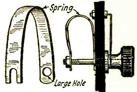
Method of mounting efficient contact switch.
