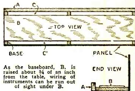
As the baseboard, B, is raised about ¼ of an inch from the table, wiring of instruments can be run out of sight under B.
