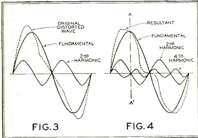
Fig. 3 illustrates the breaking down of a sine wave. Fig. 4 shows a distorted wave composed of the fundamental, 2nd and 4th harmonic frequencies
