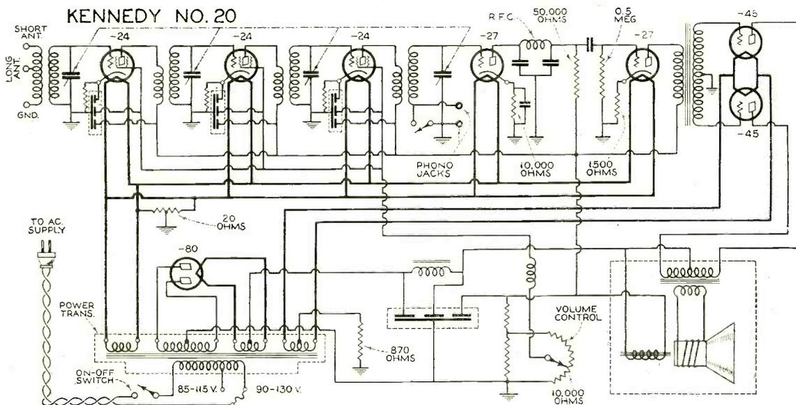
THIS receiver, the Kennedy Model 20, is of conventional design and sound engineering principle. Eight tubes are employed, three -24's in the radio frequency stages, two -27's in the detector and first audio stage, and two -45's in the power output, push-pull stage. The first audio stage is resistance coupled, the push-pull stage being transformer coupled. Volume control is accomplished by varying the screen-grid voltage on the r.f. tubes. Provision is also made
