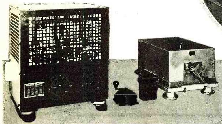
Shown above is the equipment for plane installation, which weighs but 100 pounds altogether. The receiving and transmitting equipment for the radio-telephone installation in planes is remotely controlled from the pilot's cockpit
