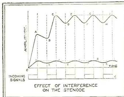
Fig. 7. Here is shown the amplitude of a signal to which the Stenode is tuned, contrasted to that of an interfering signal
