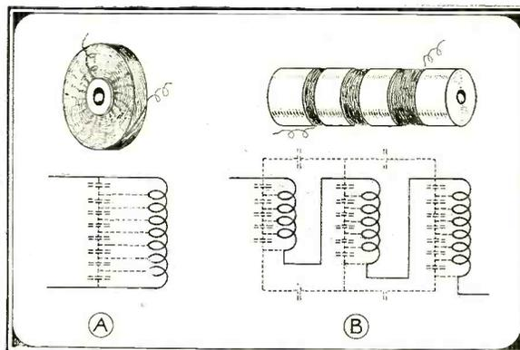
and in shunt, as will be seen, to the entire winding and to each individual turn, resulting more or less as a short circuit for the radio frequencies, and causes the formation of resonant circuits within the choke. These conditions, when of a large degree, make for a worthless choke.
