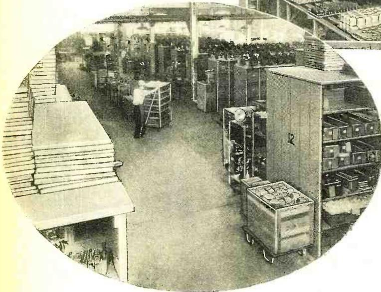
Above, the coil winding department where the enormous number of coils are made that are required daily in the construction of Silver-Marshall Superheterodyne receivers. At the left is the 12,000-foot, centrally located stock room into which all material flows and from which it is drawn as needed by the various departments. All preliminary inspections of raw materials are also made here which greatly speeds up operations in manufacturing departments
