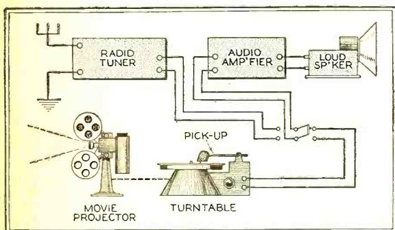
In this diagram is depicted the various units which go to make up a satisfactory home talking movie outfit. By means of a double-pole double throw switch the audio amplifier of the regular radio installation may be thrown over from radio reception to the phonograph pick-up on the turntable which is mechanically geared, by means of a flexible cable, to the movie projector
