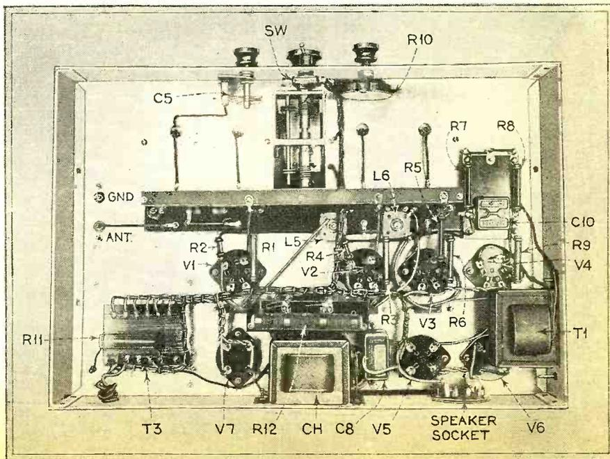
mounted in position to the right of the tuning knob, the midget trimming condenser, C5, to the left. The switch, SW, is mounted in the hole directly beneath the tuning knob. The four-gang tuning condenser is then mounted, followed by the mounting of the power transformer, T3, and the large electrolytic condenser, C11, for the "B" unit.
