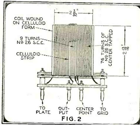
the center and this center-tap connects to the rotor section of the variable tuning condenser. In order to make the shaft of the tuning condenser "cold" a double condenser is used so that the mid-point may be at ground potential. The plate circuit of the oscillator tube is shunt fed through an r.f. choke.
