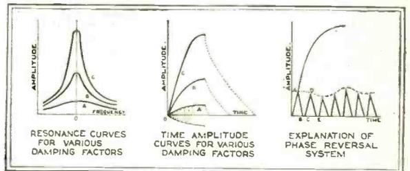
Thus for the signals K we find that the receiver continues to build up according to the curve OABCD, finally reaching a steady state with the amplitude varying according to the signals.
