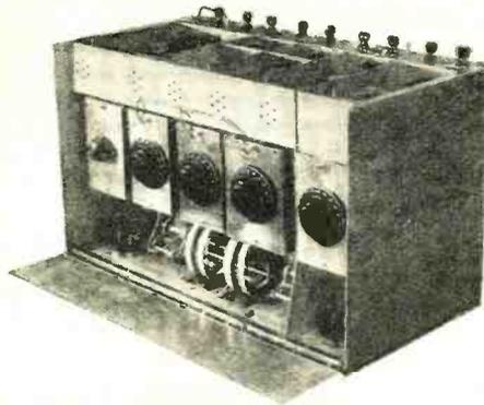
The tuner section of the Stenode lying on its face and showing the tuned intermediate stages
