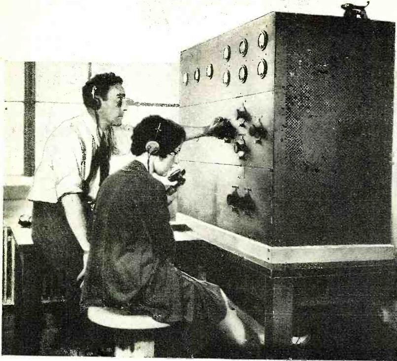
Tuning the transmitter at one of the twenty-two ground stations of the Boeing System. The young lady seated at the radiophone apparatus is talking with a pilot flying a Boeing mail-passenger plane 14,000 feet above sea level and 152 miles distant
