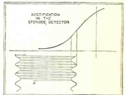
Note how rectification is obtained in the Stenode by utilizing only that portion of the r.f. excursions which constitute the variation in amplitude
