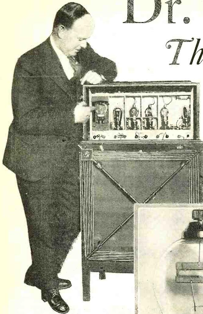
Above—Dr. Robinson is pointing to the "Quartz Crystal" tube, which is located in the last stage of intermediate-frequency amplification of a regular broadcast superheterodyne. Note the loop attached to the back of the cabinet, for signal pick-up. Below, to the right, is a close-up view of the quartz crystal mounted within an evacuated tube. This crystal is ground to resonate at a frequency of about 100 kc., corresponding to the frequency of the intermediate amplifier
