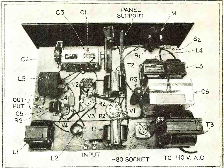
This view shows the arrangement of the apparatus on the baseboard. All of the parts have been lettered to correspond to the circuit diagram and the list of parts. This view shows the placement of the parts so clearly that the constructor should have little difficulty in laying out the apparatus
