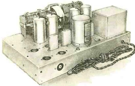
The top view of the receiver shows the shielded inductances placed immediately back of their respective tuning condensers. The corresponding tube sockets are placed as shown to enable short high potential leads in wiring
