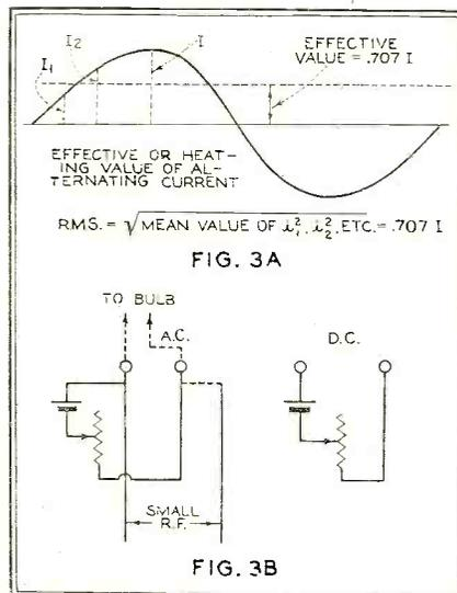
circuit the milliammeter then reads the desired effective value of a.c. In a laboratory test the home-made comparison meter was connected in series with a standard a.c. milliammeter, a resistance and 60-cycle supply. When the standard meter read 150 mils the comparison meter gave 140 mils (accuracy  $\pm 7$  per cent.) and with the standard at 250 mils the bulb instrument gave 240 mils (accuracy  $\pm 4$  per cent.)—results surprisingly good for such visual estimation.
