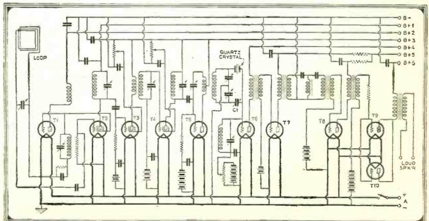
For practical purposes a superheterodyne circuit is employed in the Stenode, since then only one crystal need be employed (in the i.f. amplifier), as shown in the circuit above
