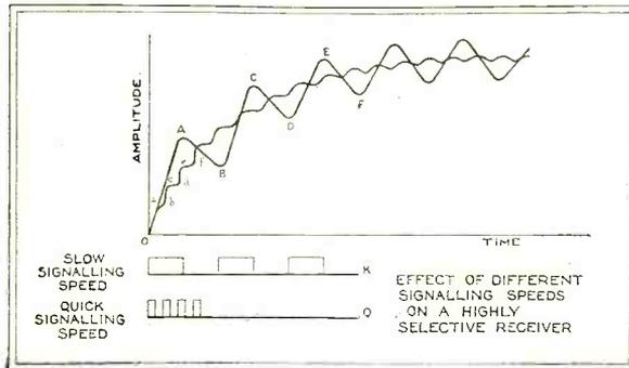
Fig. 3. In a circuit such as that wherein a quartz crystal is employed, thus having low damping, the effect of various signalling speeds or audio-frequency modulation produces an effect as shown above
