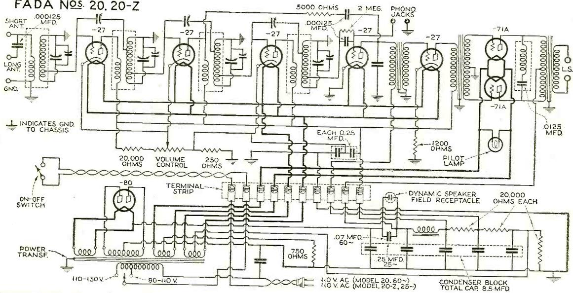
THE Fada 20 and 20-Z are alike except that in the 20-Z a power transformer is used that is satisfactory for 25-cycle lines. The receiver is of the neutrodyne type, utilizing five type -27 tubes in the three radio-frequency stages, detector, and first audio stage. Push-pull type -71A tubes are used in the output stage. An -80 tube is used as a rectifier. Provision is made to excite the field of the dynamic
