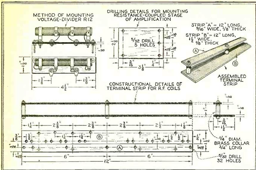
The method of mounting the voltage divider, resistor coupler and the tuning inductances in units simplifies the construction
