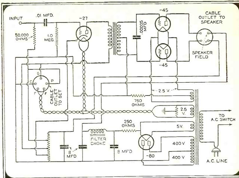
Fig. 1. The circuit diagram of the universal amplifier-speaker unit for radio, phonograph and home movies
