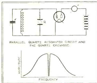
Fig. 4, above, shows a quartz crystal shunted across a tuning circuit, the resultant resonance curve being that shown in the lower part of the figure. Fig. 5, to the left. In order to utilize the crevasse of the crystal resonance curve a series resonance circuit is arranged as shown above. The lower tuning capacity is employed to balance out the capacity of the crystal holder
