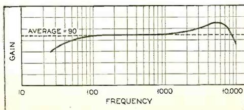
Fig. 2. The over-all frequency characteristics of the amplifier-speaker combination
