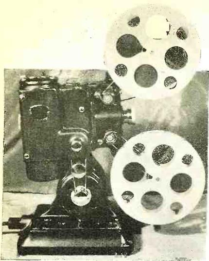
(Left) The Ampro projector, to which by means of a flexible cable it is possible to couple a turntable for home talkie use
