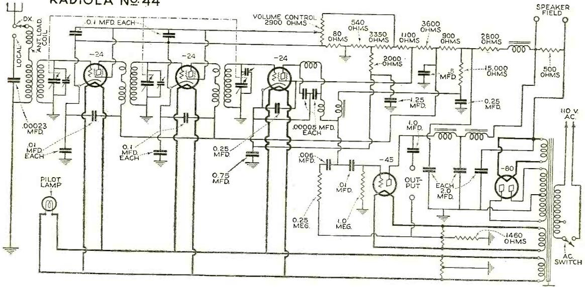
THE Radiola 44 is a four-tube receiver of quite unusual characteristics. Two stages of radio frequency amplification are used, employing type -24 tubes. The coupling between these tubes consists of a radio-frequency transformer whose primary is wound with one turn of wire very closely coupled to the grid end of the secondary, and the remainder of the primary is wound at the low potential end of the secondary. This gives both capacity and inductive coupling
