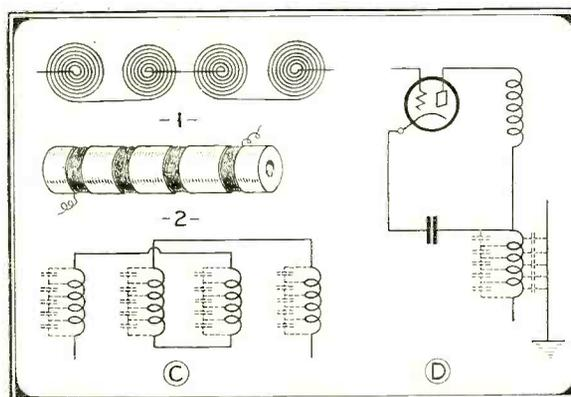
The removal of such metallic cores has in many cases overcome circuit oscillation and instability. It is preferable to cement the choke to a dowel, then using a small brass wood screw for fastening the assembly to the chassis or shielding. If possible, each choke should be placed in individual shielded compartments, with at least one inch of space on all sides.
