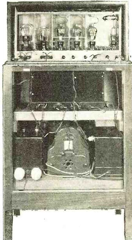
A rear view of the Stenode. At the top is the receiver chassis of the superheterodyne, while below are the audio channel and loud speaker-power supply units
