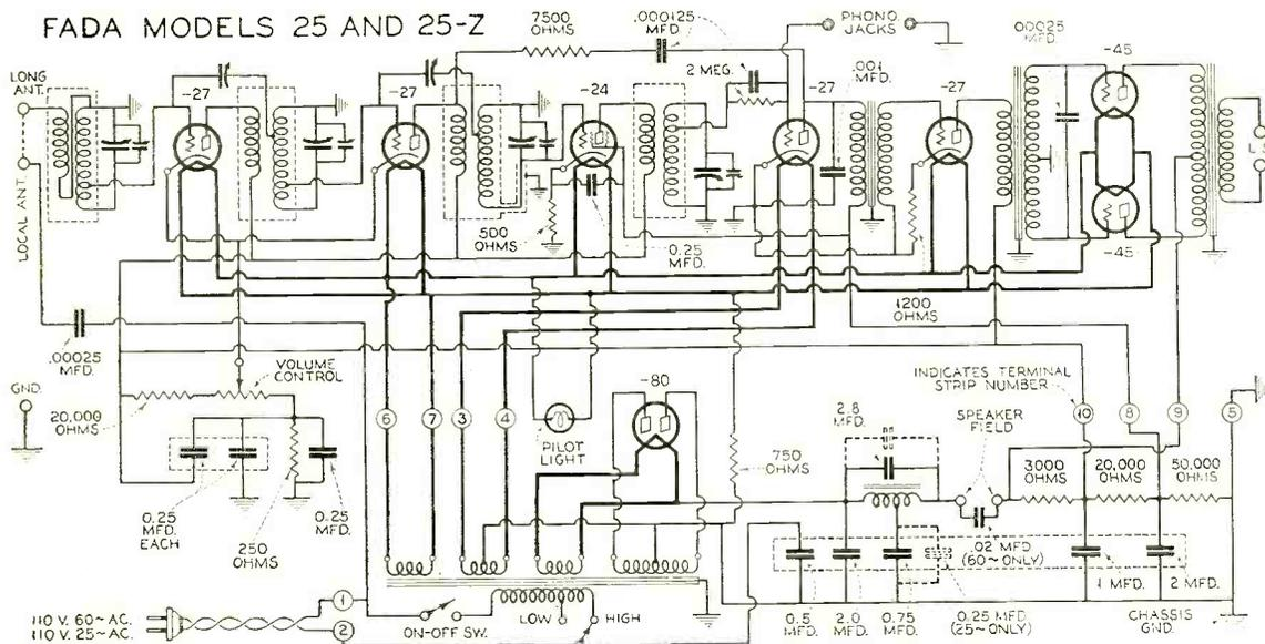
THE Fada Model 25 and 25-Z is an eight-tube receiver, utilizing two -27 type tubes, and one -24 type in the radio frequency stages, a -27 tube in the detector, and first audio stages, and two -45 type tubes in the power output stage, in a push-pull arrangement. An -80 type tube is used in the power supply. A neutrodyne circuit is employed in the radio frequency amplifier to insure stability, while a small amount of regeneration is employed to increase the gain, and selec-
