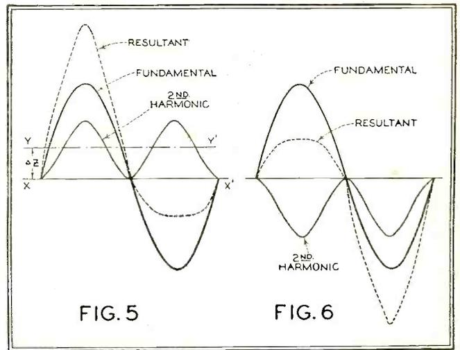
Fig. 5 illustrates the presence of a strong 2nd harmonic with the fundamental. Fig. 6 illustrates the presence of a strong 2nd harmonic, but 180° out of phase in comparison to Fig. 5
