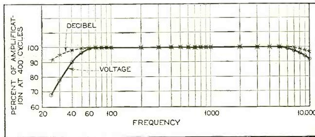
Fig. 3, to the left, shows a practical flat response from 60 to 5,000 cycles, with only a slight falling off at 10,000 cycles
