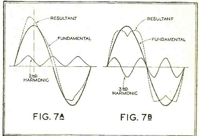
even though we speak of a distorted wave as containing harmonics, that these harmonics exist as separate waves distinct from the distorted wave, but rather the reaction of the distorted wave upon the circuit is exactly the same as if the distorted wave were replaced by a fundamental frequency and associated harmonics.
