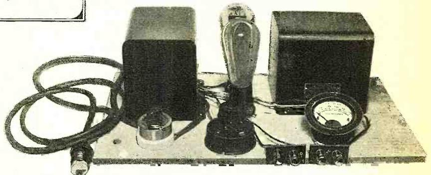
your oscillator tubes. You can buy a transformer with filament windings wound right on it for the rectifier tubes and also for your oscillator filaments. This makes a very convenient layout and also reduces the expense somewhat; always a desirable feature.
