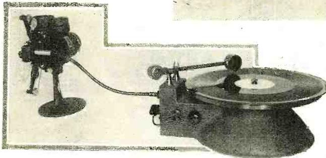
The Hollywood Film Enterprise turntable and pick-up, especially designed for use in conjunction with home movie projectors for synchronization of sound. The gear mechanism of the turntable is mounted in the base, together with speed and volume controls. Synchronization between projector and turntable is obtained by the flexible shaft shown
