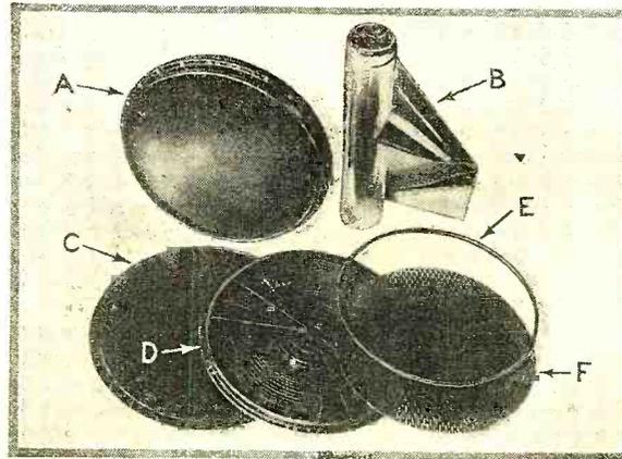
A, the assembled oscilloplane; B, a roll of the diaphragm material; C and D, stationary electrodes moulded in ribbed bakelite; E, holding ring; F, cover plate
