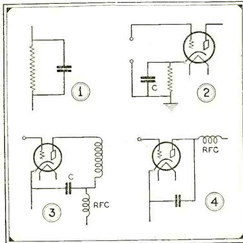
reactance formula, we get C equals .003 mfd. Allowing further losses introduced by circuit wiring and the arrangement of the parts, and to bring the value to a more convenient commercial size, the minimum value is selected as .006 mfd. Actual experience has shown that values up to and including 1 mfd. promote greater circuit stability and sensitiveness. Wherever possible such values should be used.
