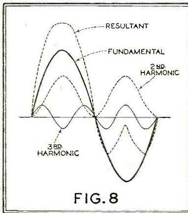
Fig. 8. The resultant wave obtained by a combination of a fundamental, a third and a second harmonic
