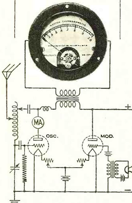
Here is the meter that transmitting amateurs have long needed for assuring maximum efficiency from their equipment. It is a dependable means for measuring directly the percentage of modulation.
