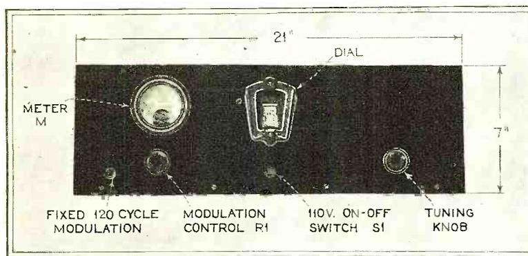
The panel arrangement is simple and neat. The various controls are indicated to correspond to the lettering of the circuit diagram
