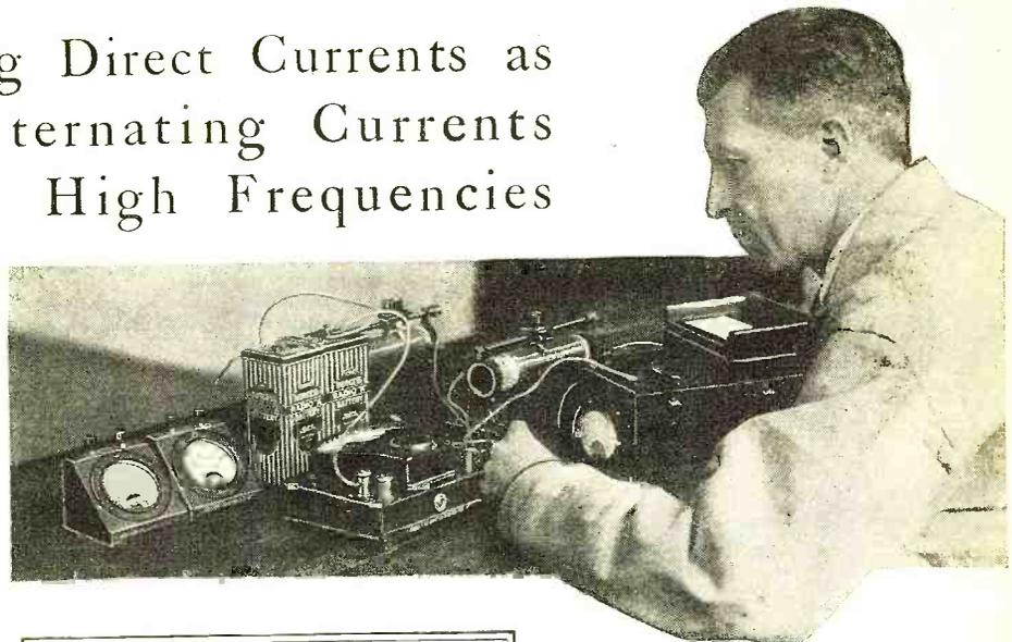
At work in the laboratory checking the comparison meter described here against costly standard instruments
