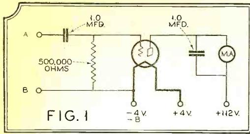
Fig. 1. The simple vacuum tube voltmeter circuit, suitable for hum measurement and similar work. Fig. 2. The circuit employed for calibrating the v.t. voltmeter. This should be recalibrated occasionally
