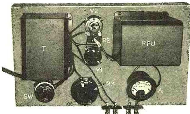
In this top view of the power supply the parts are lettered to conform with the circuit diagram given below
