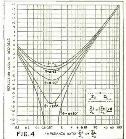
**FIG. 4. REFLECTION LOSS FOR DIFFERENT PHASE ANGLES**
