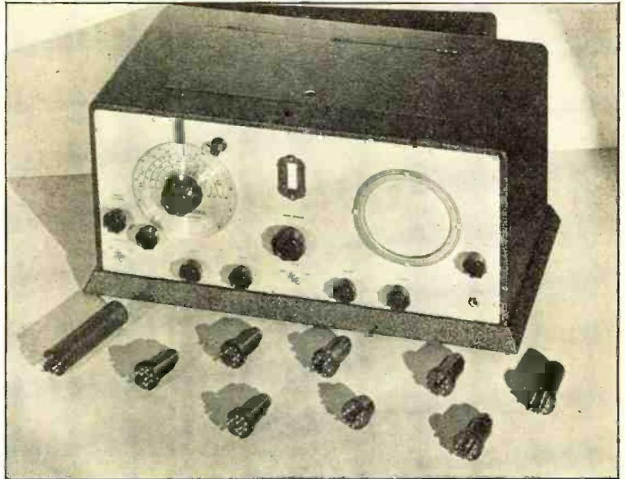
throughout as follows: a 6K7 in the r.f. pre-selector stage; 6L7 as first detector-mixer; a 6C5 as the oscillator; a 6K7 as the i.f. stage; a 6H6 as the second detector and avc tube; a 6K7 as the electron coupled beat oscillator; a 6F5 first audio, a 6F6 second audio and output tube and a 5Z4 rectifier. The 6L7 tube used here has no parallel in the glass tubes.
