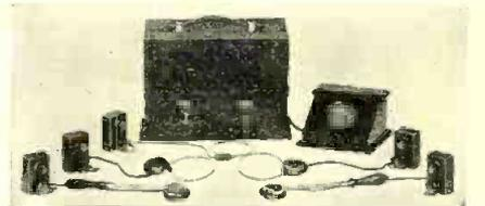
ume controls. As the microphone requires no energizing current, installation and placement of this unit is greatly facilitated.
