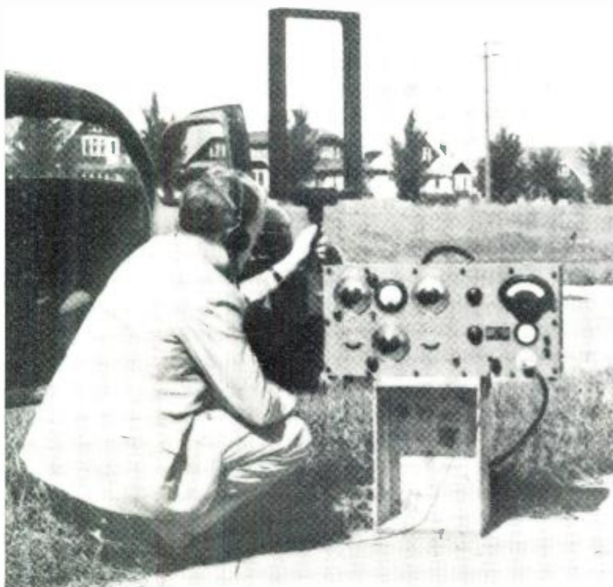
When the weather is pleasant surveys are sometimes made outside the car. The field survey meter can be dismantled and assembled outside in less than one minute.
