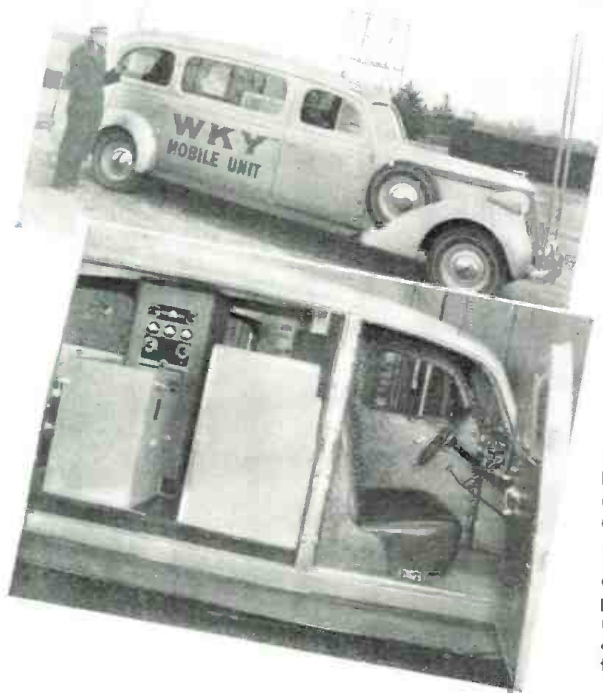
(Top) Rear view of New York mobile unit showing transmitter panel and set
