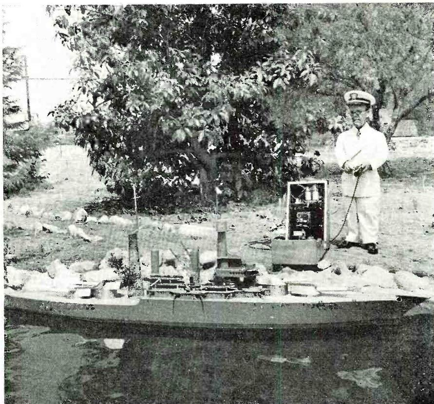
Using a telephone dial, Mr. Bixby controls the movements of his model radio navy.
