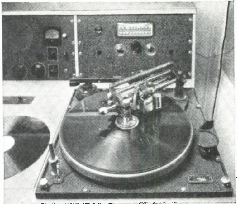
The main recording table with the cutting head in action. The playback head and arm can be seen in the back.
