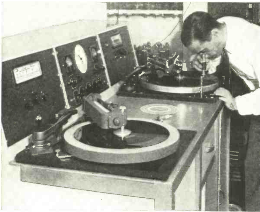
The author is using the microscope to determine the depth of the cut. This is very important if the recording is to be a good one.
