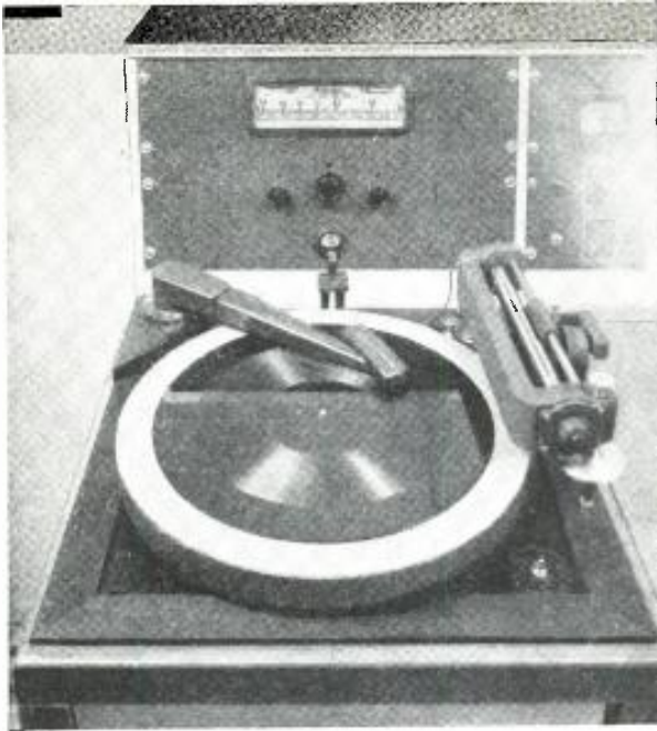
The extra playback and recording table will prove useful in "dubbing" and duplicating.
