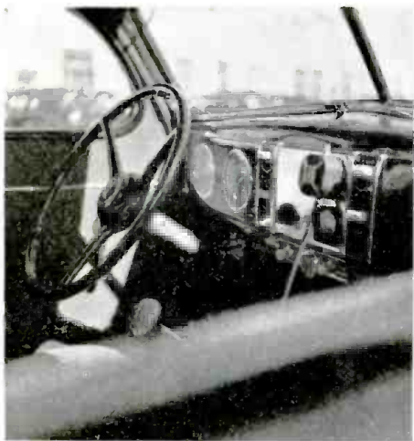
The transmitter is controlled from a small panel on the car dash-board. Push-to-talk mike mounts above meter.
