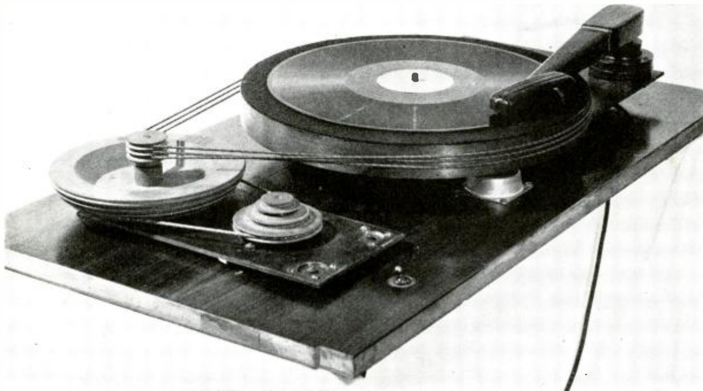
Completed turntable and drive mechanism. Note "shock-mounts" used to float the table from the motor board.
