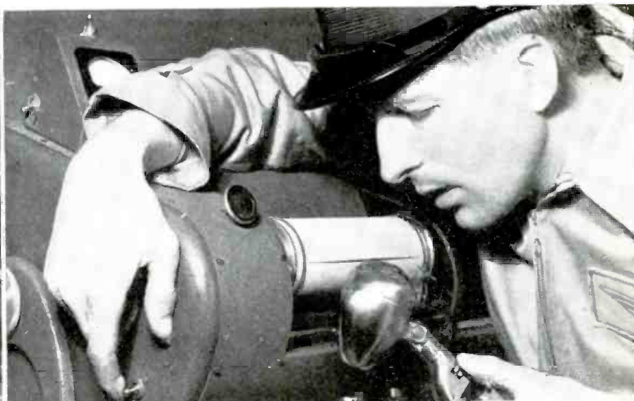
Officer in the "Blues" mobile unit gives okeh to aerial scout to start transmission of photograph from the facsimile unit in airplane via multiplexed FM radio telephony which allows him to continue giving instructions for next objective simultaneously over the same wave on which the photo is transmitted. Operator is throwing starting switch for sending.
