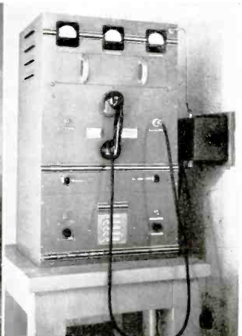
100 watt radiophone transmitter at the fixed station nerve center.
