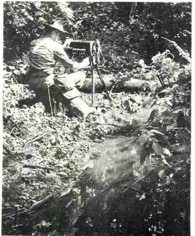
Soldier operating field telephone switchboard in heavily wooded section. Collapsible legs and compact construction make transportation simple.
