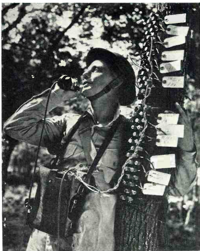
Signal Corps student operating a field telephone test station. Tags identify various lines extending to many field divisions.
