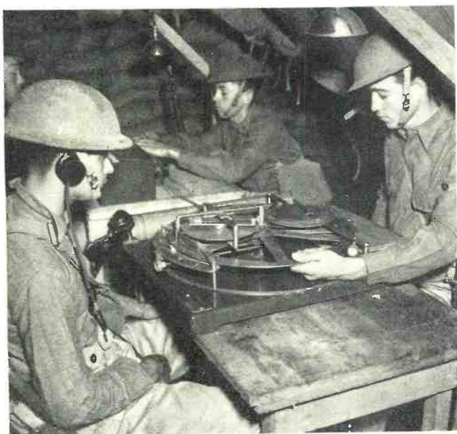
Soldiers operating a deflection board. Corrector gives range to elevation for artillery fire. Note chest-phone.
