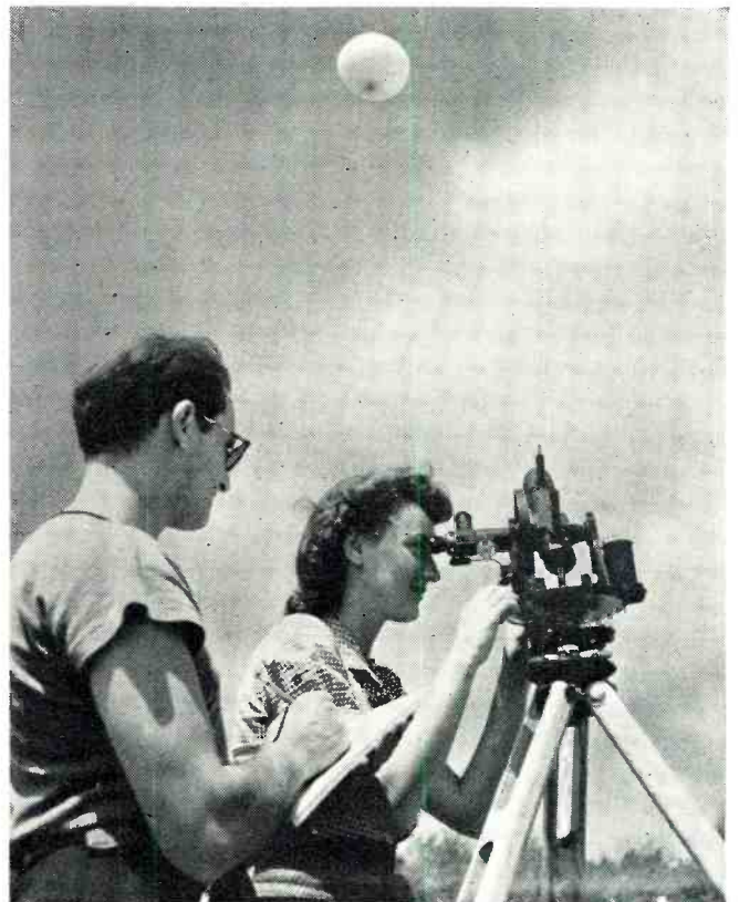
Observing the flight of a free balloon. Notes are being taken by the Laboratory worker on the left.
