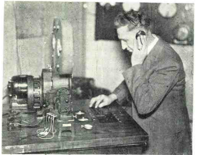
Heart of the Sound studio—the monitor booth. Operator controls volume of sound as it is photographed onto film.
