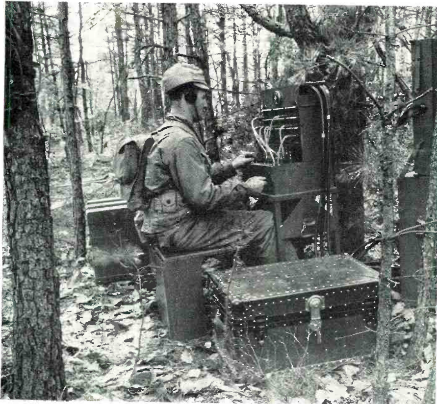
Late type field telephone switchboard. Note dial above patch cords.
