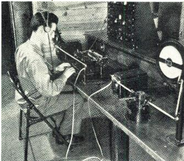
Operator reading automatic tape of high-speed radio transmission. Coordination is essential to efficiency.
