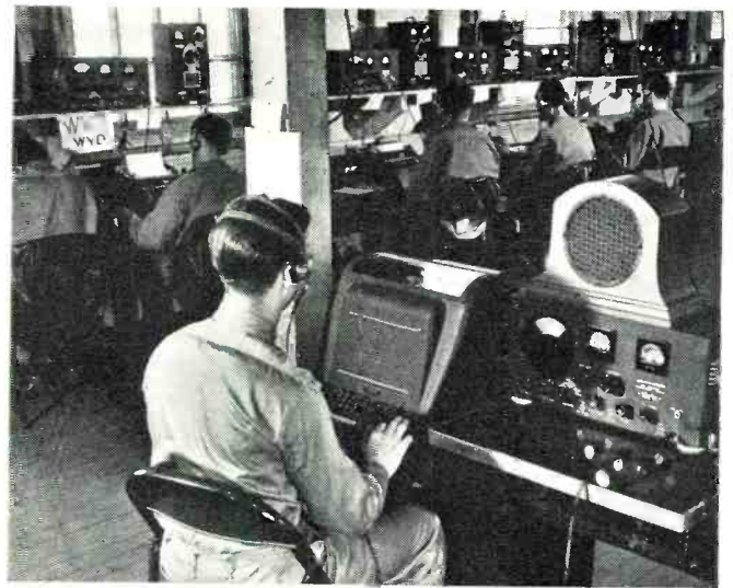
Practice networks are set up to familiarize operators with correct procedures. Note shock-mounted receiver.
