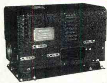
← Power Supply using rechargeable non-spill storage battery for operation of "Walkie-Talkie" radio equipment. Input Voltage, 4 Volts; Output, Numerous voltages supplying filament and plate requirements of equipment. Width, 3½"; Length, 6½"; Height, 4¾".
