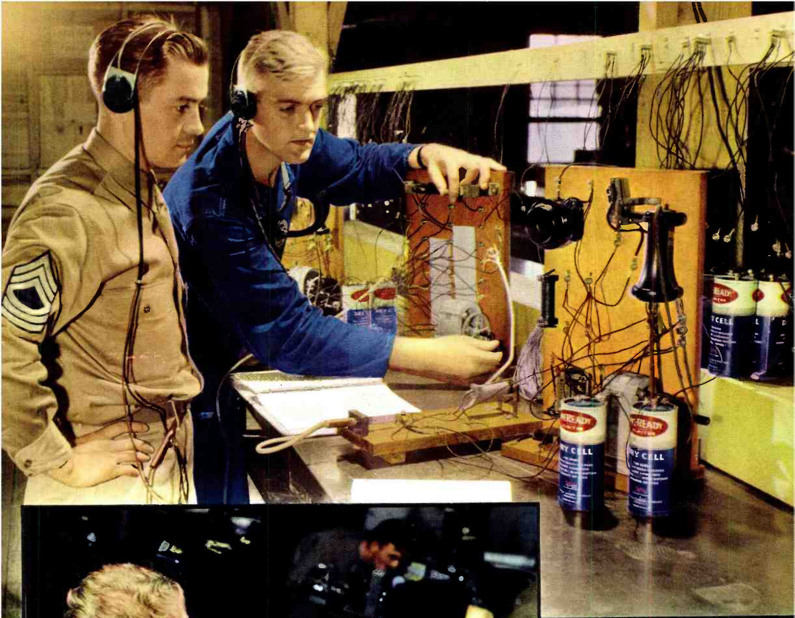
Breadboard layouts of telephone circuits facilitate the teaching of fundamentals.
