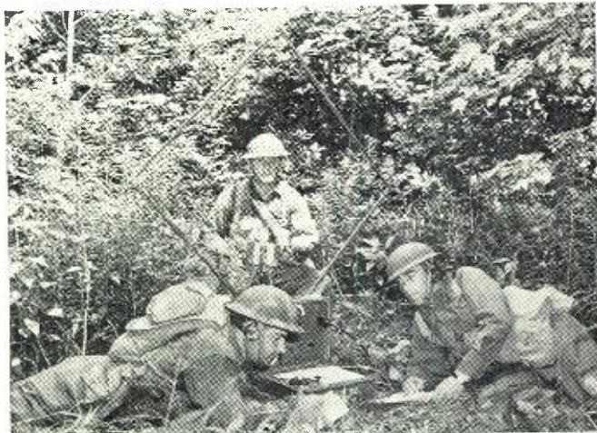
Another location for a field set. The man in the rear is operating a hand-driven generator (power source).
