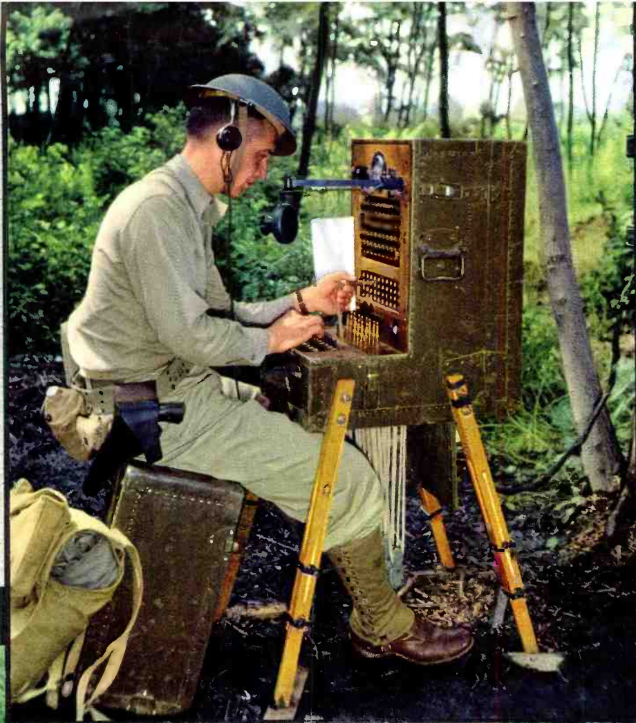
Temporary lines terminate to this portable telephone switchboard. Note collapsible legs.
