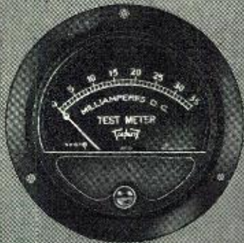
Full size of instrument. Note deep bezel for glass protection and "Quick-Look" Scale.
