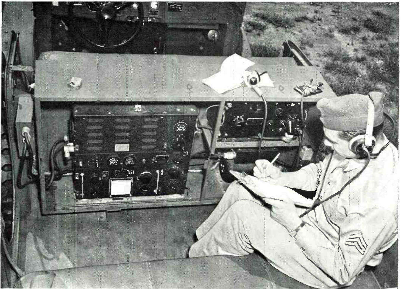
Interior of scout car. The small compartment above the receiver holds a spare set of all tubes required for the radio equipment.
