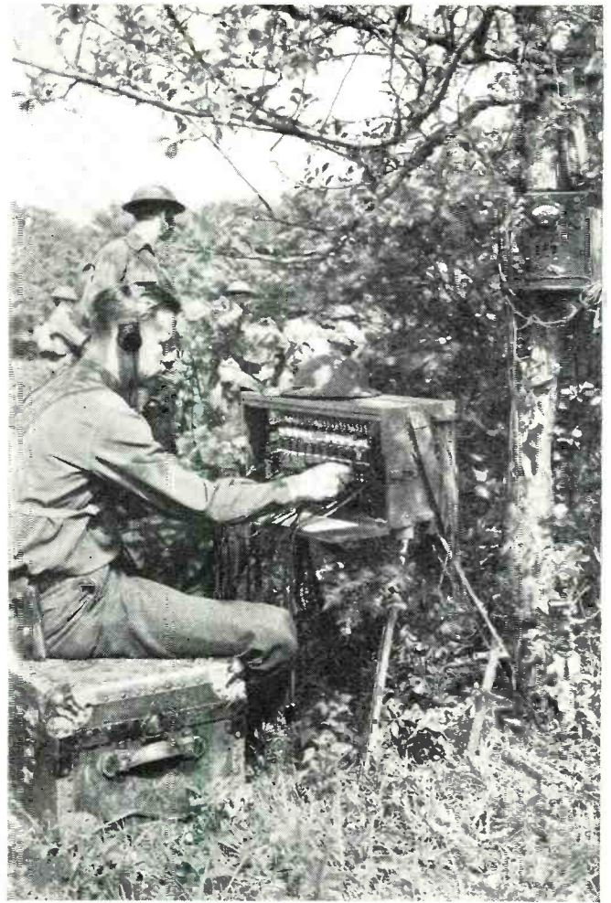
Closeup view of twelve-line field type switchboard. The instrument mounted on the tree is wire chief's testing set.
