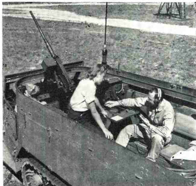
Officer inspects the installation of equipment in this armored car. Note vertical antenna support on spring mount.
