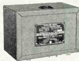
For Tank Transmitter-Receiver → Operation, Dual Input, 12 or 24 Volts; Continuous Output, 500 Volts at 200 Ma.; Intermittent Output, 500 Volts at 400 Ma.; Efficiency, 55% to 60%; Regulation, 13% on 24 Volts; 22% on 12 Volts; Output Ripple, Less than ½ of 1%; Width, 8½"; Length, 13½"; Height, 9½" (including Shock Mounting Assembly).
