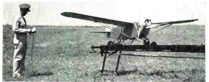
A small radio-controlled glider was developed for target purposes during the period between the two world wars.
