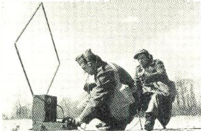
Compact, self-powered field set is operated by this two-man team. This set uses a square loop antenna.
