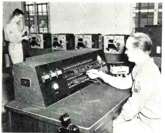
Code from the many tape machines are fed to this control panel where signals are fed to various classrooms.
