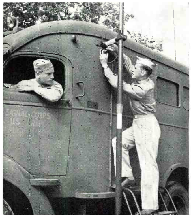
Transmitters in truck connect to vertical antenna through the bowl type insulator. Note sturdy supports.
