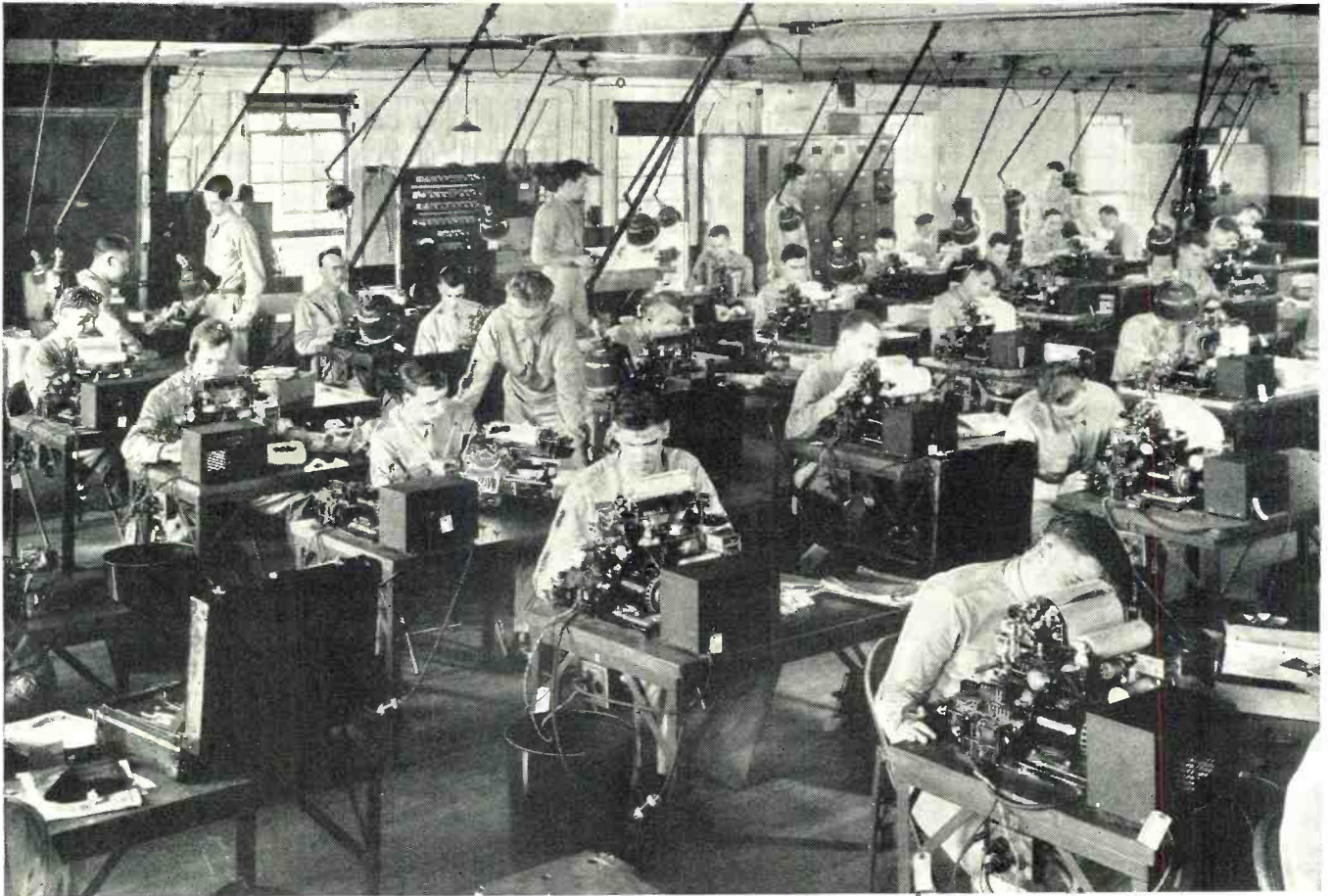
Teletypewriter Maintenance laboratory. Students learn detail assembly and service of mechanical and electrical parts.
