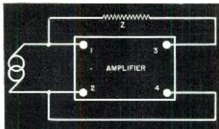
Fig. 2. How negative resistance is obtained.
