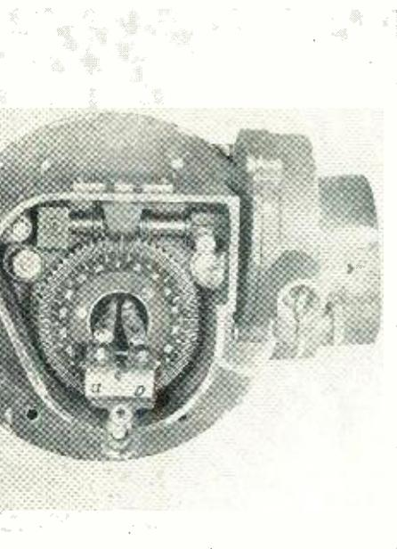
An underside view of a direction-finder loop, a part of the Telefunken direction-finding equipment.
