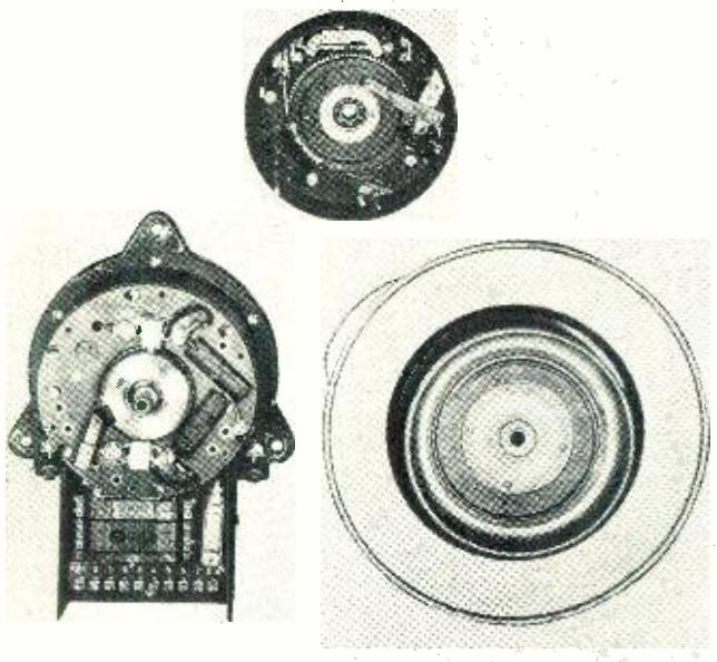
The trailing winch of a dissected antenna system.
