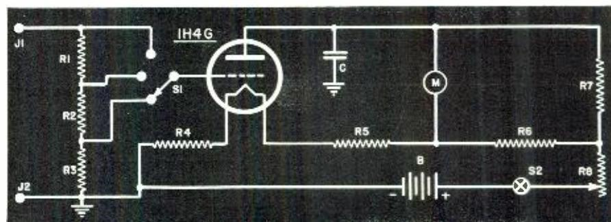
Fig. 4. Another single tube battery-operated meter.
