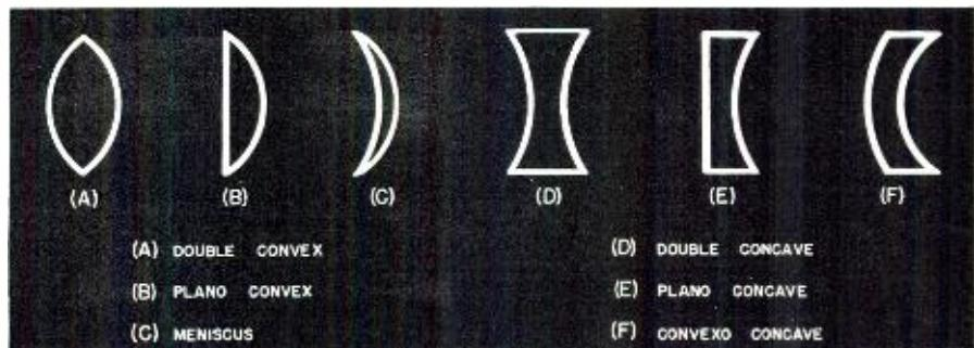
Fig. 2. Illustrated above are six types of lenses.
