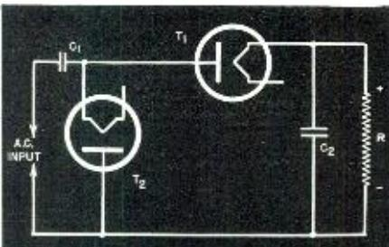
Fig. 1. Half wave voltage-doubler.
