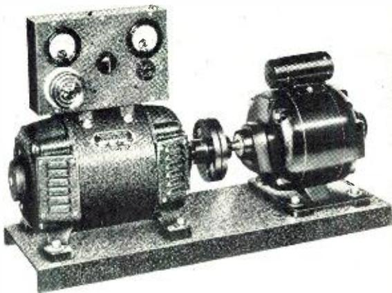
Motor-Generator set with control box.
