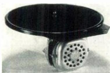
**NEW G. I. PHONO MOTOR** Model CX 78 RPM. Gear driven. 9" turntable. Quiet operation. Powerful synchronous motor, rubber insulated from turntable. Positive direct drive through silent helical cut gears sealed in oil. Depth from mounting plate to bottom 3½". Special now at..... \$6.45 each
