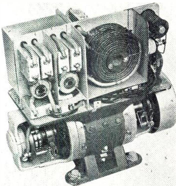
Power Unit and associated filter circuit components for the transmitter and receiver removed from Nazi aircraft.
