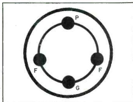
Fig. 2. Socket for dual-purpose tubes.
