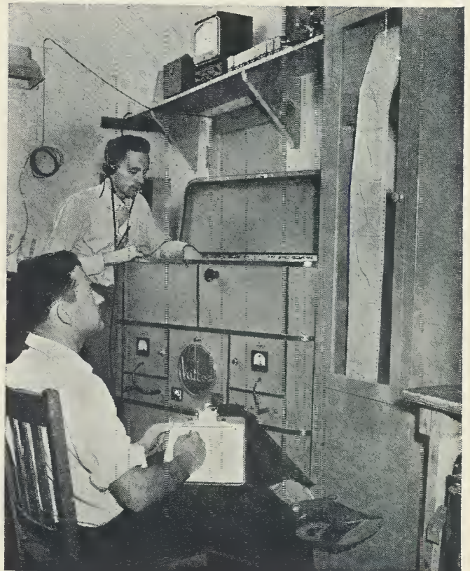
Fig. 3. An endless belt of 72 charts is used in this pen recorder. After decoding is complete, charts are cut apart.
