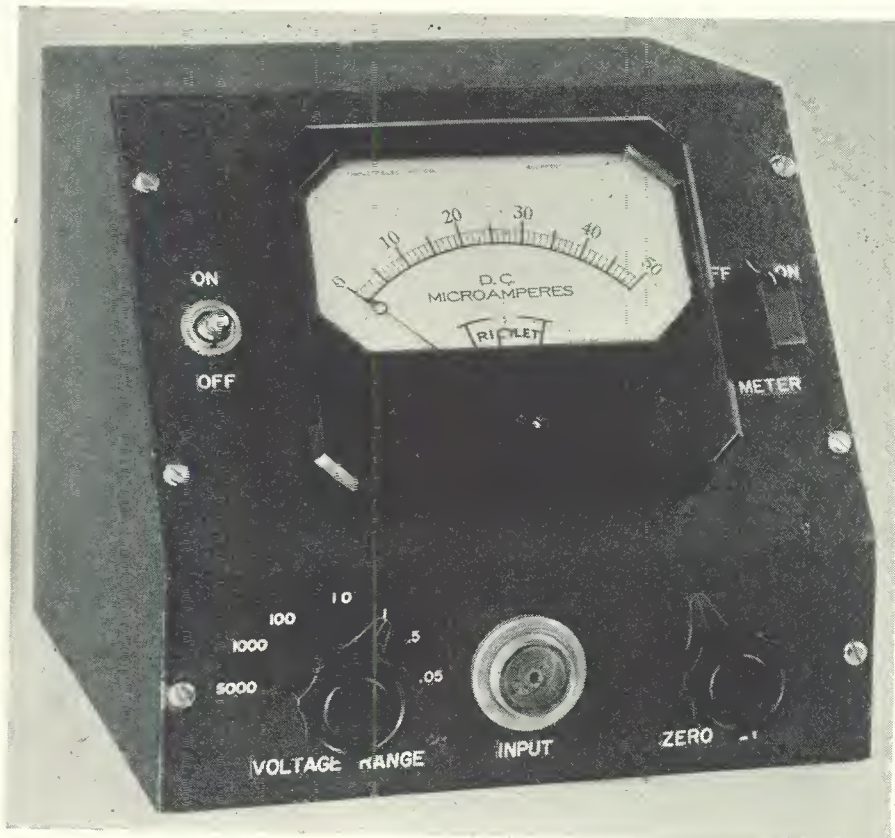
The RADIO NEWS VTVM is an example of a highly-accurate instrument with wide range.
