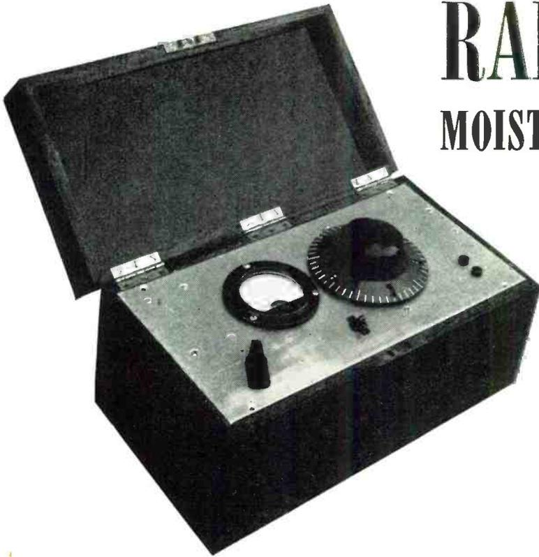
The compact portable soil analyzer. The moisture content of soils must be known to determine reactions of ground waves accurately.
