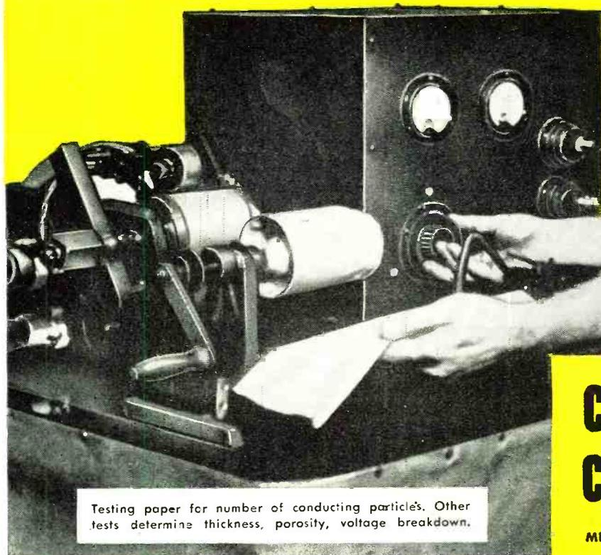
Testing paper for number of conducting particles. Other tests determine thickness, porosity, voltage breakdown.
