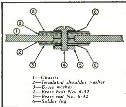
Fig. 2. A novel by-pass condenser. It can be cut into the chassis at any desired position permitting short connections.
