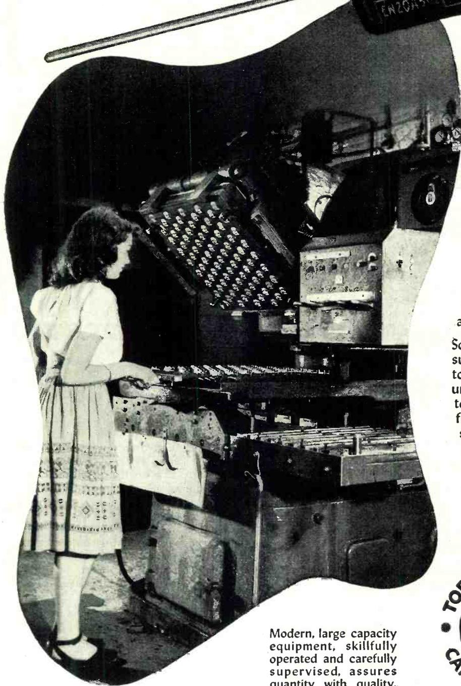
... to deliver molded oil-paper capacitors . . . in quantities more than ample for your needs . . . and in exact agreement with American War Standard C75/221 . . . is afforded by batteries of these dual-77-cavity monsters. Fed with oil-impregnated, aluminum-foil-wound, non-inductive sections and pre-forms of mica-filled phenolic, these huge presses are continually pouring forth capacitors of uniformly high quality with the consistency of characteristics for which Tobe products are famous.
