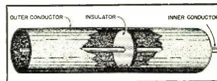
Fig. 4. Typical concentric line.
