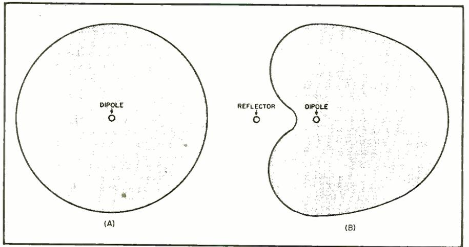
Fig. 10. Radiation pattern of (A) a basic dipole, and (B) a dipole with reflector.
