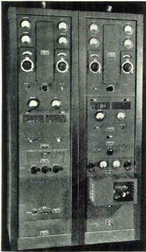
Part of ground station equipment includes, as shown, the side-band generator and audio racks.
