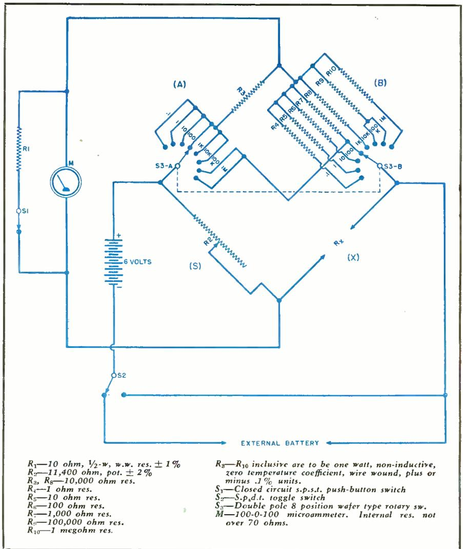
Fig. 3. Diagram of resistance bridge. Meter employed is a 100-0-100 microampere type.
