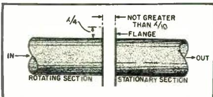
Fig. 7. A wave guide rotating joint.
