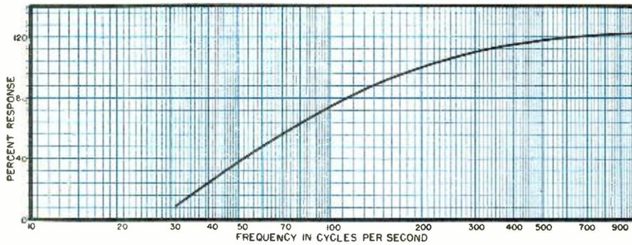
Fig. 2. Frequency response characteristic of the average of a large number of acoustic stethoscopes, minus the effects of the chest piece.
