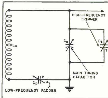
Fig. 1. Basic "padded" oscillator tuning circuit. Low-frequency padding capacitor  $C_p$  is inserted in series with resonant circuit. The oscillator tuning characteristic that will result is shown in Fig. 2.
