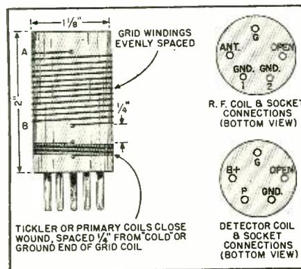
Fig. 2. Coil assembly showing proper position of the various coil windings.
