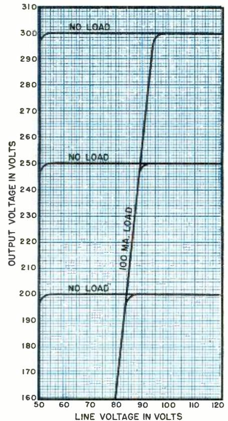
Fig. 1. Curves show variation of output voltage with changes in line voltage.
