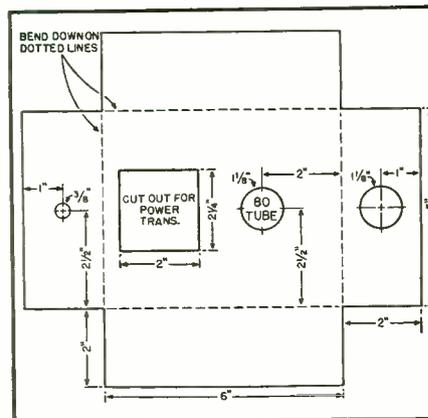
Fig. 3. Power supply chassis layout.
