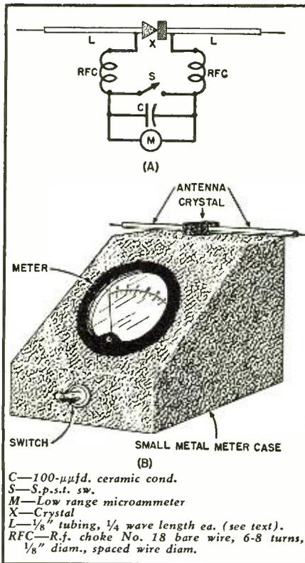
Fig. 4. An efficient field strength meter. This instrument employs a fixed crystal detector as a rectifier connected to a low range microammeter.
