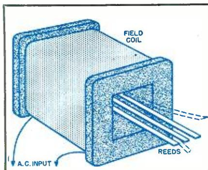
Fig. 1. Mechanical construction of the vibrating-reed frequency meter.
