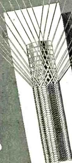
Braided wire covering forms electrical shield over flexible conduit.
