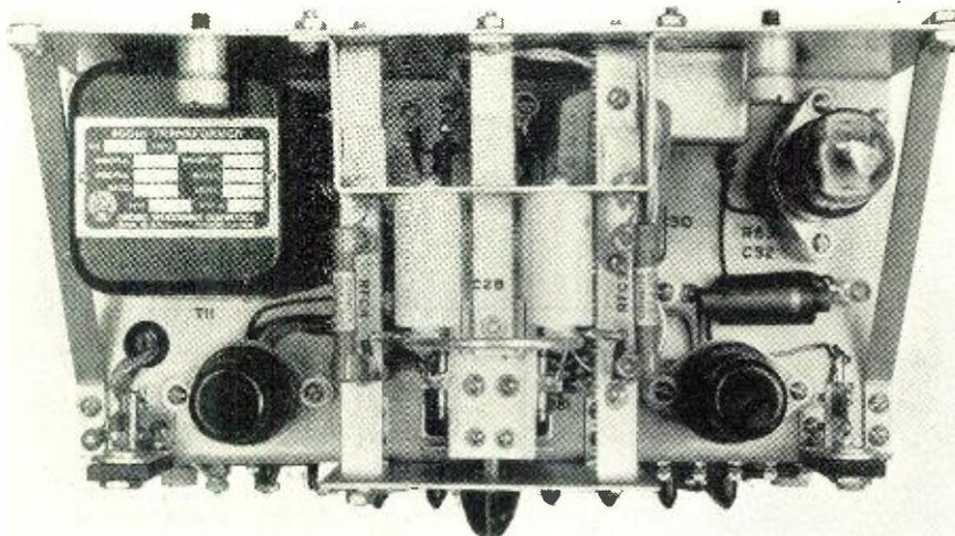
Top view of field detector unit. This instrument has particular application in measuring the radio field strength of airport glide paths.
