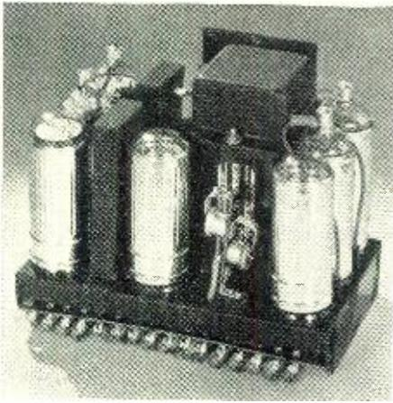
Fig. 8. The Stetho-Cardiette amplifier employing a total of 7 radio tubes; a set of 3 tubes is used for the stethograph section while the other 4 are used for the electrocardiograph. Schematic diagrams for this unit are shown in Figs. 7 and 12.
