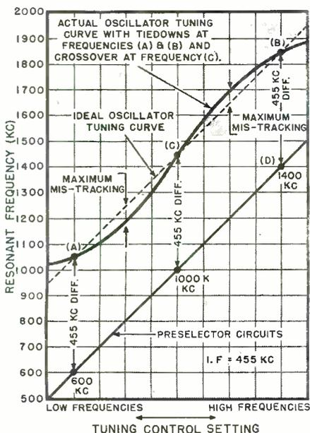
age oscillator tracking is obtained when the three frequencies at which exact tracking occurs are so chosen that the maximum deviations of the tracking curve within the tuning range are small and all the same, as is the case in Fig. 2.
