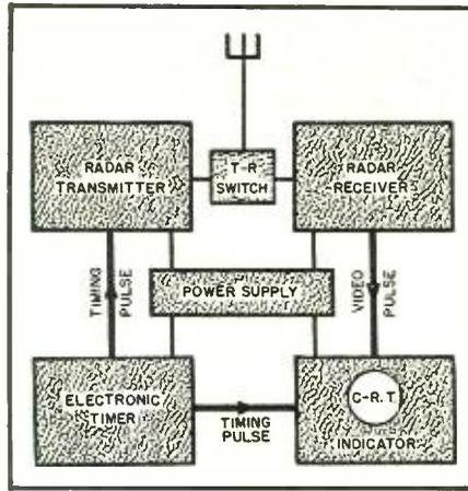
Fig. 13. Single-antenna radar system.
