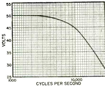
Fig. 2. Frequency response characteristic of a copper-oxide rectifier-type a.c. voltmeter. Its accuracy is undependable over 1000 cycles. It is advisable to employ a v.t.v.m. type meter when making frequency measurements.
