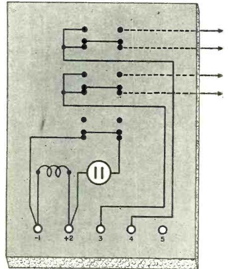
Wiring diagram of time delay relay. Timer must be connected positive and negative as shown, otherwise instrument may be damaged.
