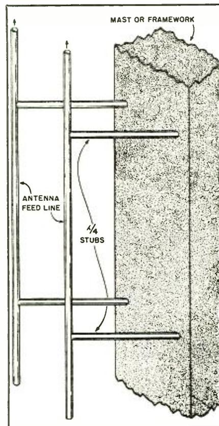
Fig. 3. Use of stub supports.
