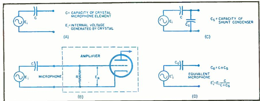
Fig. 6. Step by step analysis of applying a crystal type microphone to pulse wave recording. The standard crystal, as we know it, is not suitable as the time constant RC is too small when used with an amplifier. By adding shunt capacity across this crystal, it can be well adapted to pulse recording equipment.
