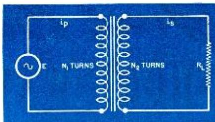
Fig. 1. Iron-core transformer.
