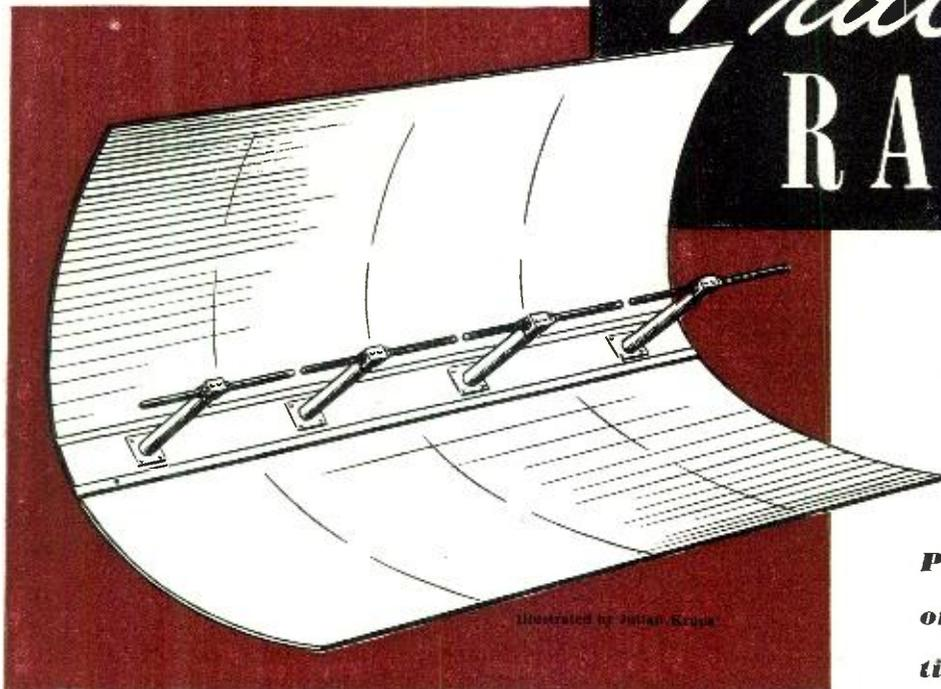
Fig. 1. Antenna used for transmitting u.h.f. pulses.
