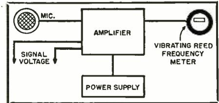
FIG. 5. Basic operation of the amplifier-type reed frequency meter
