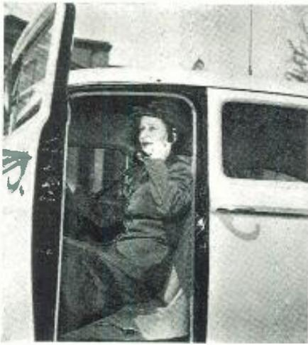
Woman taxi driver for the Yellow Cab Co. is shown using telephone handset in cab for test being conducted by the company in Philadelphia. Mobile two-way radio equipment installed in the test cab and a two-way "land station" on the roof of the 10-story Aldine Trust Building, permits conversations, reports, and instructions between the company's dispatchers and the test cab, whether parked or in operation. The antenna used for mobile operation is shown on roof.
