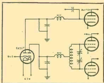
If the grid current greatly exceeds the supply rating, and the grid leak draws a small current, bias isolating rectifiers may be used. The grid leak values will depend on the type of tube in use.
