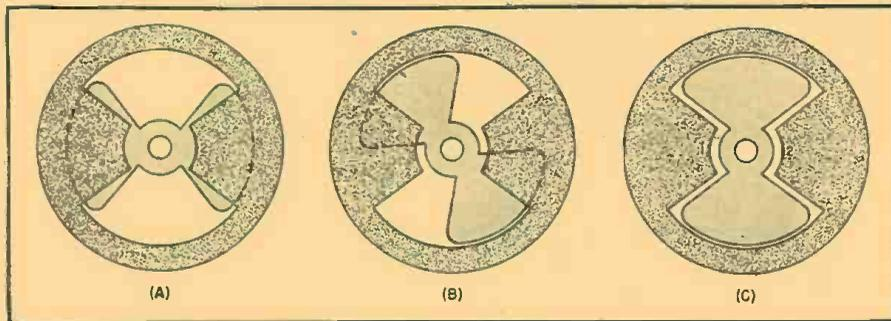
Fig. 7. Butterfly condenser. Refer to text for principle of operation.
