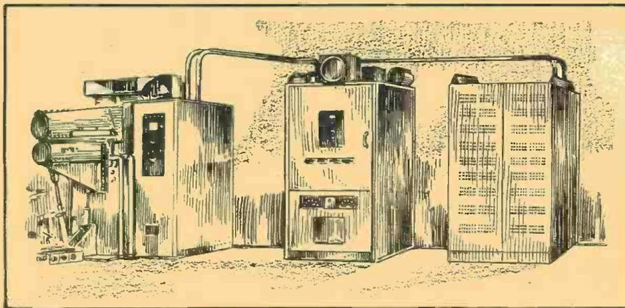
voice currents are already in demand. Using this type of intercommunication system, it is only necessary to plug the intercommunicating units into the power line and select the station of operation.
