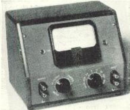
from 7 c.p.s. to 1.6 mc. which makes the unit suitable for voltage measurements in the vibration, audio, super-sonic and broadcast frequency bands.
