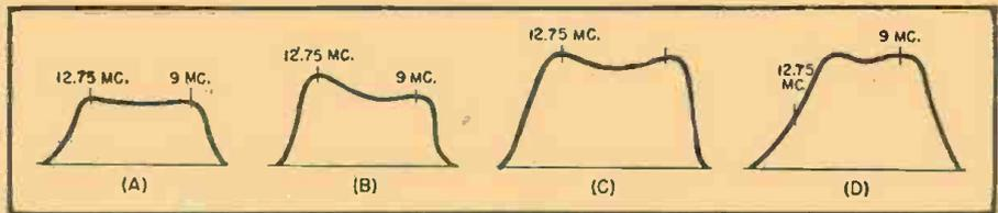
Fig. 4. Curves illustrate i.f. alignment.
