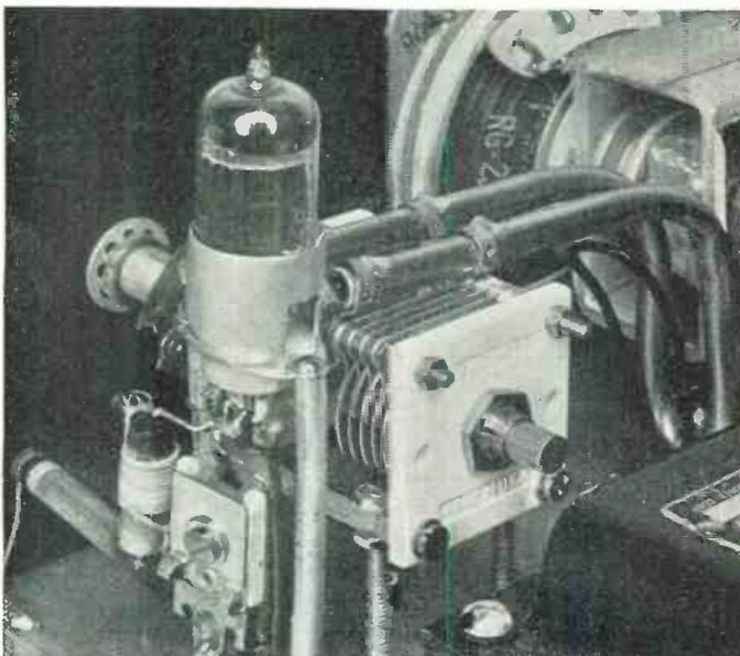
over the fingers, being careful not to bend too sharply, working the curve in gradually. The inductance is fastened to the condenser by means of spade lugs with the open ends of the lugs fastened directly to the stator plates of the condenser, the lugs then bend around to fit snugly on the copper tubing. This forms a low resistance r.f. path for the heavy circulating current.
