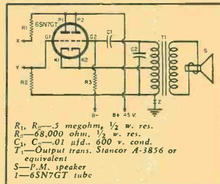
Fig. 1. Circuit diagram for control tube keyed audio oscillator.
