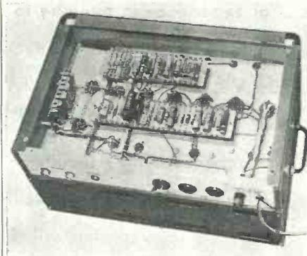
rated at 10, 20, and 30 watts respectively, are in production at the present time. These amplifiers have a virtually flat response from 30 to 15,000 cycles.
