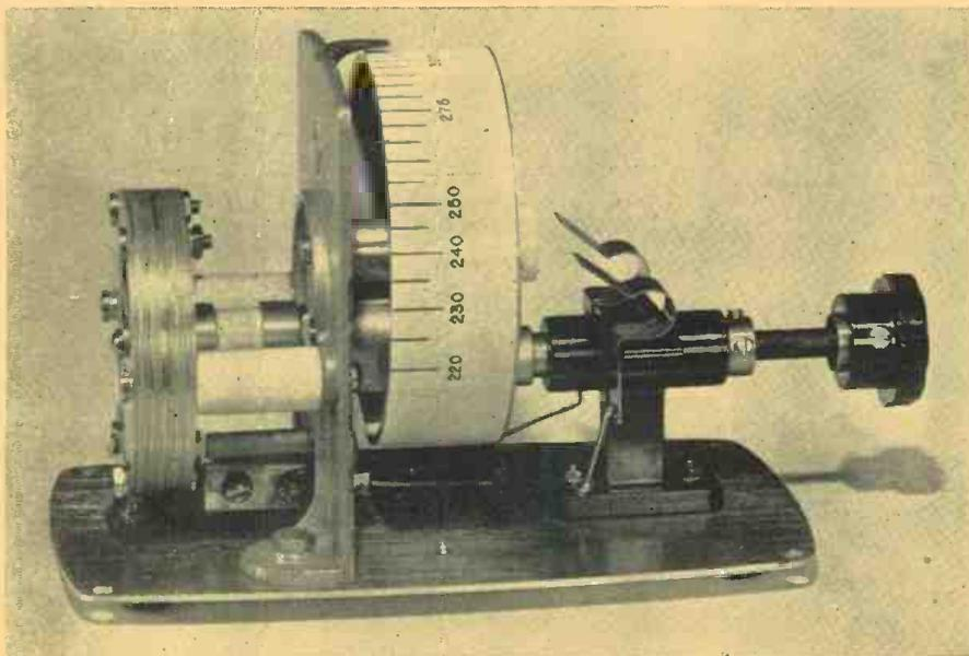
tograph,  $\frac{1}{4}$  inch above the top stator plate, with its center above the center of the rotor. The slider arm is just another piece of No. 12 wire, of the proper length (about  $\frac{3}{4}$  inch) to mount the brass eyelet slider correctly, and is soldered into a groove filed in the shaft of the rotor to give the solder connection a certain amount of mechanical strength. The total inductance of the circuit varies from about .02 to .06 microhenries.
