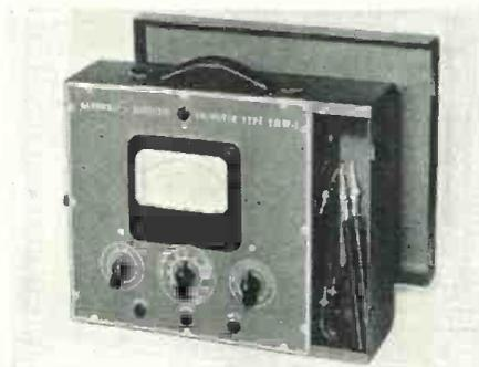
twelve-pound, multi-range measuring instrument will be useful for service and general laboratory work. Accurate measurement of volts, ohms, current and decibels, plus a single rotary selector switch which controls all functions and ranges, are features of this new instrument.
