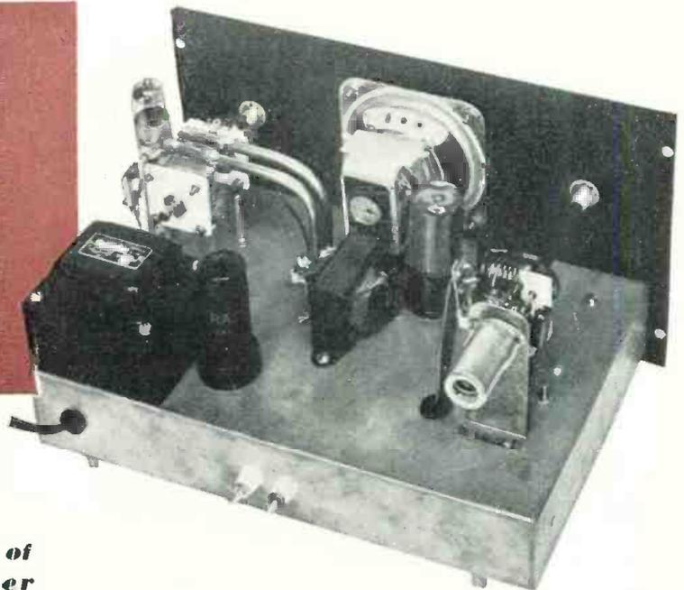
Rear view shows transmitter section (upper left) and receiver (lower right).
