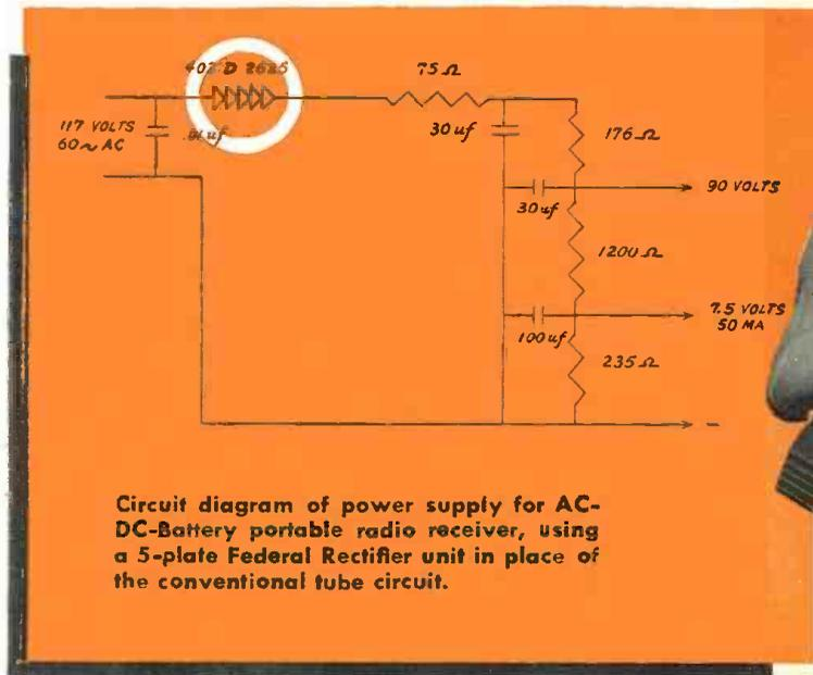
Circuit diagram of power supply for AC-DC-Battery portable radio receiver, using a 5-plate Federal Rectifier unit in place of the conventional tube circuit.
