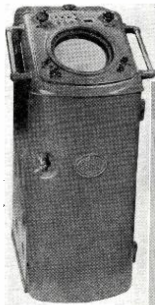
Indicator binnacle of the Sperry Gyroscope set houses 12" PPI and associated controls. Visible are range selector switch, variable range marker, bearing cursor, anti-clutter selector switch, and azimuth scale illumination control.
