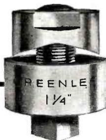
Saves hours of work cutting clean, accurate holes in radio chassis—for connectors and other receptacles. Simply insert cap screw in hole to be enlarged (drill small hole if necessary), turn with ordinary wrench to force punch through the metal. No reaming or filing—hole is smooth and clean. No distortion—die supports metal. Ten sizes from 3/4" to 2 3/4"; also up to 3 1/2" for meters. Write for free catalog 33E to Greenlee Tool Co., 1204 Columbia Ave., Rockford, Ill.
