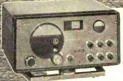
**Model SX-42** Described by hams who have operated it as "the first real postwar receiver." One of the finest CW receivers yet developed. Greatest continuous frequency coverage of any communications receiver—from 540 kc to 110 Mc, in six bands. FM-AM-CW. 15 tubes. Matching speakers available. **\$275.00**
