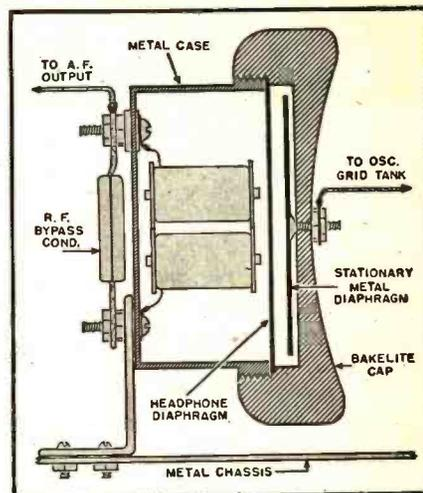
Fig. 4. Mechanical details of an ordinary headphone unit that has been converted for frequency modulation operation.
