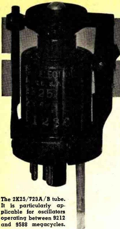
The 2K25/723A/B tube. It is particularly applicable for oscillators operating between 9212 and 9588 megacycles.
