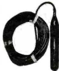
Ideal for detecting underwater sounds, such as fish swimming in schools, within a 15 mile area. Using a Rochelle salt crystal, which is about 1000 times more sensitive than quartz, as the active unit the sound is transmitted up a 60 ft. length of cable. It is completely enclosed in a solid rubber sheath. This sound detector was originally used in harbor defense. Coupled to an audio amplifier, this can be found to have many valuable applications. Ask for SD-1. \$6.95
