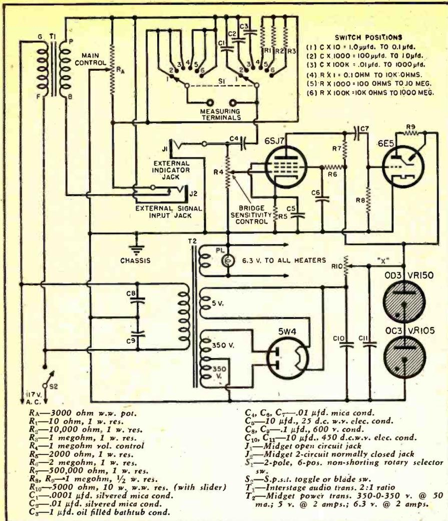
Fig. 2. Schematic diagram of RC bridge. Test instrument covers capacitance ranges from 1 µfd. to 1000 µfd. and resistance ranges from .1 ohm to 1000 megohms.
