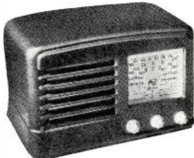
7 tube 3 band (11.8-4.5, 43-1.51 and 184 to 595 meters). Works on 110 or 220 volt AC-DC, 25 to 60 cycles, chassis completely tropicalized, external phono and speaker connections, extra heavy plastic case in various colors
