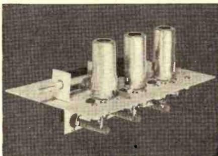
consisting of a 6AK5 r.f. amplifier, 6AG5 mixer and a 6C4 oscillator.
