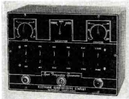
stability, while low leakage is effected through use of double shielding. The set, which operates on a.c., attenuates to less than one microvolt. The panel is of acid etched aluminum with a steel case.
