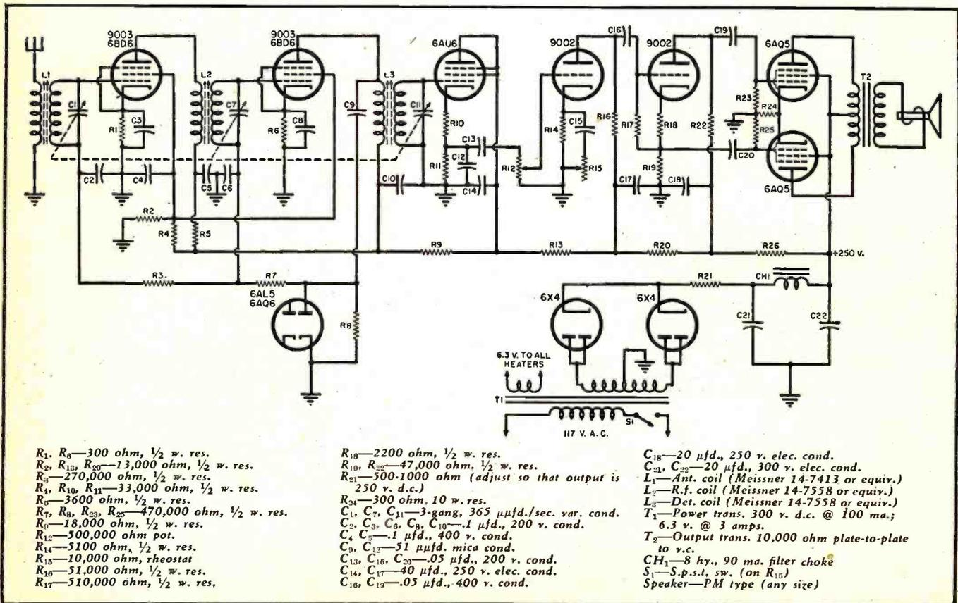
At this plate voltage, two of these tubes will yield 10 watts of power at only five per-cent distortion.
