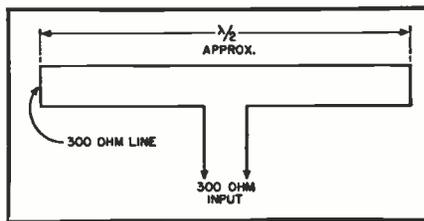
Fig. 1. Electrical representation of the FM and television folded dipole antenna.
