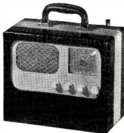
7 tube, battery and AC-DC, 110-220 volt portable, s.w., 10-100 MC and broadcast bands, blue or brown alligator leather case with contrasting leatherette stripe, special antenna furnished for s.w.
