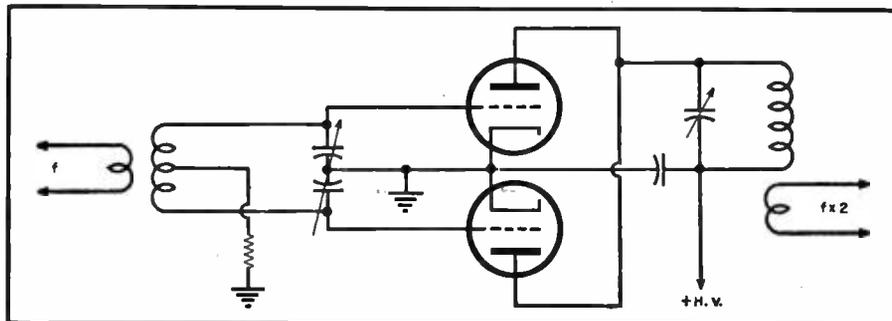
frequencies, the problem of obtaining satisfactory operation of frequency multipliers becomes more difficult, if any appreciable output power is required. If an extremely low output will be sufficient, the low capacity receiving type of tube may be used quite satisfactorily.
