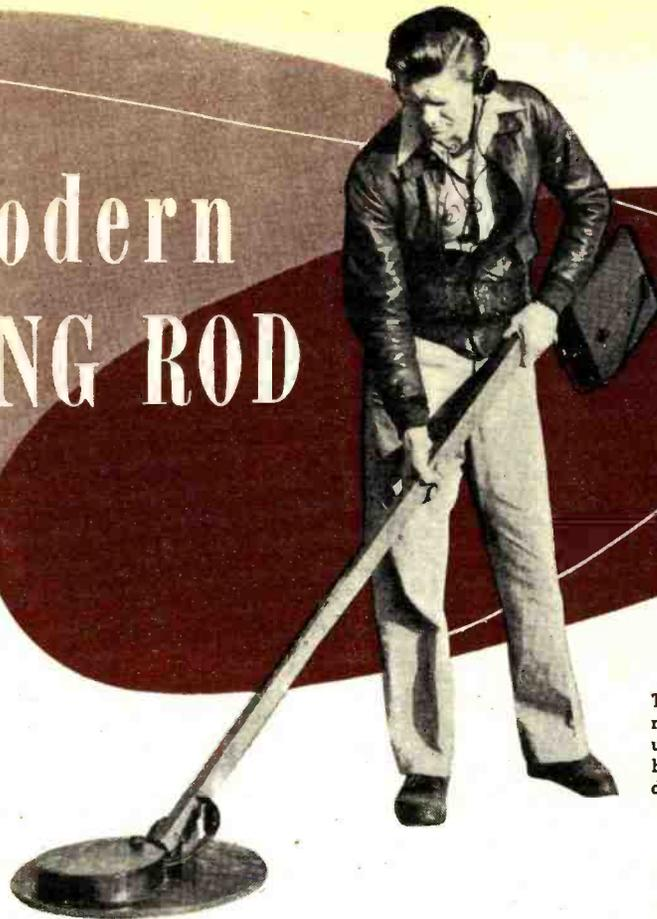
The Goldak Co. Model 520 metal locator. This type unit was used effectively by the British for the detection of land mines.
