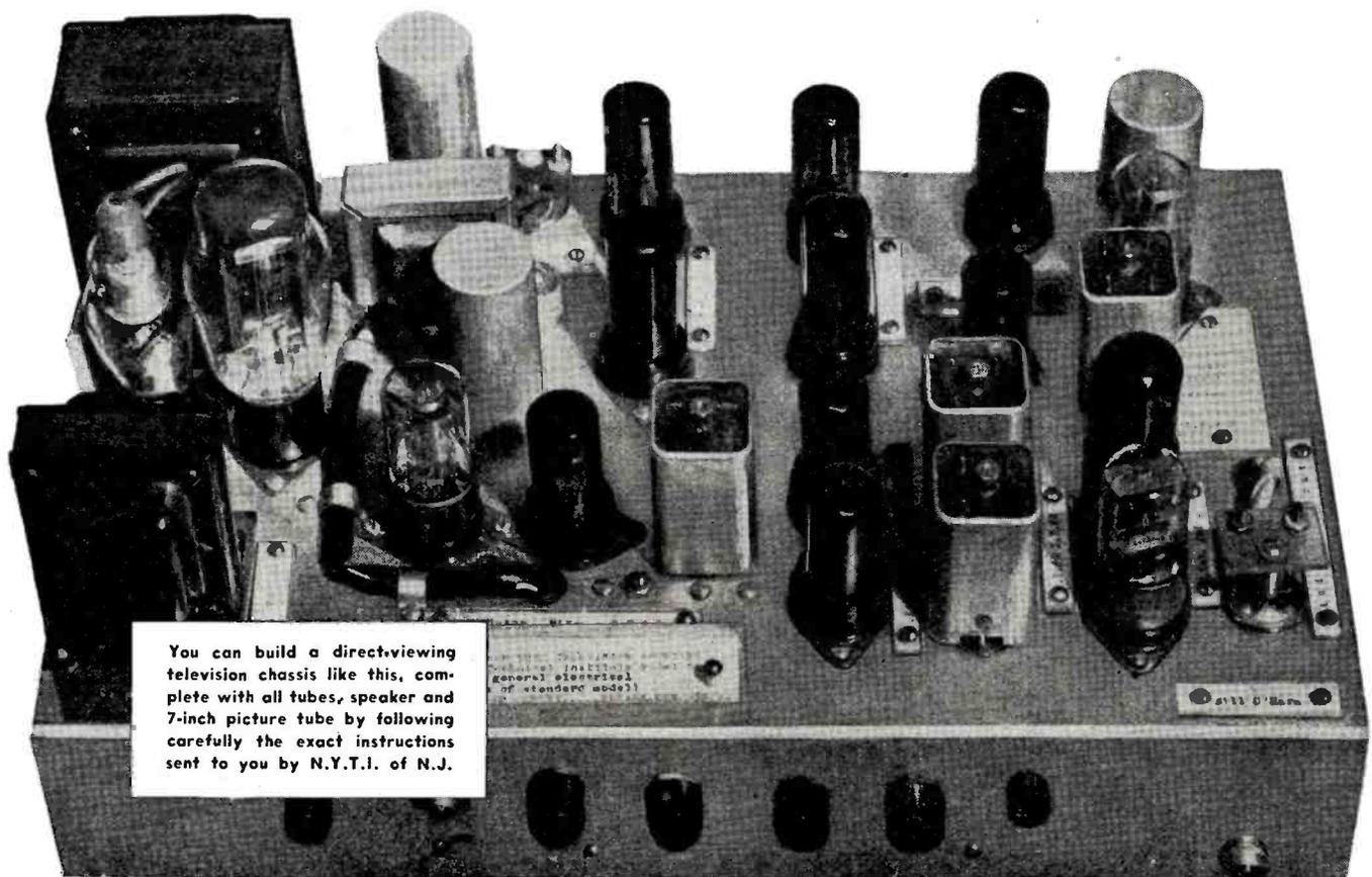
You can build a direct-viewing television chassis like this, complete with all tubes, speaker and 7-inch picture tube by following carefully the exact instructions sent to you by N.Y.T.I. of N.J.
