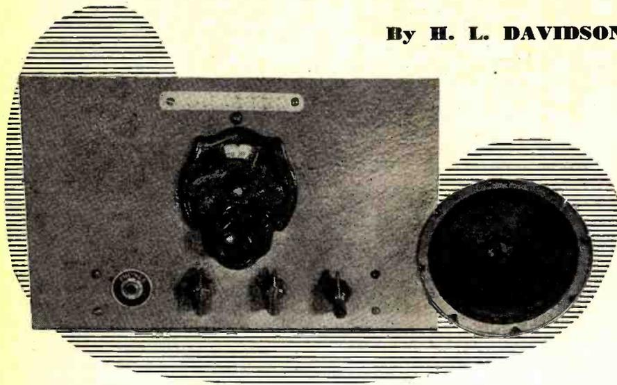
Panel view of home-built 3-tube receiver. Controls from left to right are: phone jack, regeneration control, R<sub>2</sub>, tuning condenser, C<sub>2</sub>, and volume control, R<sub>1</sub>.
