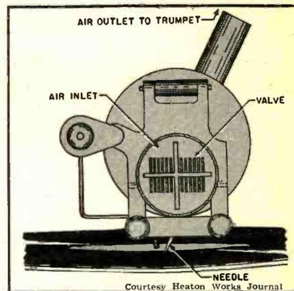
Fig. 4. Construction details of Parson's Auxetophone designed for intensifying sound by means of air pressure.
