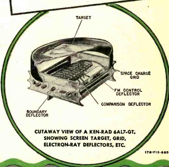
CUTAWAY VIEW OF A KEN-RAD 6AL7-GT, SHOWING SCREEN TARGET, GRID, ELECTRON-RAY DEFLECTORS, ETC.
