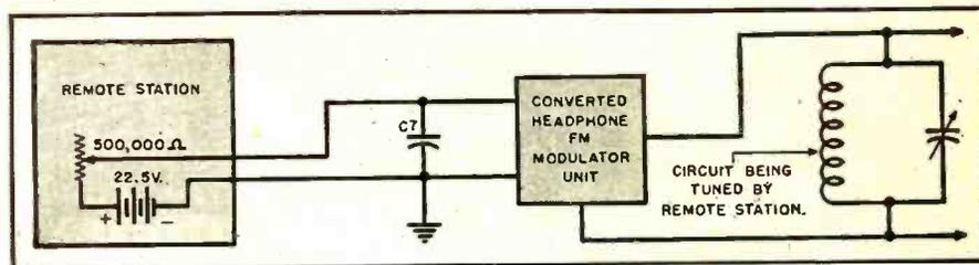
Fig. 3. FM frequency shifting circuit that can be actuated from remote position.
