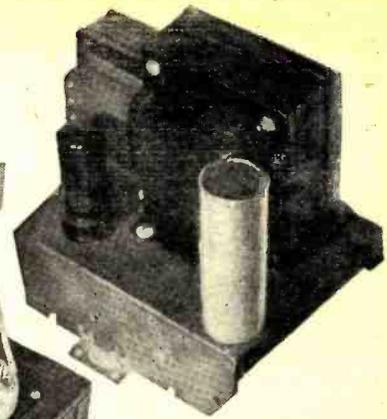
Power supply. A conventional choke input type filter has been incorporated.
