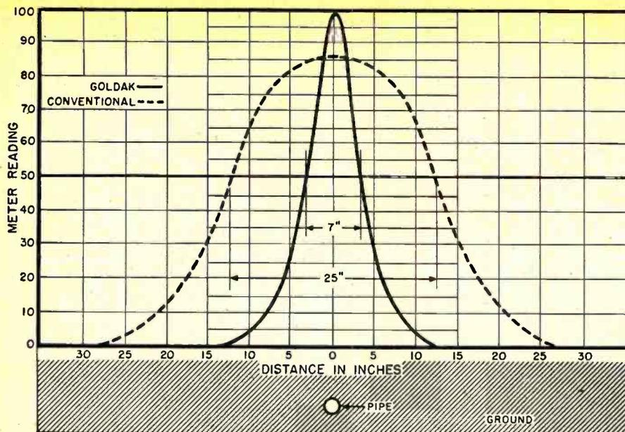
Sensitivity curve shows relative sharpness of positive signal of a modern metal locator as compared to the conventional prewar models.
