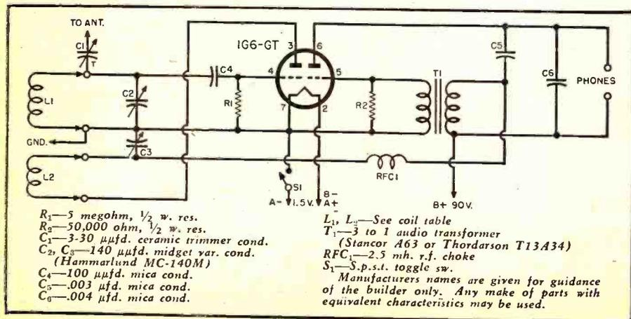
nals. If the desired station is using phone, the regeneration should be adjusted until the receiver is just on the verge of oscillating. It will probably be necessary to retune slightly as the regeneration is adjusted.
