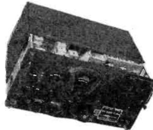
Built for continuous duty, this band switching, six band receiver with a frequency range of 200 to 500 kc. and complete 1.500 kc. to 18,000 kc. Has automatic noise compensator—constant sensitivity on all bands—output at 300 or 4000 ohms—xtal filter AVC-MVC-BFO; Smooth vernier tuning; 90 turns of tuning for each band. Tubes include 1st RF—6K7; 2nd RF—6K7; RF Osc.—6C5; 1st Det.—6J7; 1st IF—6K7; 2nd IF and CW Osc.—6F7; 3rd IF and 2nd Det.—
