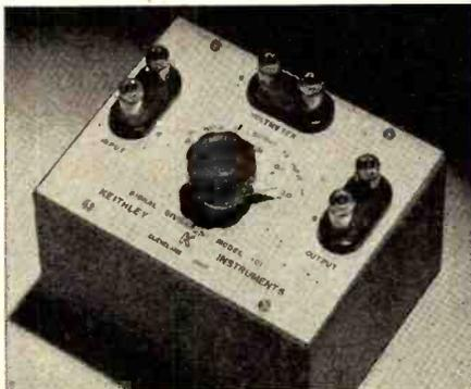
Input and output terminals and a switch knob for setting the ratio are provided on the panel. The voltmeter terminals, connected in parallel with the input, permit the signal to be measured at high level by an insensitive voltmeter, and at the impedance level of the output impedance of the
