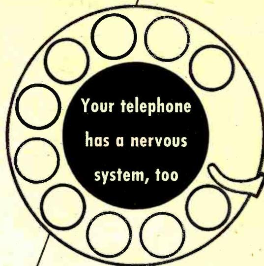
**W**HEN you spin the dial of the latest type of telephone system—known as “common control switching”—you order into action a giant nervous system. It sends electrical impulses through an intricate maze of circuits: more than 10,000 contacts can be opened or closed in a single dial call.
