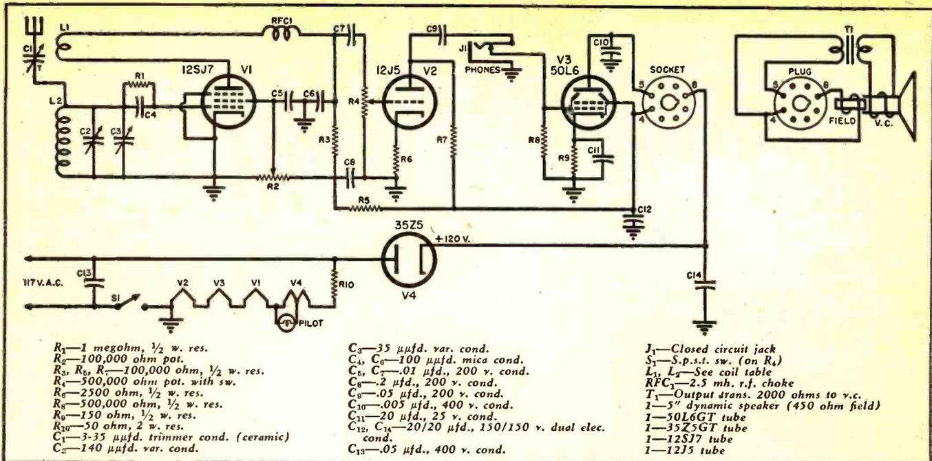
Fig. 1. Schematic diagram of 3-tube receiver. When phone plug is inserted in jack, *J<sub>1</sub>*, speaker is automatically silenced.
