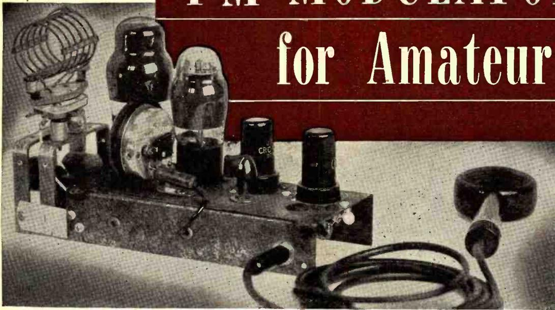
Photograph of home-built FM modulator. A crystal microphone is used for the input. The converted headphone used to produce an FM signal is mounted on the chassis.
