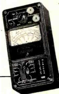
Has A. C. and D. C. Volts at 1000 Ohms per Volt 0-10-50-250-1000-5000 (compensated copper-oxide rectifier provides for A.C. measurements); D.C. Milliampers 0-10-100-500; resistance 0-300-Ohms; 10 Ohms reading at center scale; 0-250,000 Ohms.
