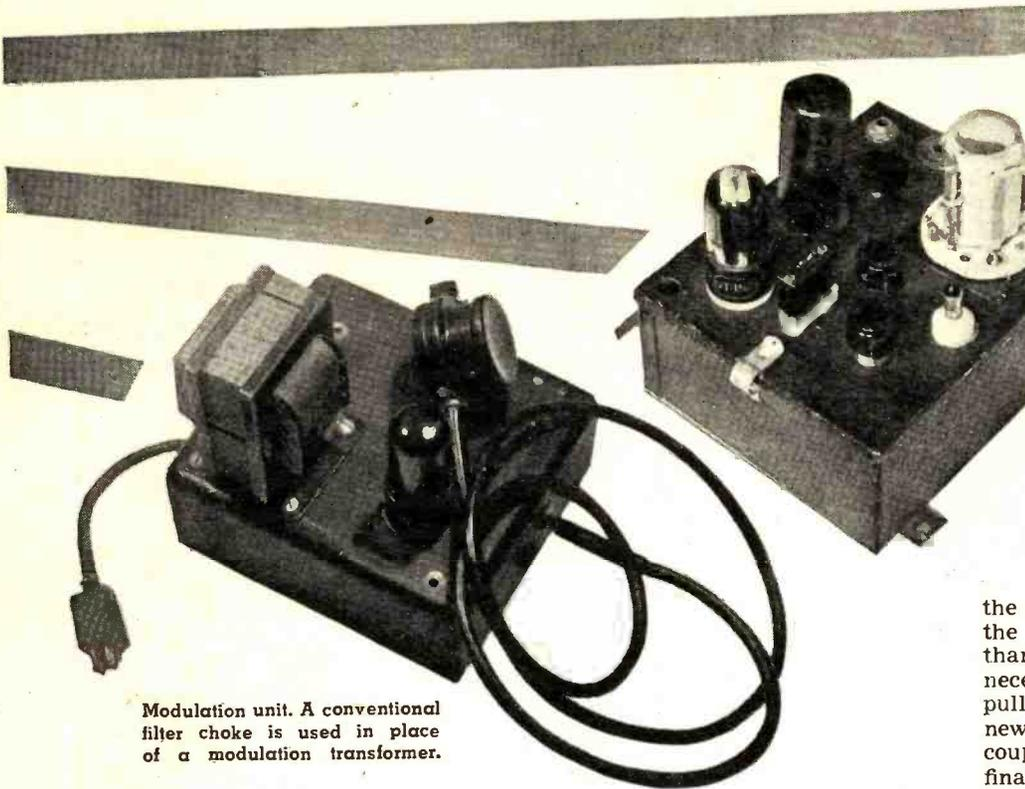
Modulation unit. A conventional filter choke is used in place of a modulation transformer.
