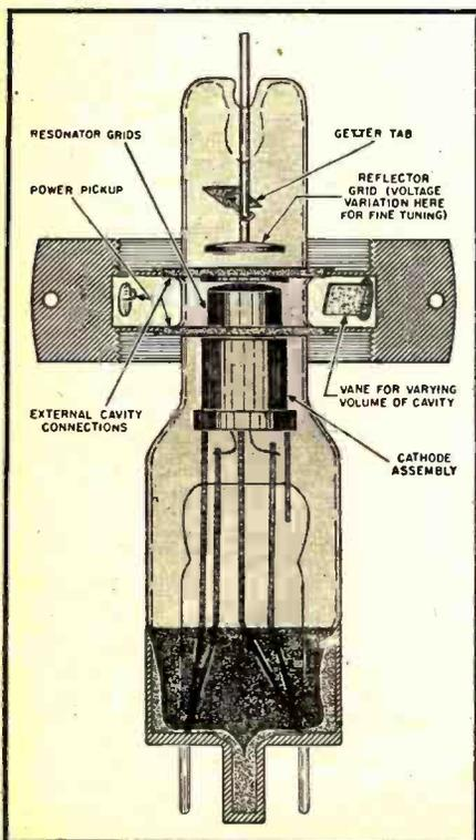
amplifiers. Also, the frequency must be adjustable within a range to accommodate all the frequencies which the receiver is expected to handle. The power of the local oscillator output is also a factor to be considered in design since it is necessary to have the heterodyning carriers of the same power magnitude in order to produce an undistorted i.f.
