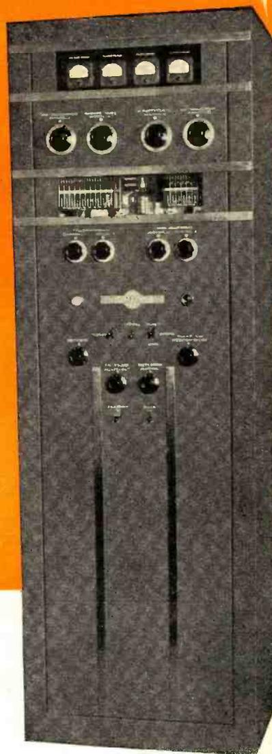
The new Collins 30K-2 embodies certain design features that are of outstanding benefit to owners who employ radio communication from point to point, ground to plane, or shore to ship. This 250 watt radio transmitter can be pretuned to any two frequencies between 2.0 mc and 30.0 mc. Relay operation of all r-f circuits, including antenna tuning, provides instantaneous frequency shift.
