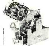
Philco rotary tap tone control. 3 position, including condensers. Only 1 wire to connect to grid of audio tube. ¼" shaft. 25c
