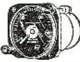
APN-1—ALTIMETER INDICATOR—Basic movement 0-1 ma. 5 ma shunt, 270° scale. An excellent basic G. E. movement for constructing your own meters. N-1. \$1.95
